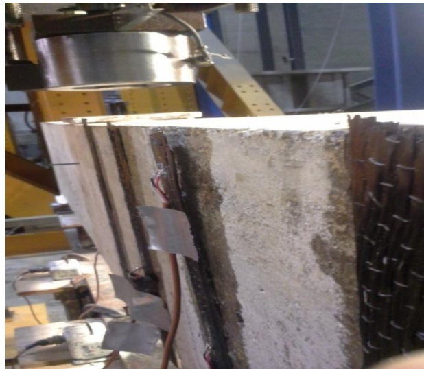
Figure 4-4: Middle FRP U-wrap of beam U-30-NA-2L after debonding
