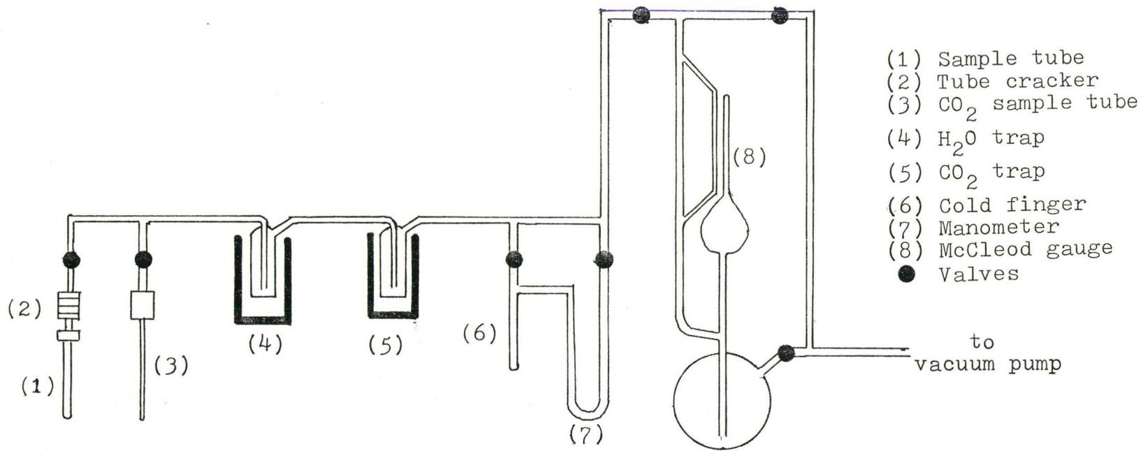
FIG. 6. Apparatus used to make volume measurements. The manometer was used to measure CO<sub>2</sub> volumes and the McCleod gauge was used for CH<sub>4</sub> volumes.
