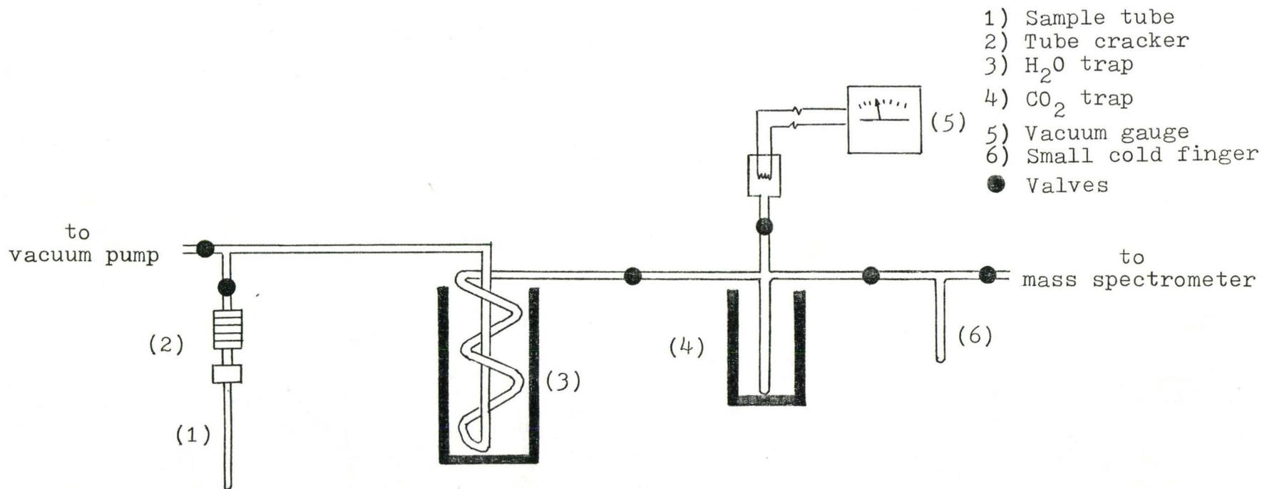
FIG. 5. Apparatus used to isolate CO<sub>2</sub> for mass spectrometer analysis. Small CO<sub>2</sub> samples are retained in the smaller cold finger.
