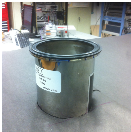
Figure D.8: The base of the cryostat, with the interior (see Fig. D.7) removed for sample mounting.
