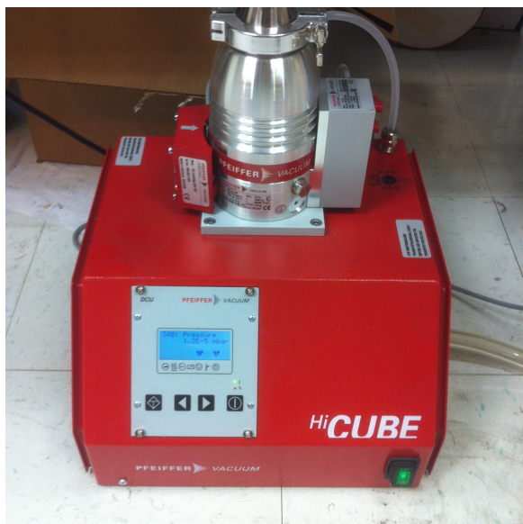
Figure D.5: Pumping station (turbo pump, with diaphragm backing pump).
