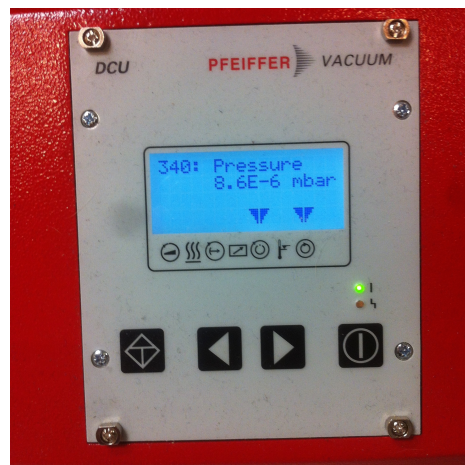
Figure D.6: Stabilized 300K pressure reading (from Pirani gauge in Fig. D.4) of pump connected to cryostat (as shown in Fig. 4.1).
