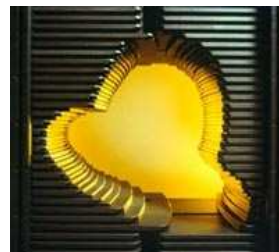
Figure 1.2: A multileaf collimator shapes the radiation beam to conform to the target in the patient's body [2].
