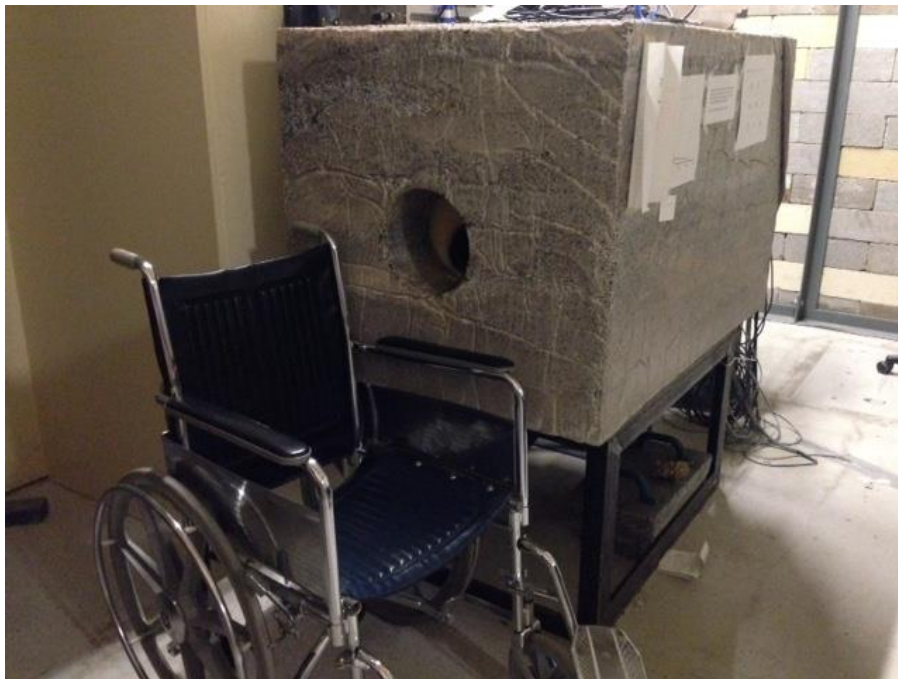
Figure 2.2. The shielded 4\pi detector assembly at McMaster University.
