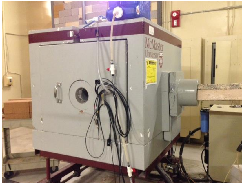
Figure 2.1. Irradiation cavity of the Tandetron accelerator at McMaster University.
