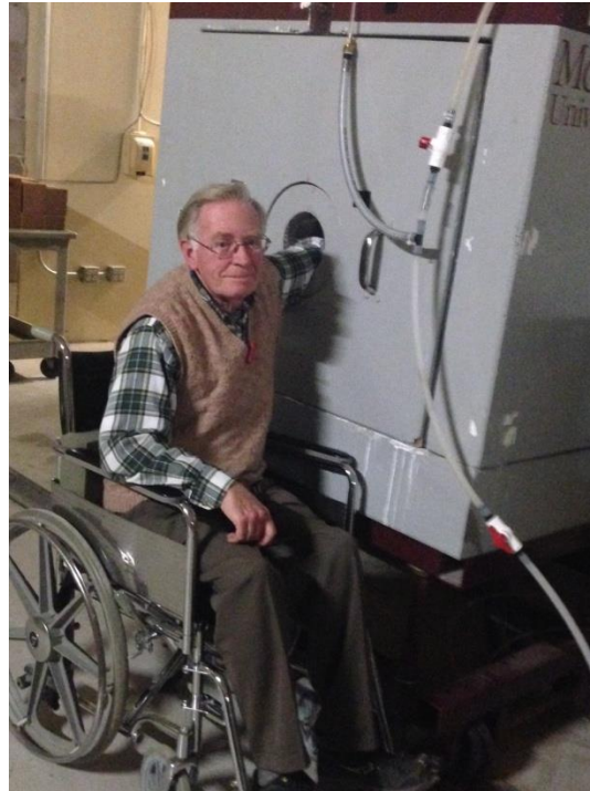
Figure 1.2. Irradiation cavity of the Tandatron accelerator at McMaster University showing a subject positioned for irradiation.
