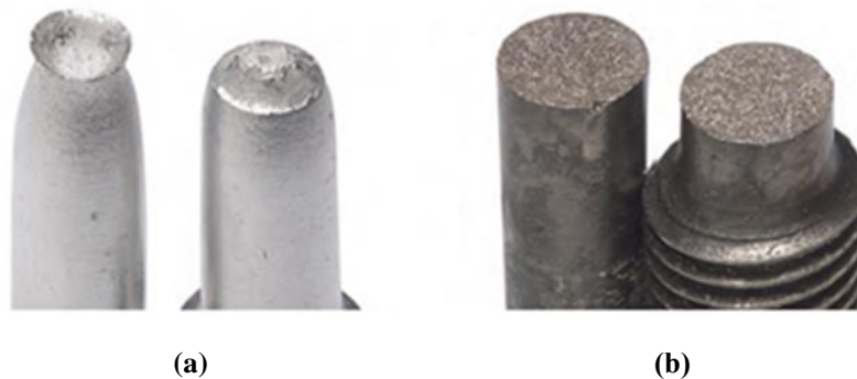
Figure 2.5: (a) Cup-and-cone fracture in aluminum. (b) Brittle fracture in a mild steel.
