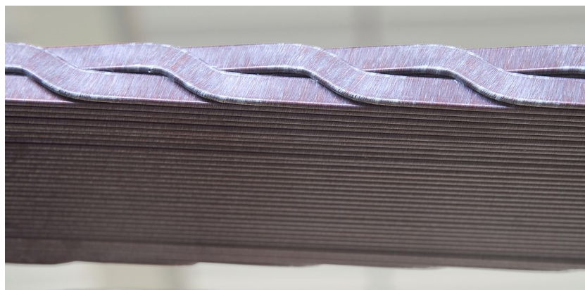
Fig. 6.4. A typical Roebel bar winding (Photo courtesy Partzsch Group) [136].
