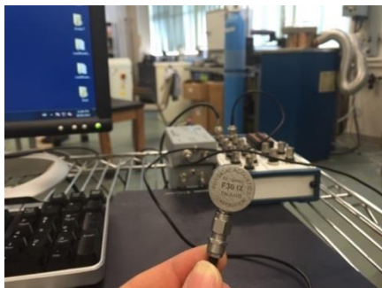
Fig.3.3. F-30 \alpha AE sensors which have high sensitivity and flat response at band width of 150-700 kHz
