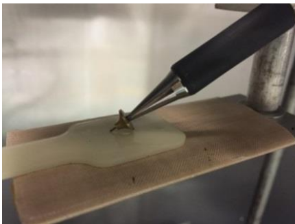
Fig.3.6. Nielsen shoe used for pencil lead break test
