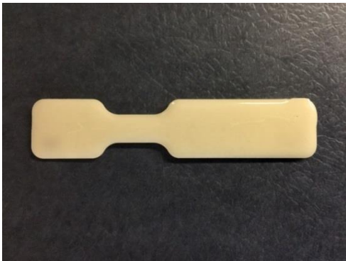
Fig.3.2. Modified dog bone specimens used in all trials, flexural and tensile for this project.
