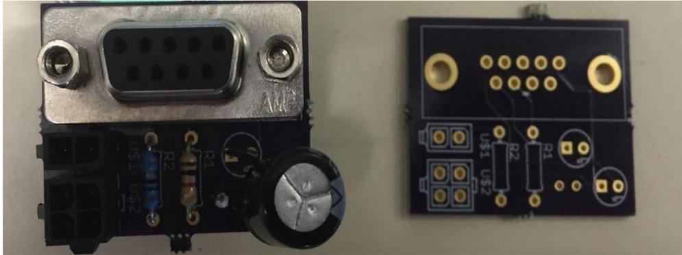
Figure 3.6: Current Sensor PCB
