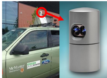
Figure 4.11 The car equipped with Velodyne HDL32 LiDAR
