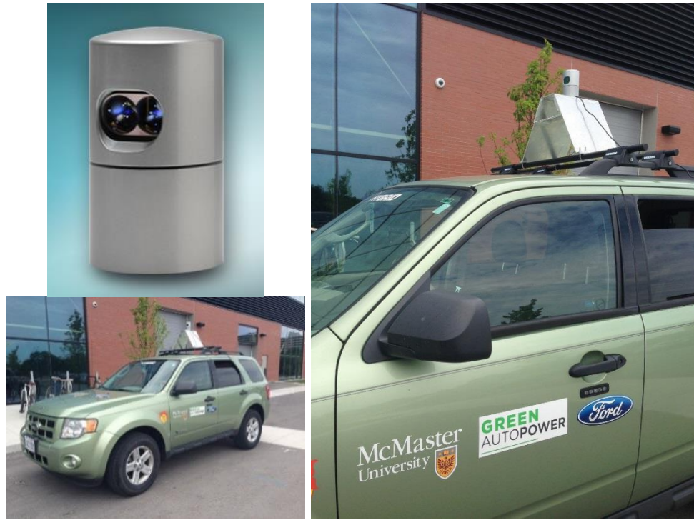
Figure 1.7 LiDAR sensor and experimental set-up
