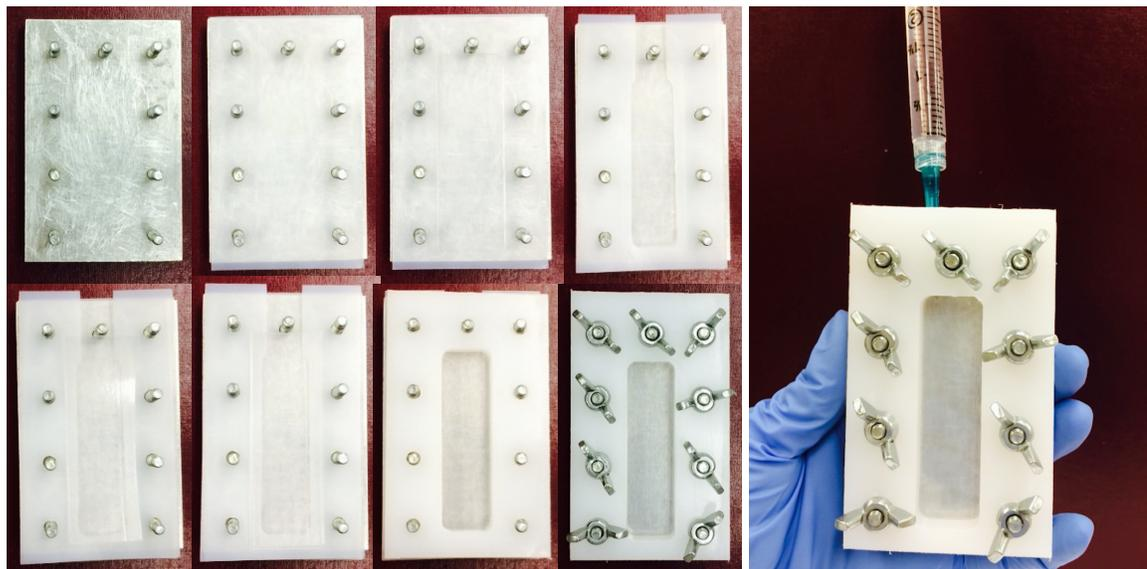
**Figure 3.2.3** Assembly of casting mold and injection of macromer mixture into mold.
