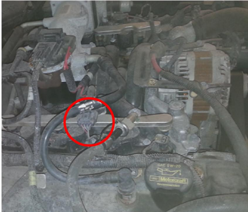
**Figure 5.2.2** Example of a spark plug connector.
