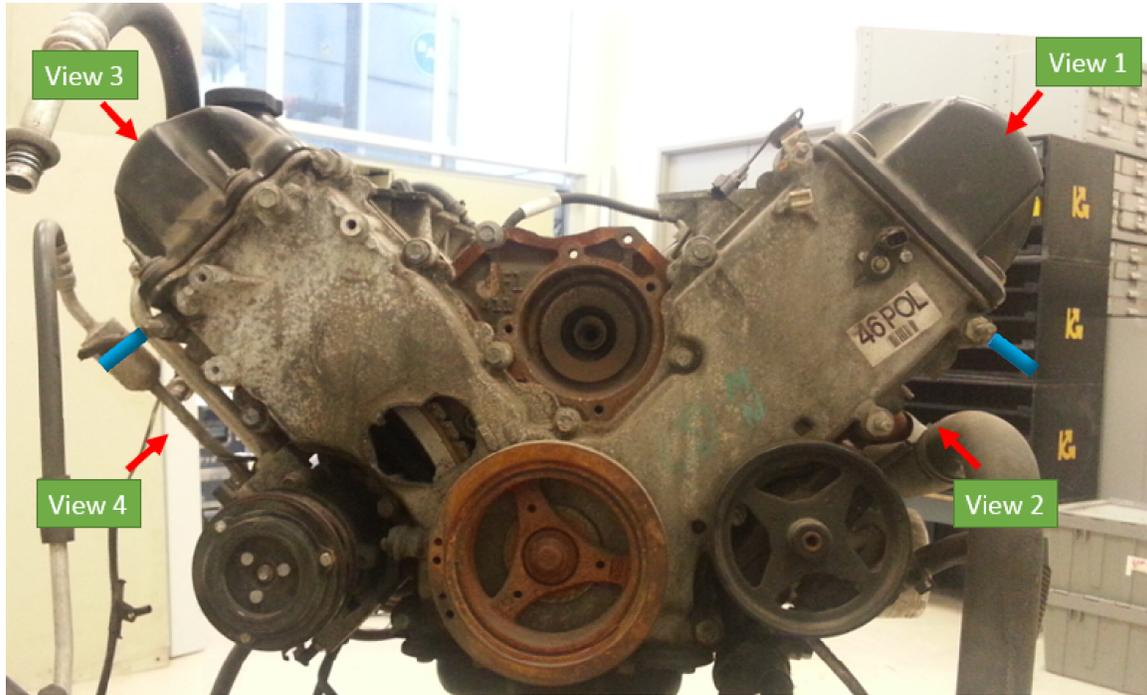
(a) Positions and orientations of the accelerometers shown in the front view of the ICE. (The blue shapes stand for the sensors. Same with View 1 & 3.)
