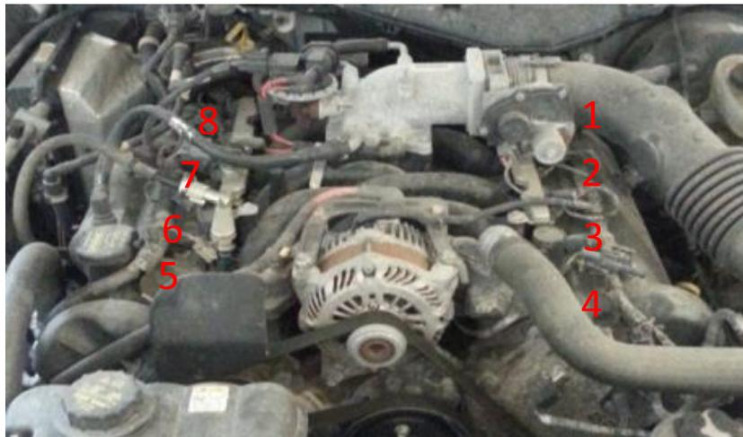
**Figure 5.2.1** Spark plug numbering.
