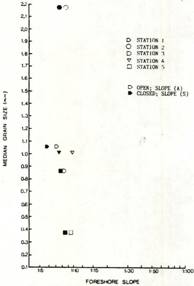
Figure 2.0: The foreshore slope plotted against the median grain size.
