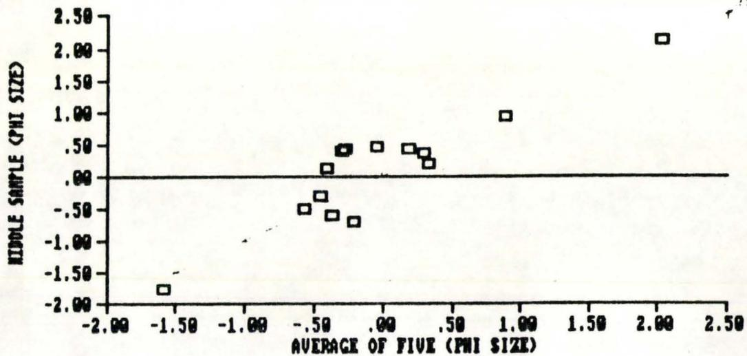
Figure B3.0: The average of the five sediment samples from the first sampling day plotted against the middle sample (C) from the last sampling day. This graph illustrates that the middle sample is not representative of the sediment at that time.
