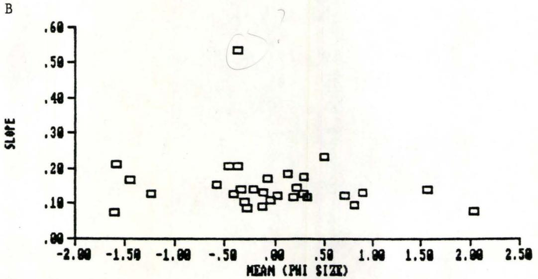
Figure 3.0: The relationship between the mean grain size and the slope for: A) Slope (A); and B) Slope (S).
