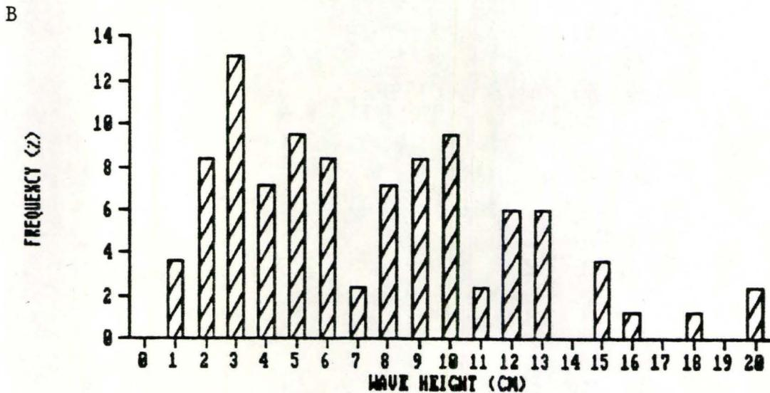
Figure B5.0: The frequency of wave height occurrence at the study site, where: A) is the total number of waves for the entire study period; and B) is a graph of the waves which appear to affect the area the most.
