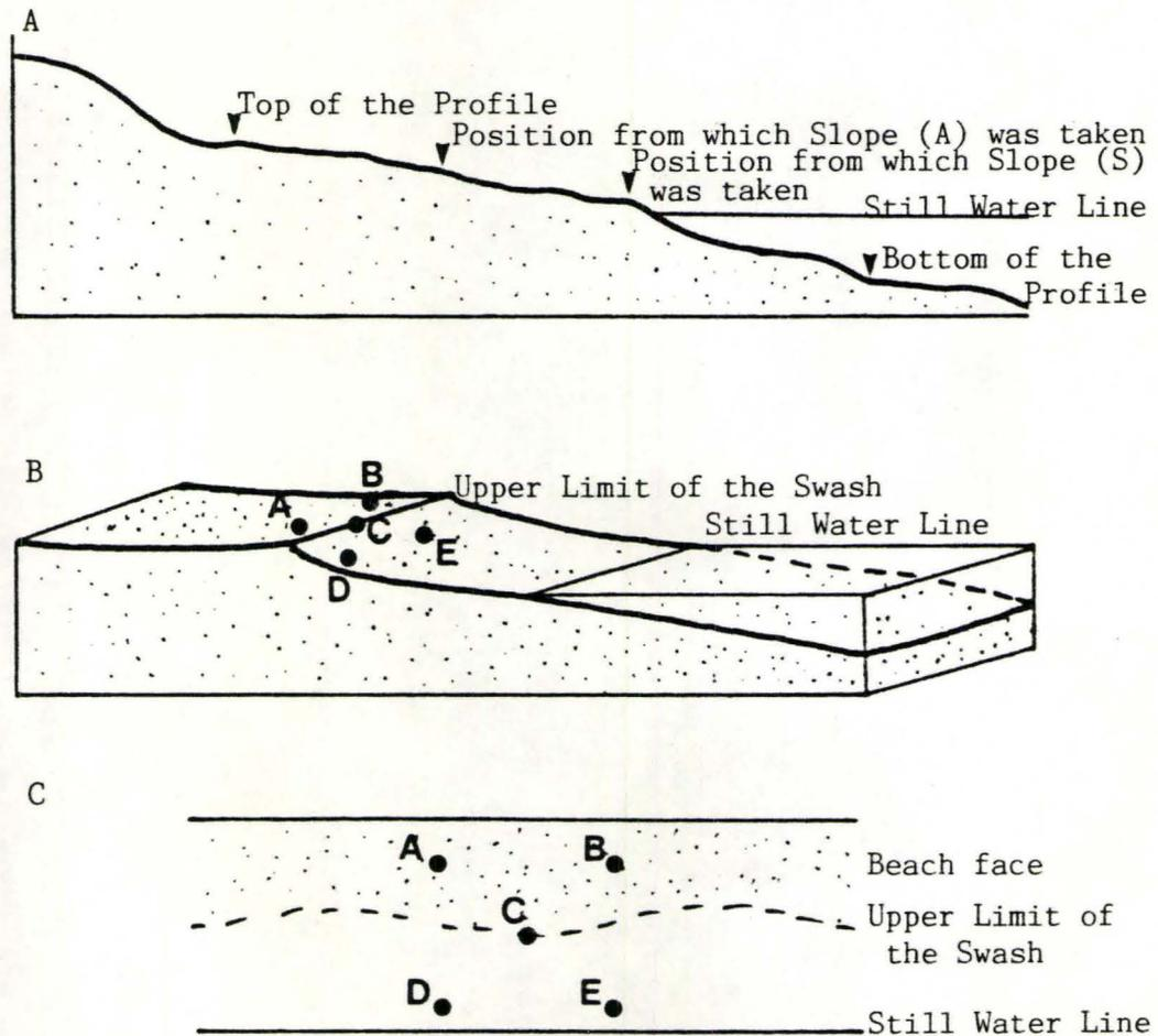
Figure B1.0: These figures demonstrate the method of sampling where: A) illustrates the maximum and minimum limits of the profiles, and from where the two slopes were calculated; B) shows a three-dimensional view of the location of the sediment samples collected in the field; and, C) shows the plan view of the position of the sediment samples on the beach.
