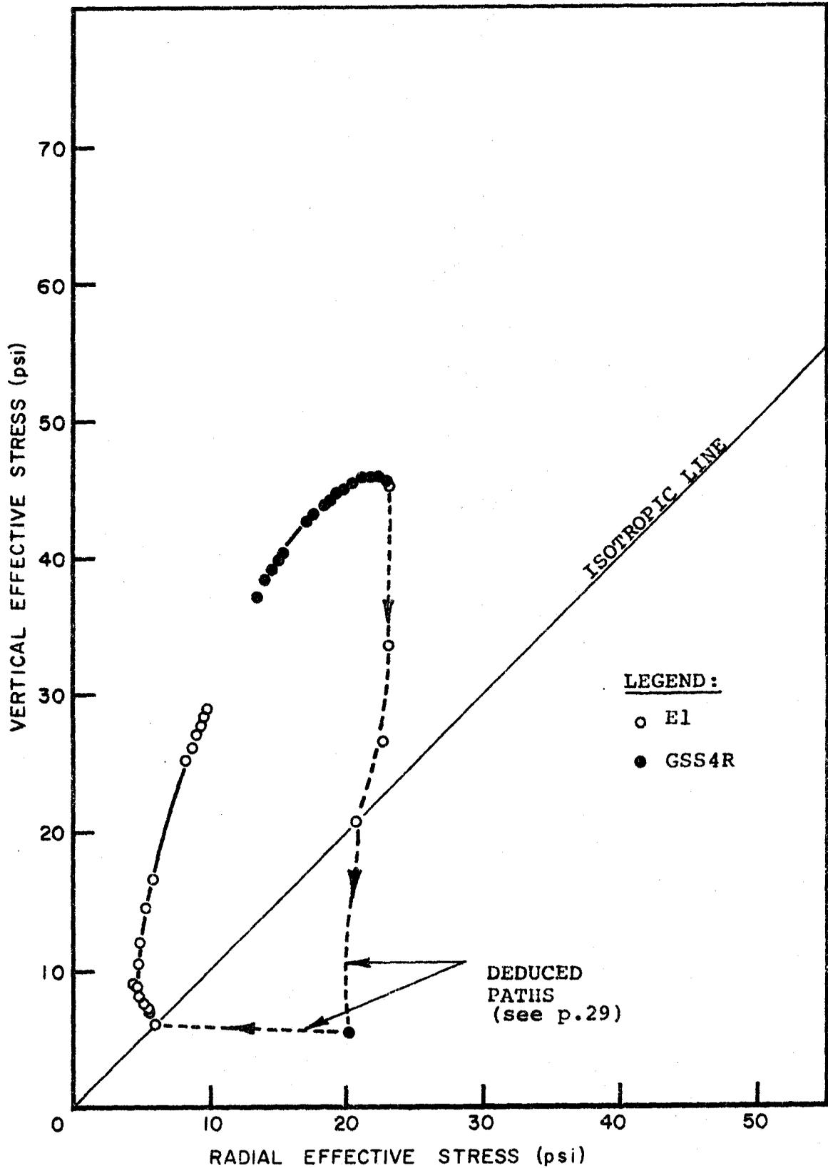
FIG. II. EFFECTIVE STRESS PATH OF "EXTENSION" and "GROUND" SAMPLES.
