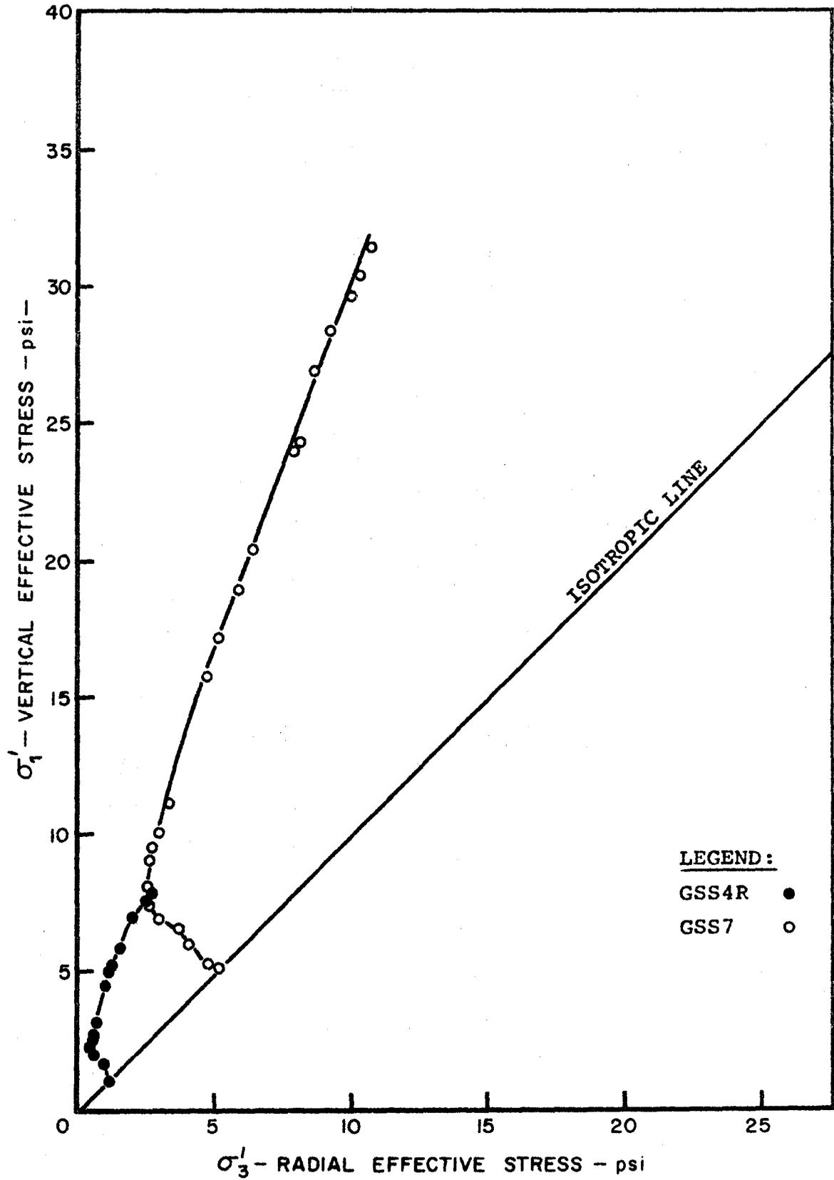
FIG. 13. EFFECTIVE STRESS PATH OF REMOLDED SAMPLES.
