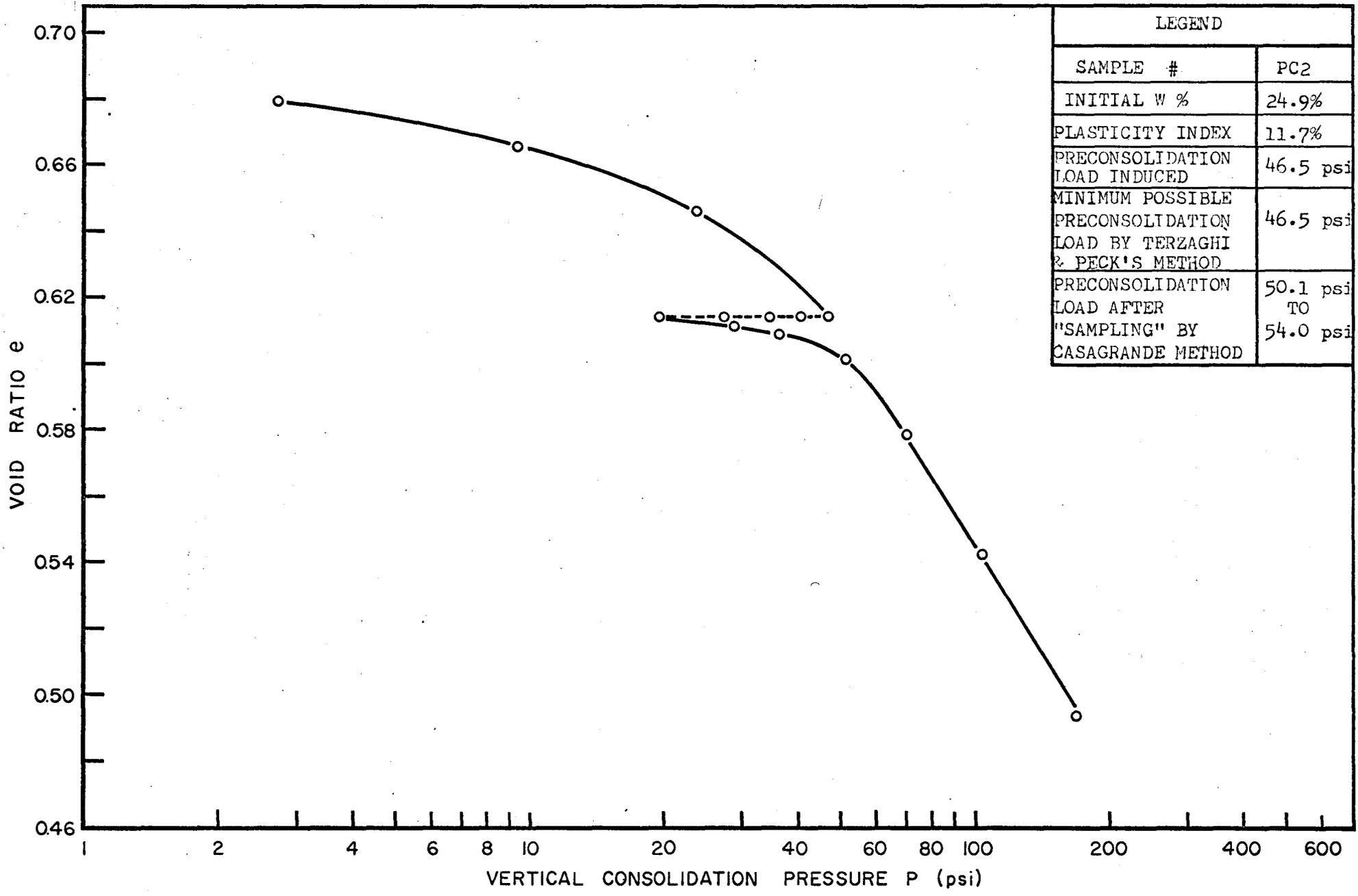
FIG. 18. EFFECT OF "PERFECT" SAMPLING CYCLE — TRIAXIAL  $K_0$  CONSOLIDATION —
