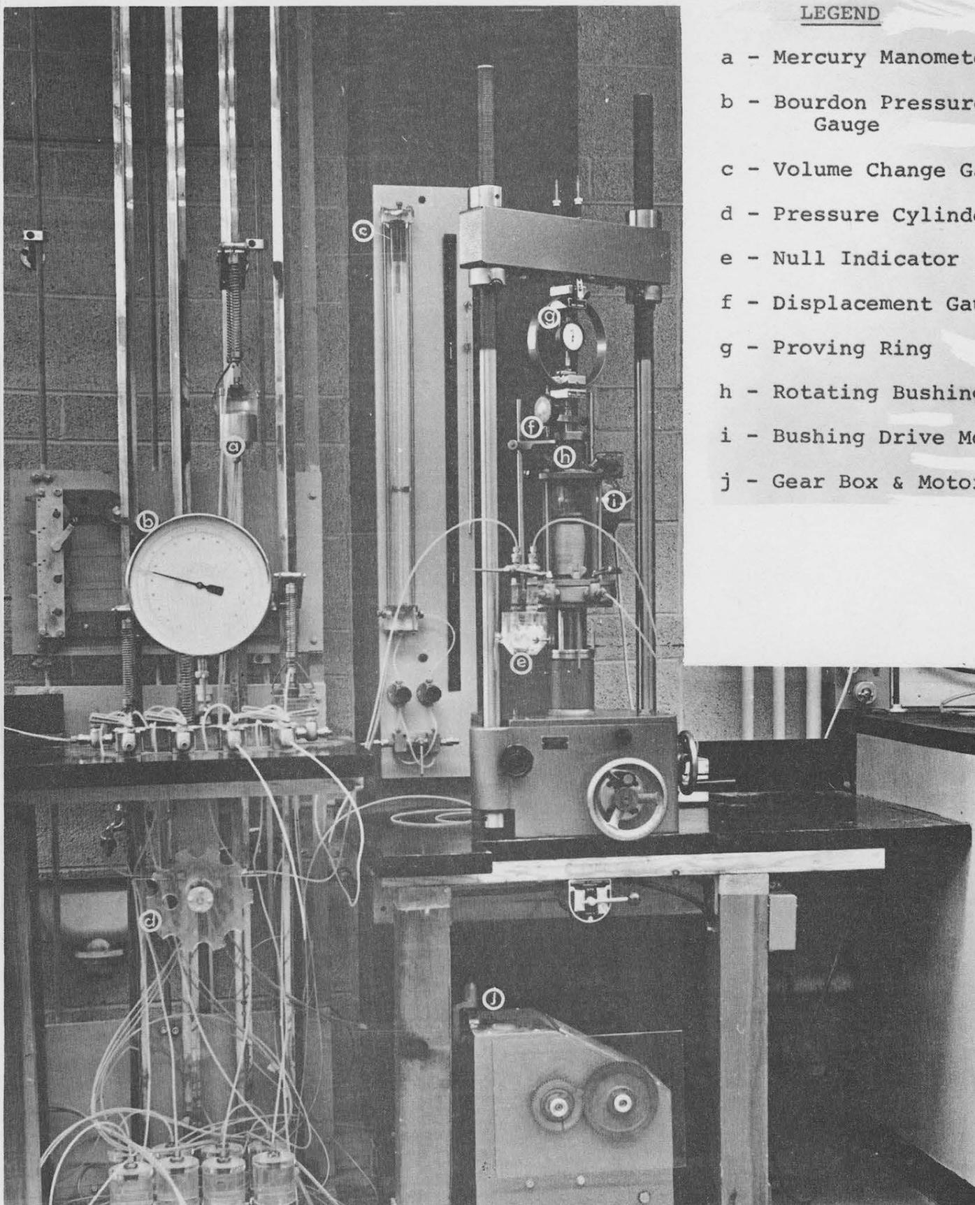
FIGURE 3 TRIAXIAL TEST APPARATUS
