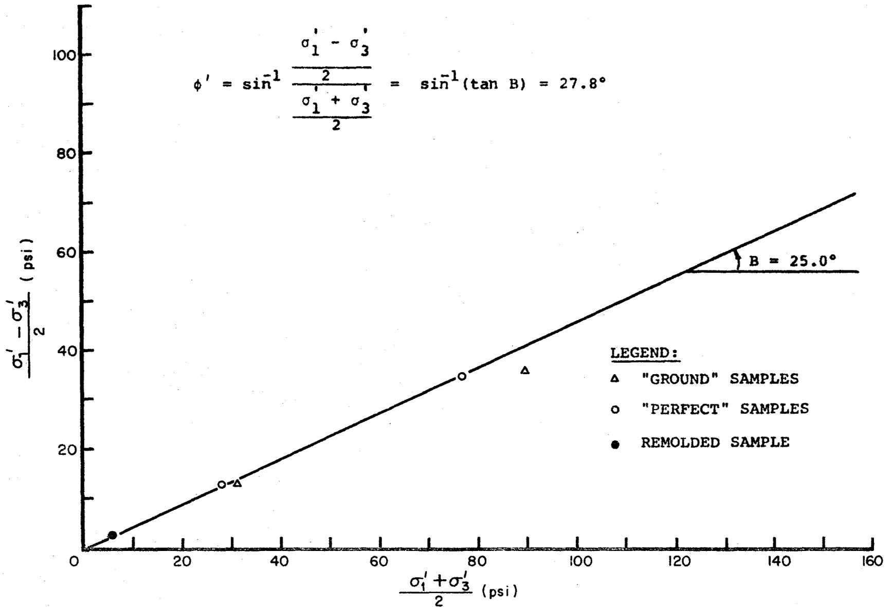
FIG. 14. FAILURE ENVELOPE OF "SILTY CLAY" at  $(\sigma_1 - \sigma_3)_{max}$ .
