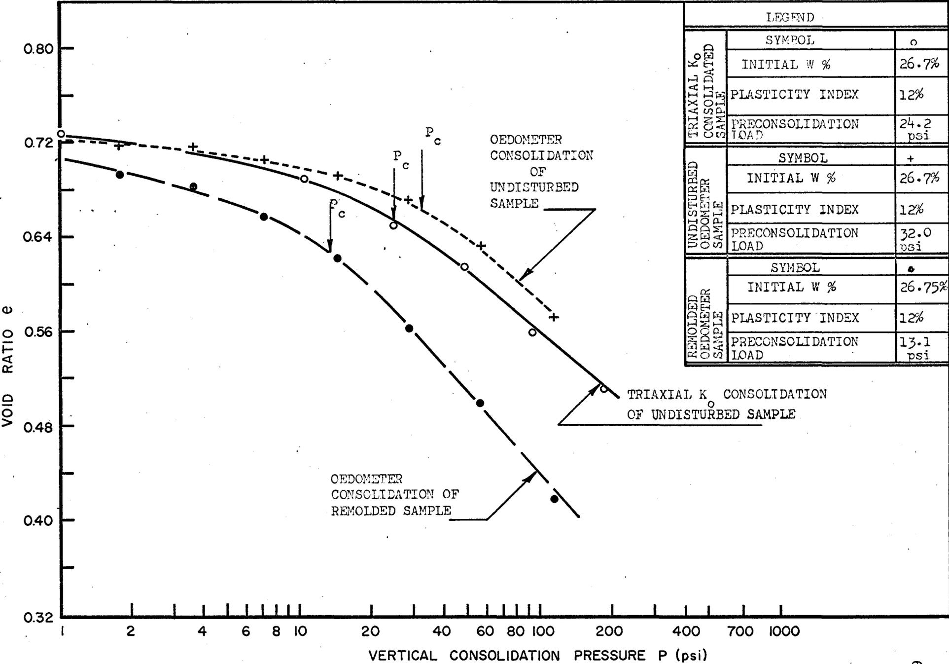
FIG. 19 . FACTORS INFLUENCING PRECONSOLIDATION LOAD DETERMINATION.
