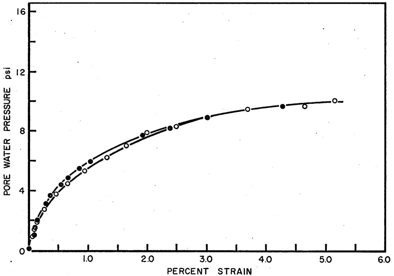
FIG. 25 . EFFECTS OF STRAIN RATE ON STRESS-STRAIN RELATIONS.
