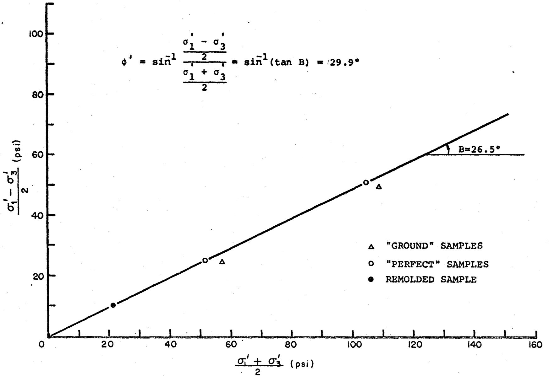
FIG. 15 . FAILURE ENVELOPE OF "CLAYEY SILT" AT  $(\sigma_1 - \sigma_3)_{max}$  .
