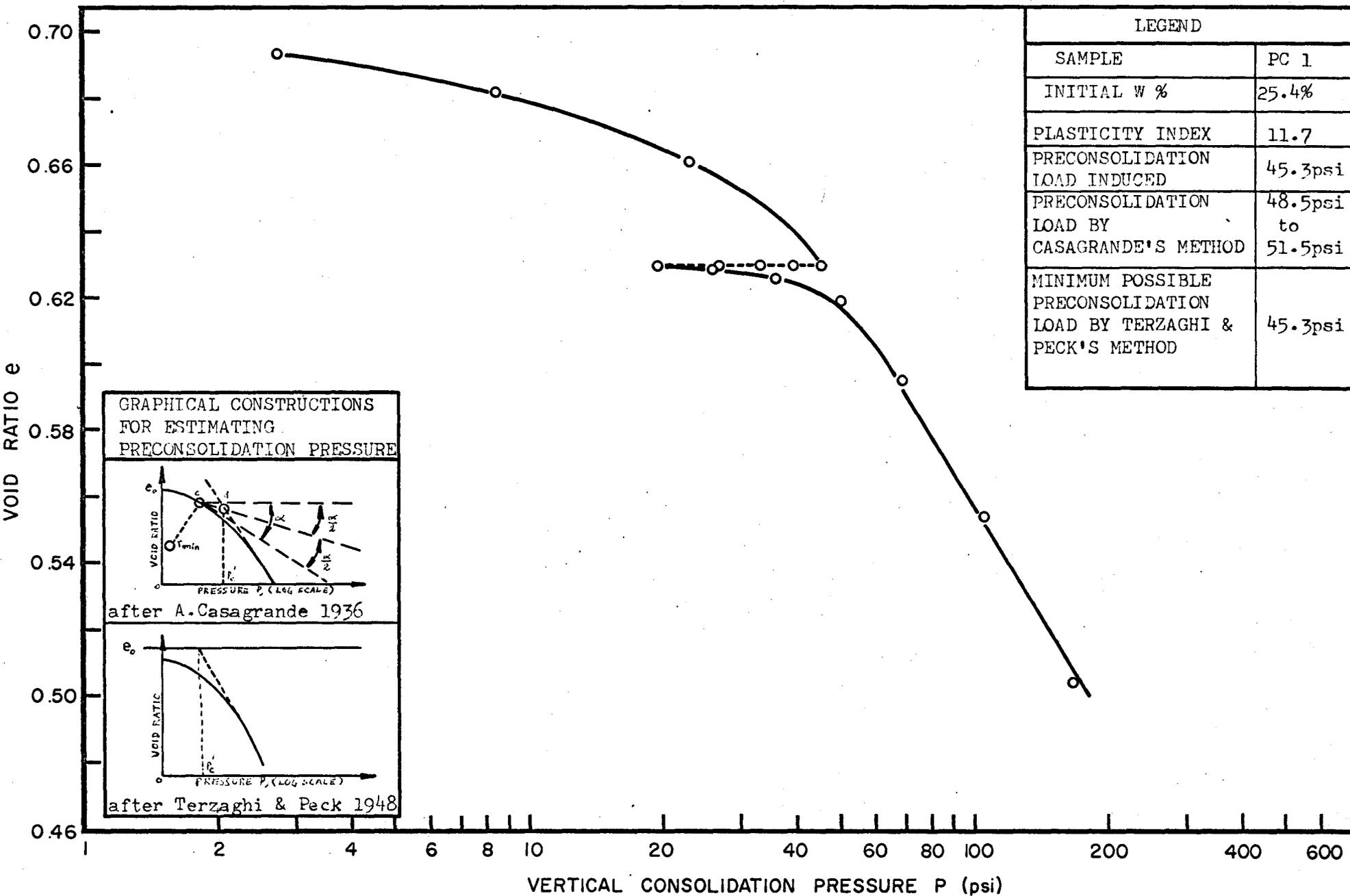
FIG. 17. EFFECT OF "PERFECT" SAMPLING CYCLE — TRIAXIAL  $K_0$  CONSOLIDATION —
