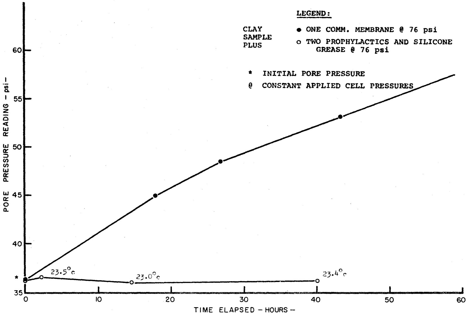
FIG. 24 . OBSERVATIONS OF PORE PRESSURE CLIMB - with a SOIL SPECIMEN -
