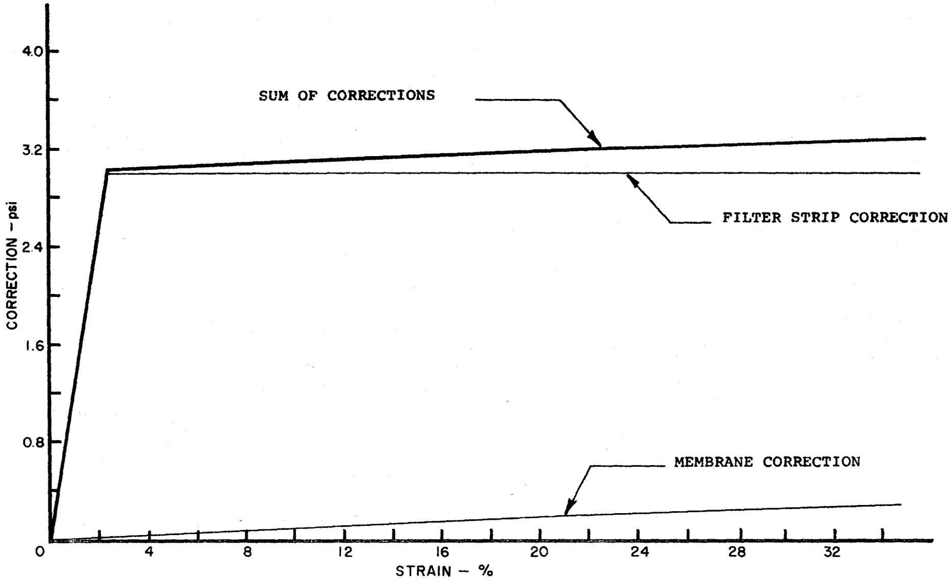
FIG. 22 . DEVIATOR STRESS CORRECTIONS.
