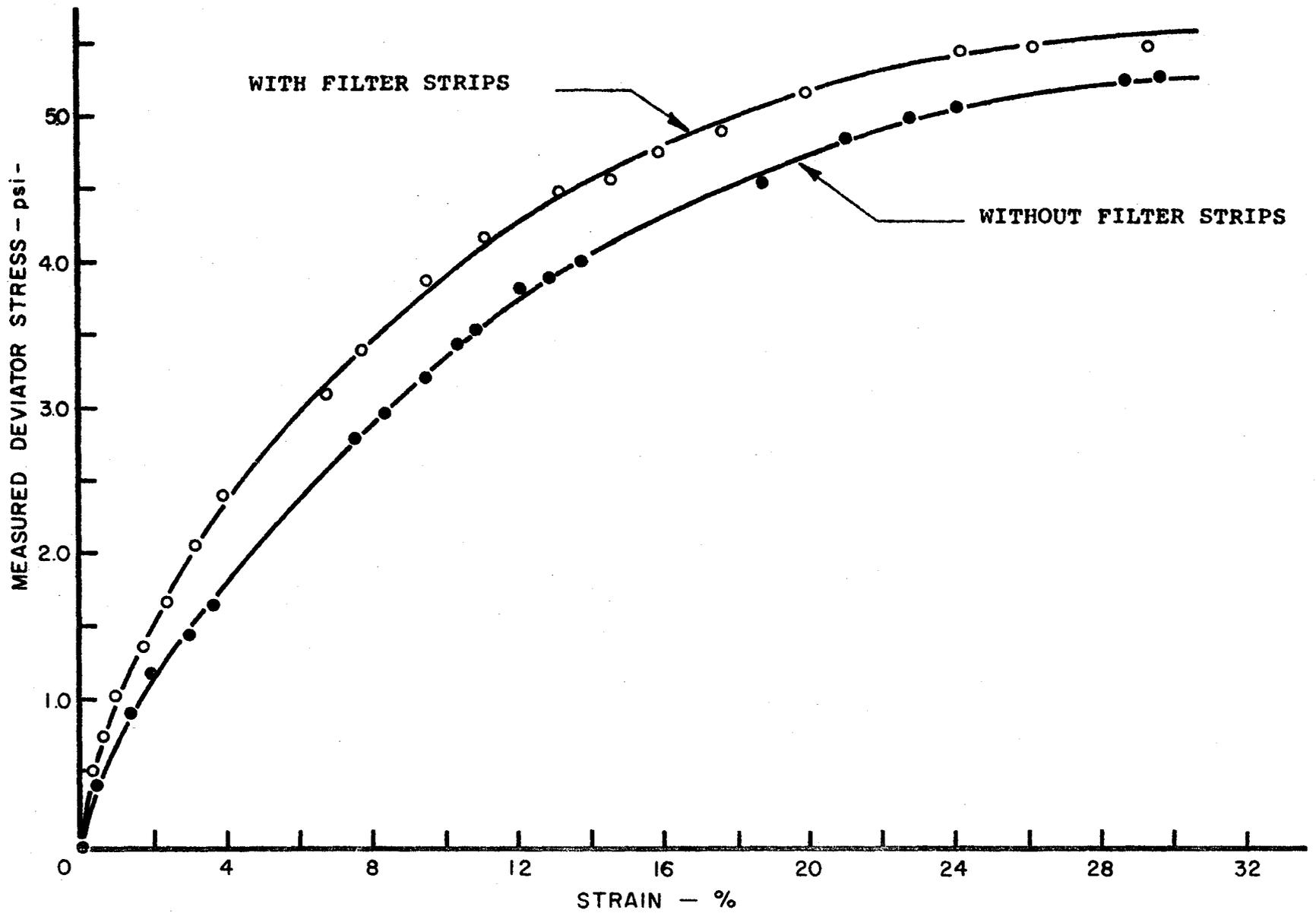
FIG. 21. STRESS-STRAIN CURVES FOR SOFT SOILS - WITH and WITHOUT FILTER STRIPS -
