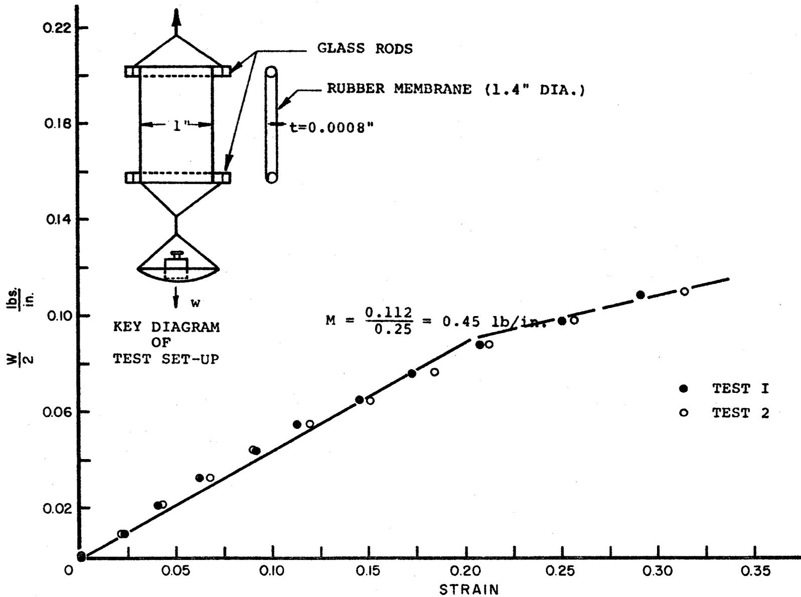
FIG. 20. MEMBRANE (PROPHYLACTIC) EXTENSION MODULUS TEST.
