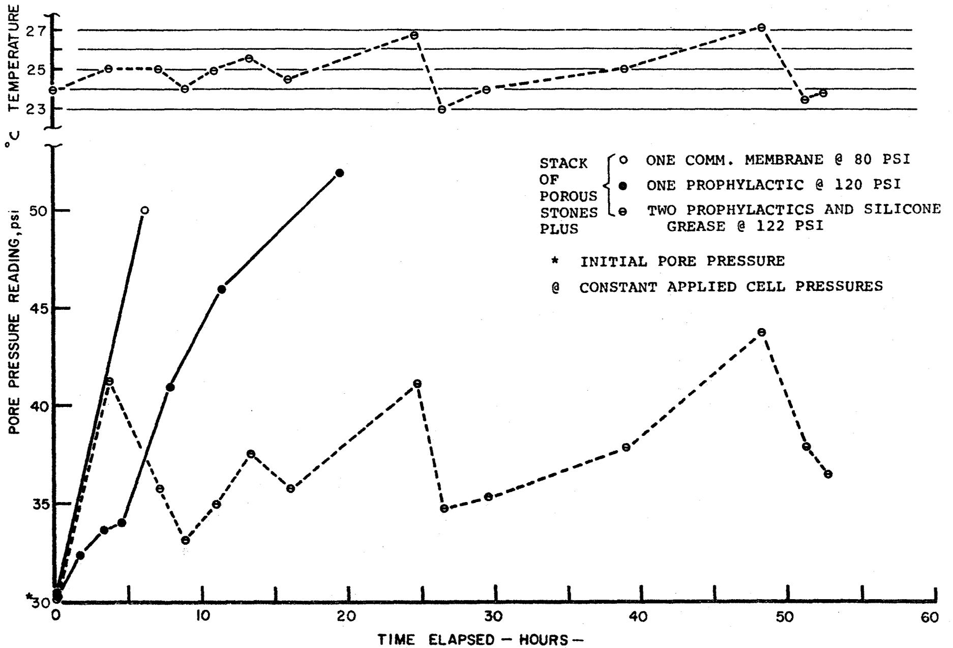
FIG. 23. OBSERVATIONS OF PORE PRESSURE CLIMB - with SATURATED POROUS STONES -
