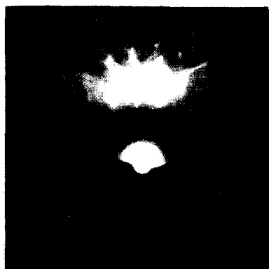
Fig. (4-1): HEED patterns obtained from 3000 Å silicon layers evaporated onto Si<111>substrates having temperatures 700°C, 600°C and from the substrate material.
