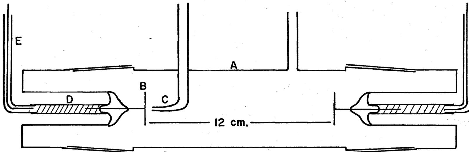
Figure 10. THE ELECTROLYSIS CELL A. Pyrex glass tubing B. Platinum Electrode C. Luggin capillary D. Tubing containing mercury E. Glass envelope containing connecting wire
