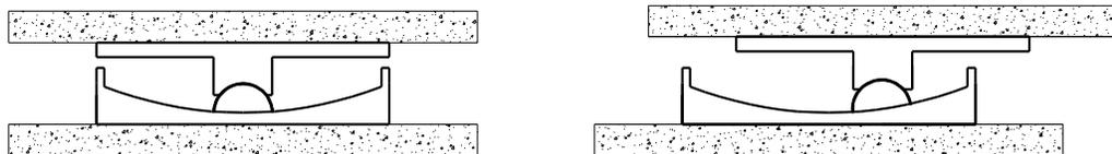
Figure 1-3: Friction Pendulum System
