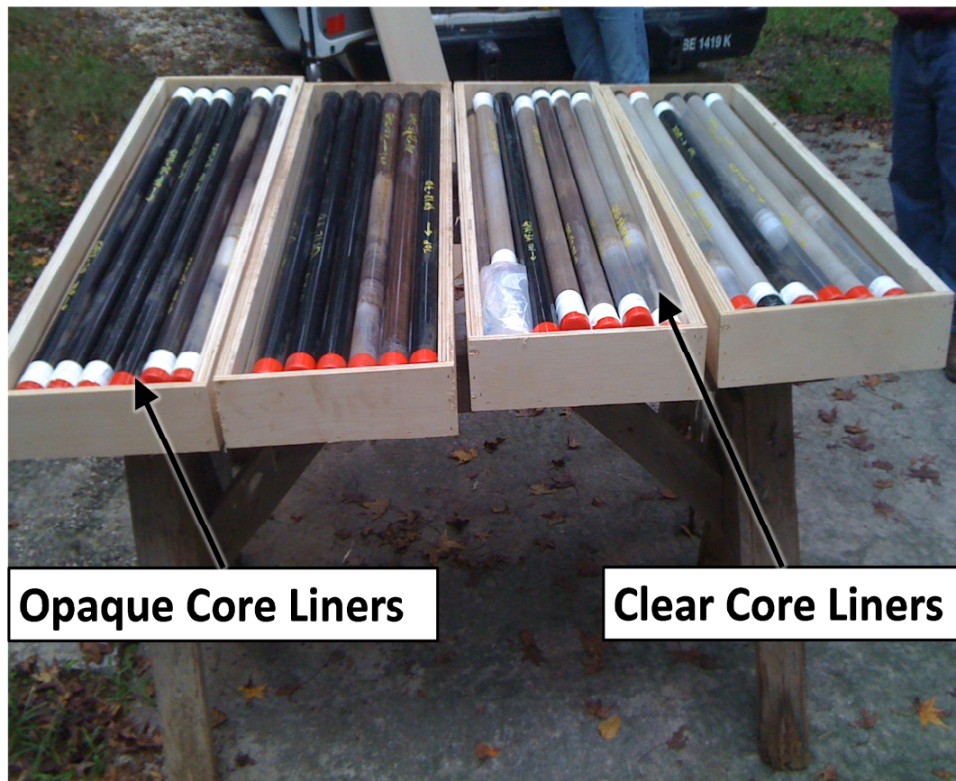
Figure 21: Core liners used to collect the core for lithologic logging (clear) and geochronology (opaque black).
