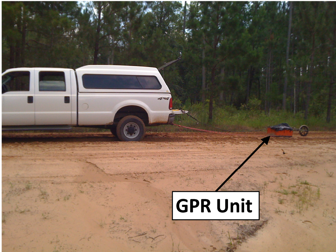
Figure 20: Set up of the GPR survey with a truck pulling the GPR unit behind it.
