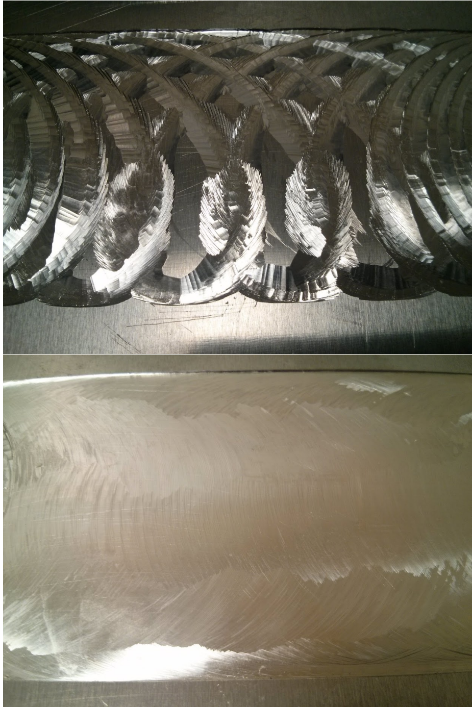
Figure 4.11: Images of the machined thin plate without magnetic damping (top) and with magnetic damping (bottom)
