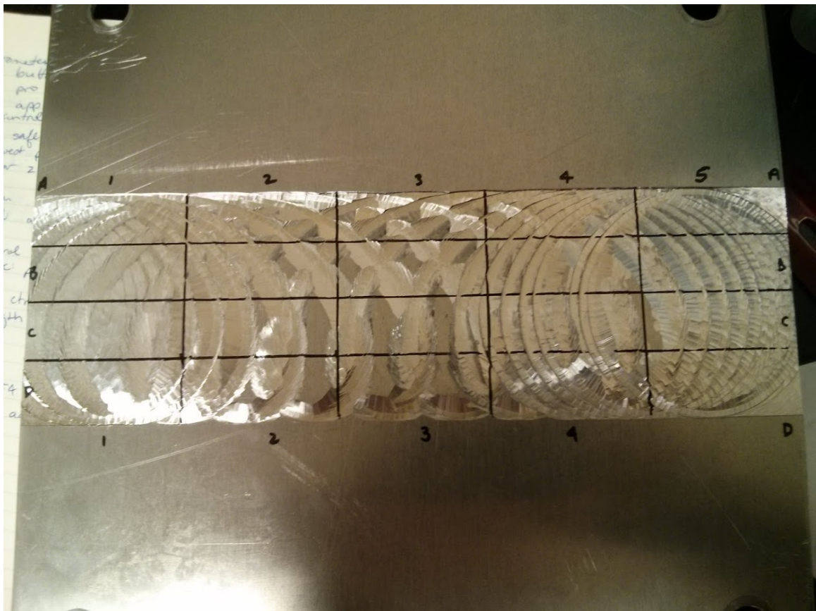
Figure 4.16: Flat plate surface roughness measurement locations; columns are designated 1 through 5 from left to right and rows are designated A through D from top to bottom
