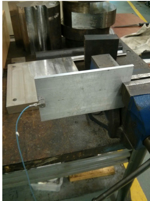
Figure 4.5: Images of the undamped impact test setup
