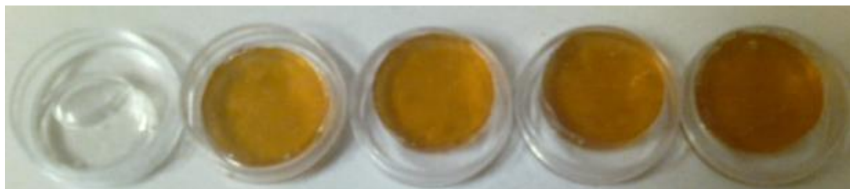
Figure 2.7. A photograph of the reference, pre-irradiation, and post-irradiation for the 15% (three FTCs) 20/80 water/DMSO dosimeter system.
