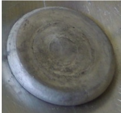
Figure 5.34. A defect-free UPJ head from AM60 protrusion formed with a very high maximum current, a high CSTP and a low compression rate.
