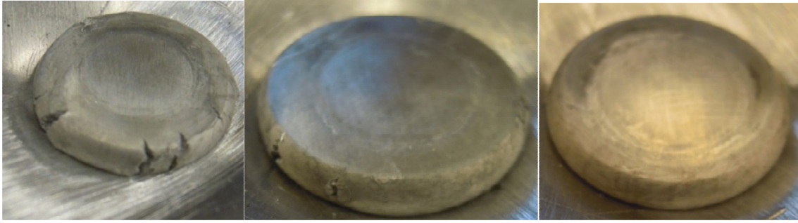
Figure 5.54. Three repeat tests for AM60 alloy based on Taguchi optimal process variables. The protrusions were compressed at a rapid rate, a low maximum current and a high CSTP.
