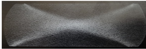
Figure 2.7. Shear bands forming an X shape within a mild steel cylinder deformed at room temperature with high-friction platens (Semiatin & Jonas, 1984).
