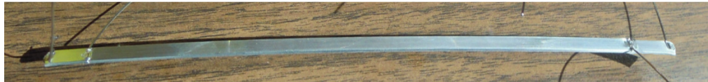
Figure 4.12. A precision magnesium AZ91 sample with aluminum wires bonded to the specimen. This design was arrived at after several iterations of sample jigs, machining practices, and specimen geometry.
