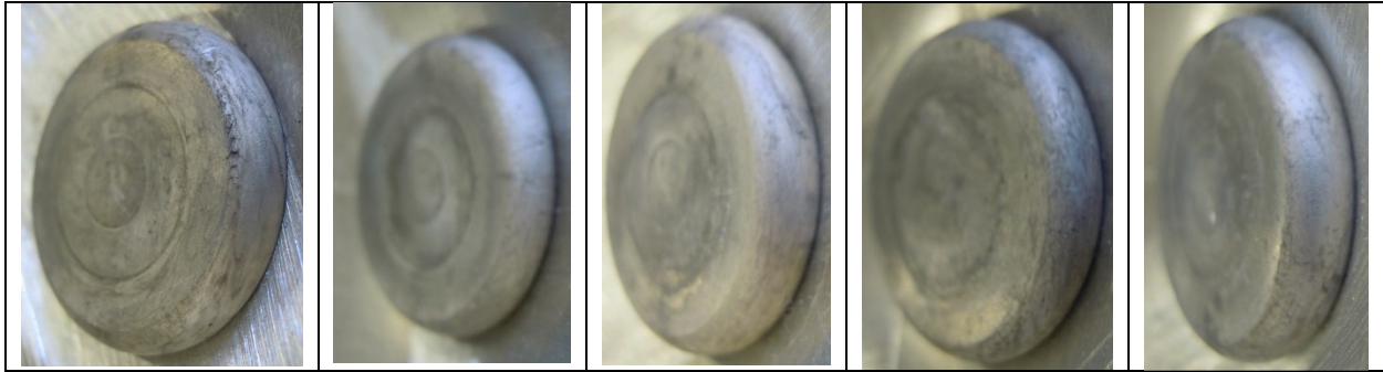
Figure 5.31. A comparison of visual appearance of UPJ heads from 5 repeat tests. Four of the 5 tests did not indicate any cracks or fissures, while the fifth (left most) had small surface cracks on the top edge that did not penetrate into the protrusion.
