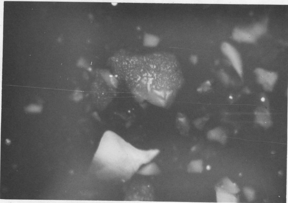
Plate 6. CaF 2 -rich glass with spherulitic structure, cross polarized light, x 125.
