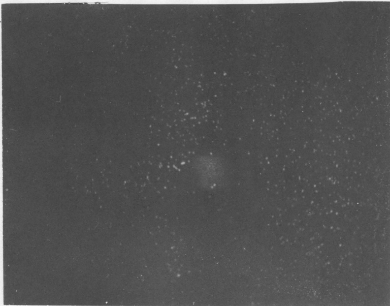
Plate 18. Showing the distribution of Mg atom in the same object as the plate 16 \text{MgK}\alpha radiation, x 2500.
