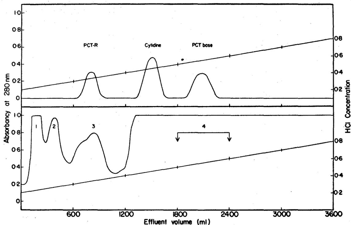
**Figure 17 a.** Elution pattern of PCT.R, cytidine and PCT from a 2 cm x 30 cm column of Dowex-50W-X8 ( $H^+$ , 200-400 mesh) eluted with a linear gradient of hydrochloric acid (0.2 N - 0.8 N, total volume 3.6 l).
