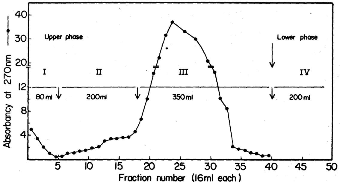
Figure 13. Celite-545 partition chromatography of an enzymic digest of 1 g of yeast tRNA, solvent E (column 2.5 cm in diameter, containing 120 g of Celite-545).
