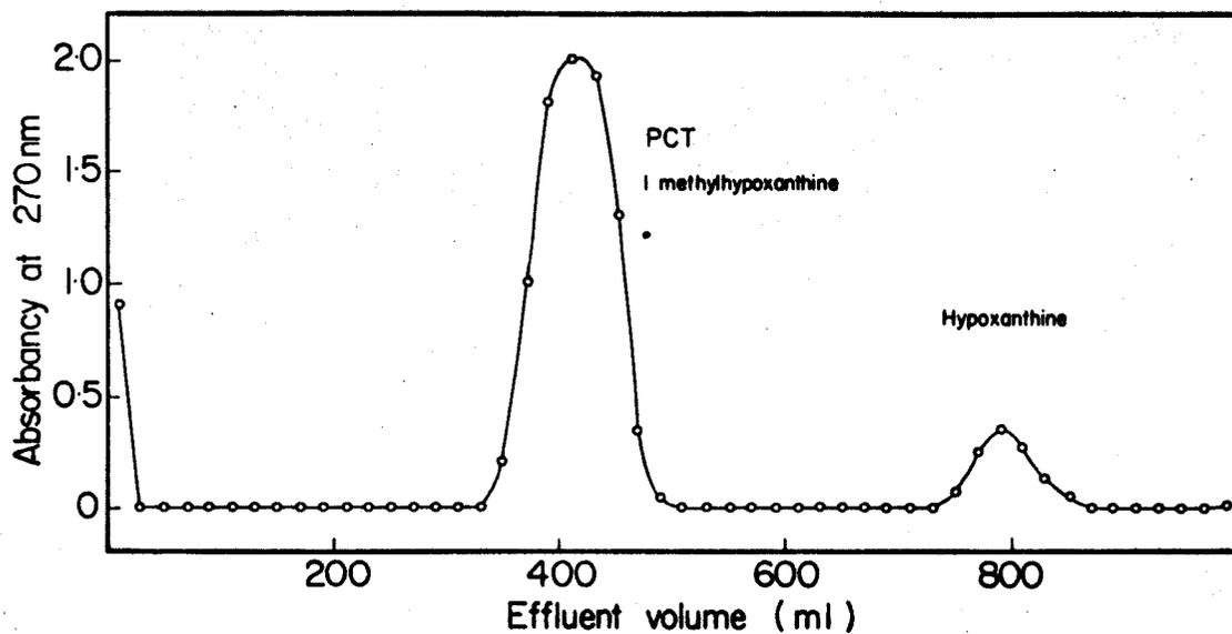
**Figure 18.** Fractionation of the material of fraction 3 (fig. 17) on a Celite-545 column (2 cm x 40 cm) with solvent F.
