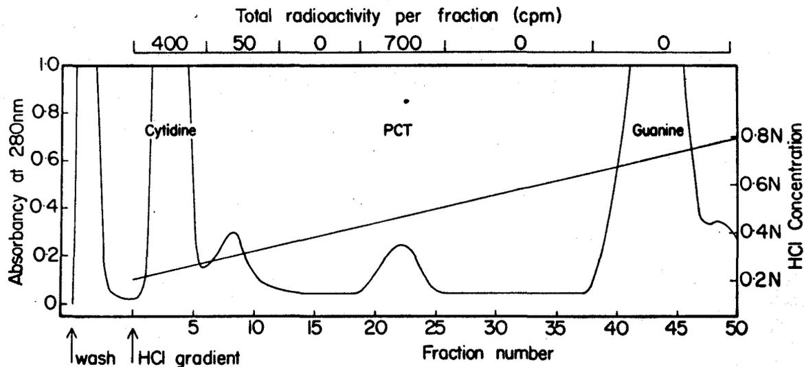
**Figure 5.** Isolation of N-(purin-6-ylcarbamoyl)-threonine from an hydrochloric acid hydrolysate of tobacco tissue on a 1 cm x 10 cm column of Dowex 50W-X8 ( $H^+$ , 200-400 mesh). The column was eluted with a linear gradient of hydrochloric acid (0.2 N - 0.8 N, total volume 500 ml).
