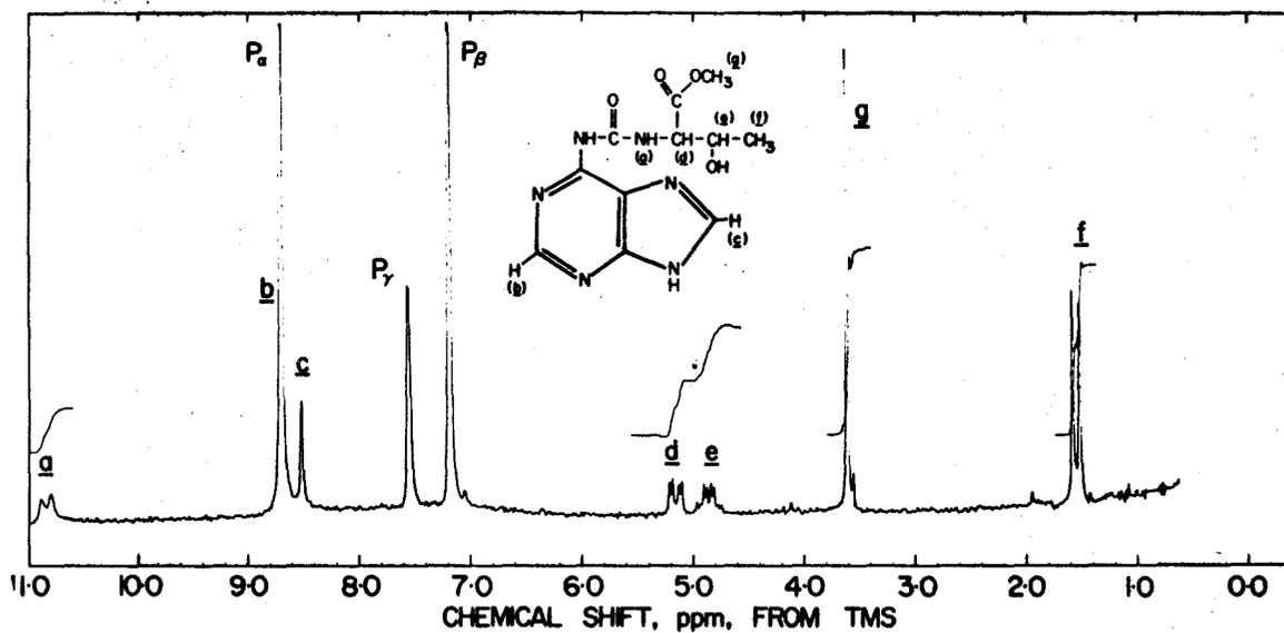
**Figure 22.** 100 MHz nuclear magnetic resonance spectra of N-(purin-6-ylcarbamoyl)threonine (top) (structure after Schweizer et al., 1969) and product 1 (bottom) in pyridine- $d_5$ .
