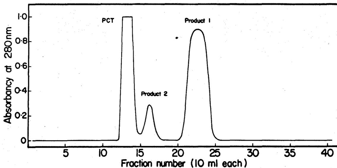
Figure 20. Separation of the 2 products of an acid-catalyzed reaction of PCT with methanol by Sephadex LH-20 chromatography. The standard column is eluted with 35% aqueous ethanol, normal pH 5.8.
