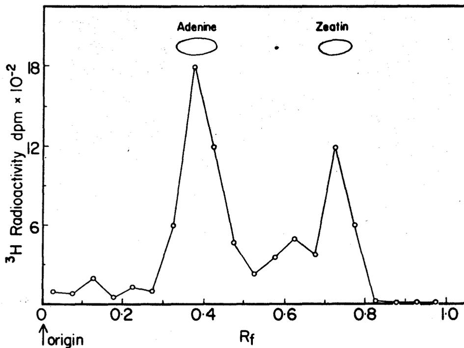
**Figure 12.** Paper chromatography purification of the zeatin fraction obtained after Sephadex LH-20 chromatography (fig. 11). The chromatogram was cut into 20 pieces and each piece was counted in a liquid scintillation counter.
