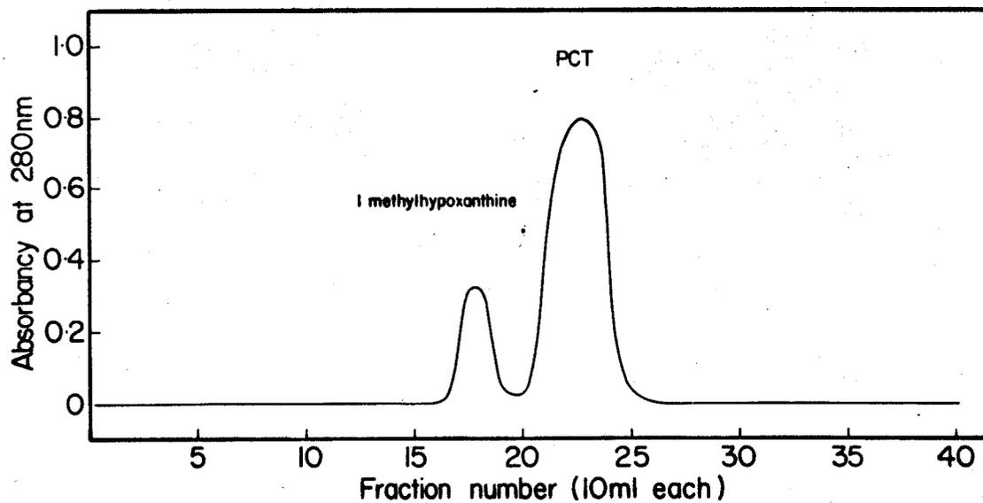
**Figure 19.** Separation of PCT from 1-methylhypoxanthine on a standard Sephadex LH-20 column, eluted with 35% aqueous ethanol, pH 2.5.
