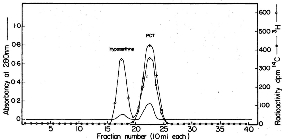
Figure 7. Purification of N-(purin-6-ylcarbamoyl)-threonine after Dowex-50W-X8 column chromatography on a Sephadex LH-20 column (50 g, 2.5 cm x 40 cm). The column was eluted with 35% aqueous ethanol, pH 2.5. Radioactivity was measured on 1 ml aliquot of each fraction.
