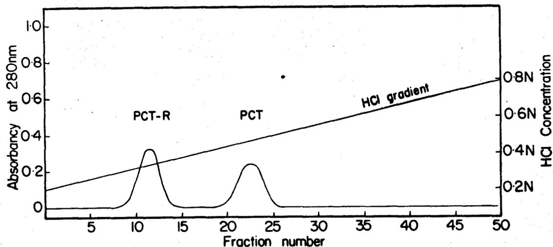
**Figure 8.** Separation of a mixture of PCT-R and PCT added to 50 ml of Rhizopogon medium by Dowex-50 column chromatography (1 cm x 15 cm). The column is washed with 100 ml of 0.001 N HCl and eluted as in figure 5.
