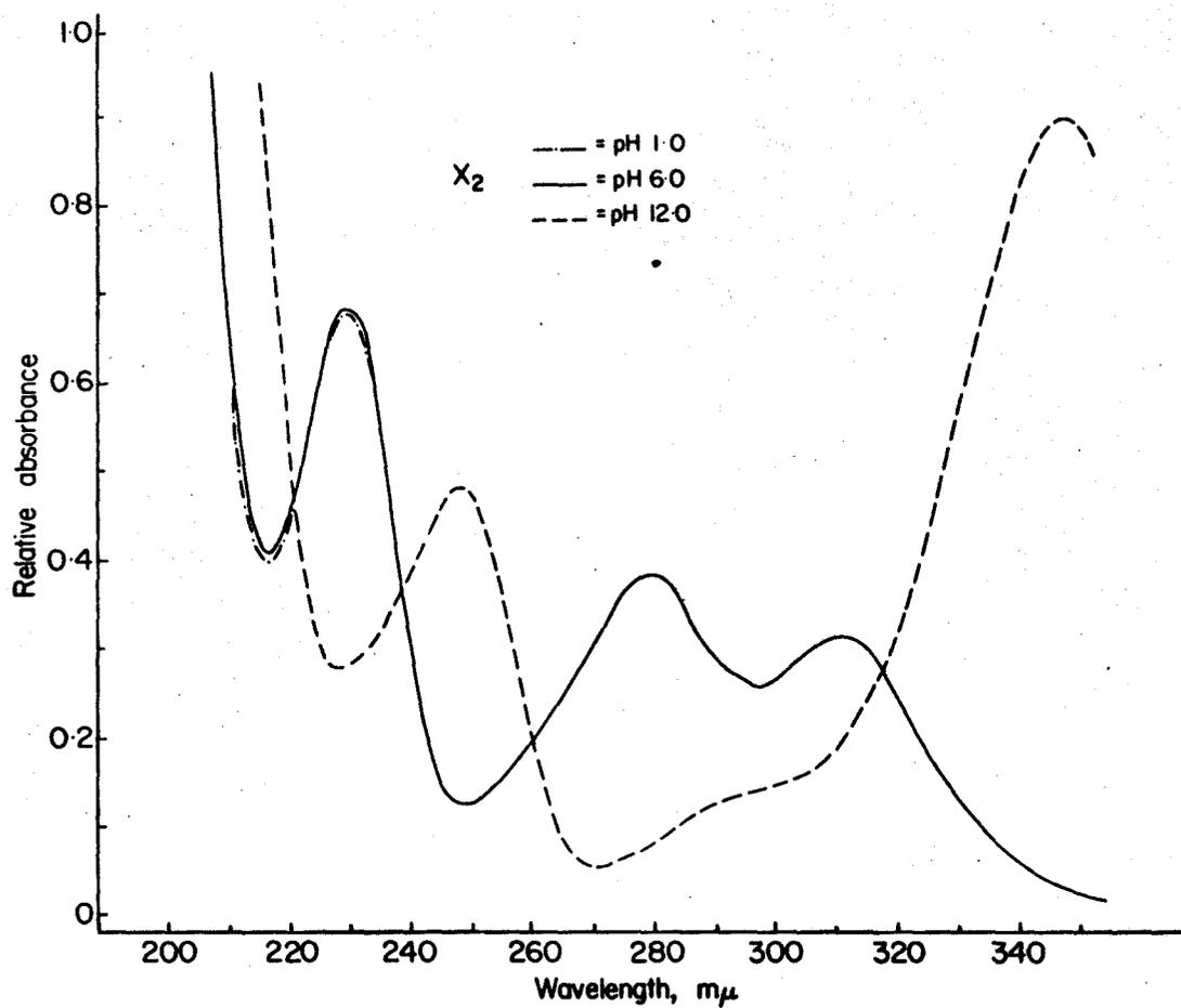
**Figure 15.** Ultraviolet absorption spectra of compound X<sub>2</sub> (fig. 14b), a contaminant extracted from Celite-545.
