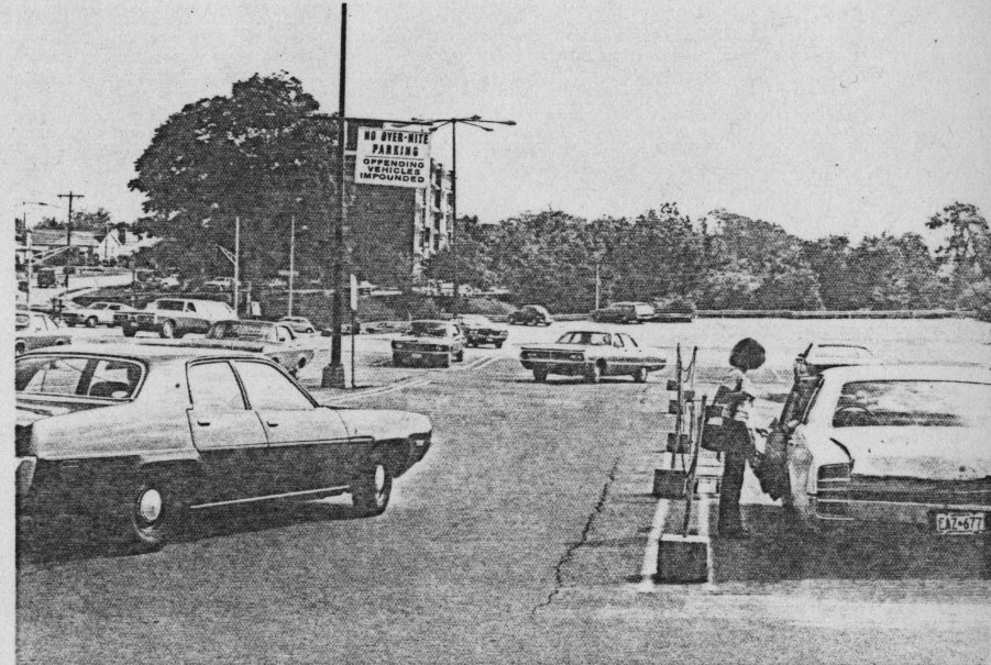
(b) Looking north along the major axis, the poor pavement markings offer a confusing route to drivers. The narrow passage opens possibilities for bottlenecks to occur at moment's notice.
