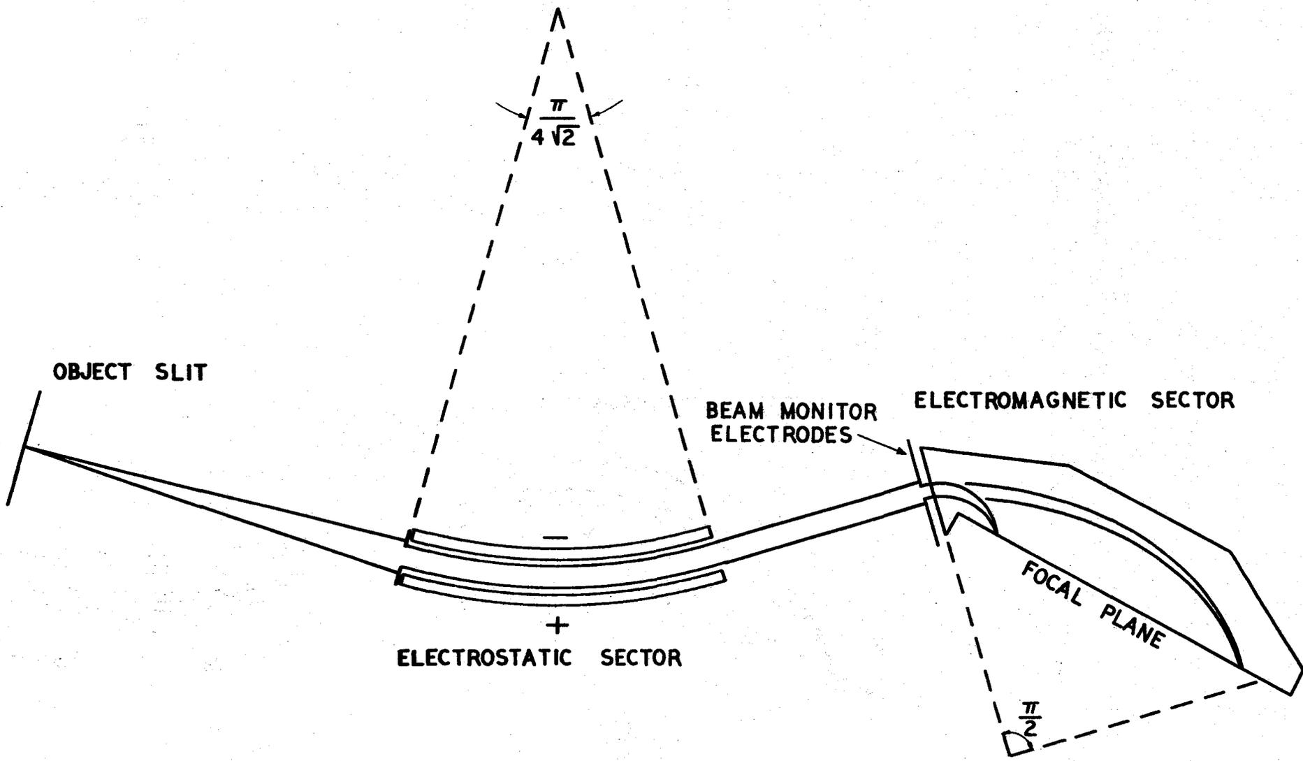
Figure 2: Double Focusing Design of Mattauch and Herzog
