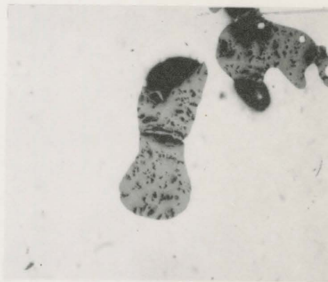
Fig. 5.24a Micrograph of FeV_2O_4 inclusions. Ingot No. 661 (0.09%V)
