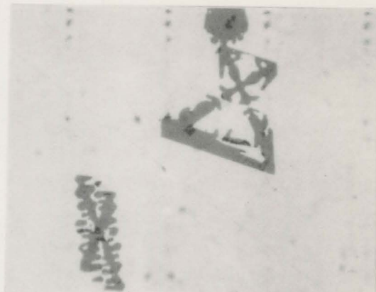
Fig. 5.24a Micrograph of FeV_2O_4 inclusions. Ingot No. 661 (0.09%V)
