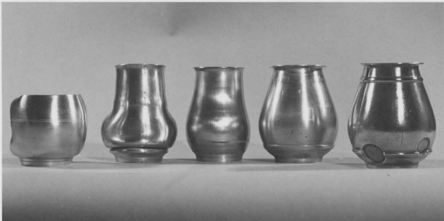
Figure 31- L to R -- (a) Rubber plug formed cup (b) Wrinkle produced due to excessive sealing load (c) Premature rupture due to localised thinning in semisuperplastic preform (d) As cast cup-- held at 250 psi for 20 minutes (e) Superplastic preform--250 psi for 1.5 minutes
