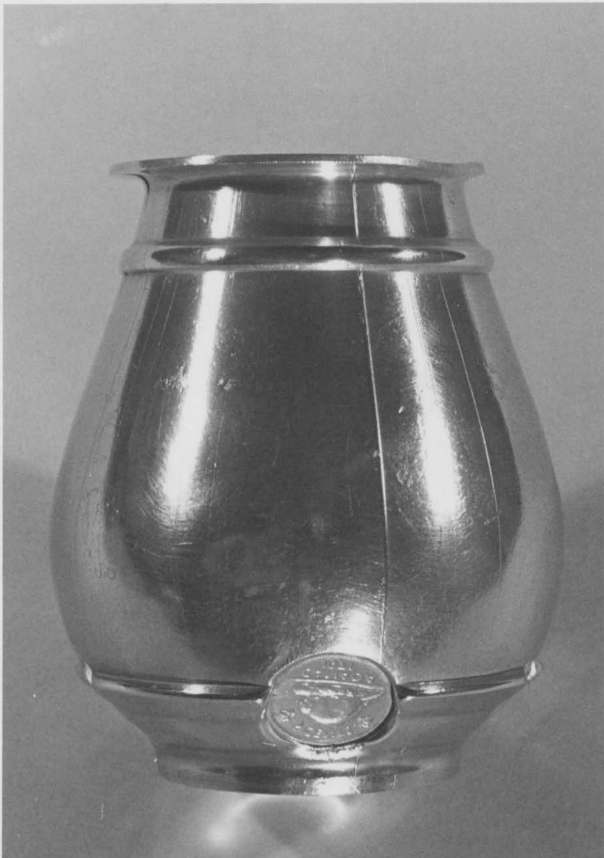
Figure 30- Pressure formed cup--250 psi, 5 minutes
