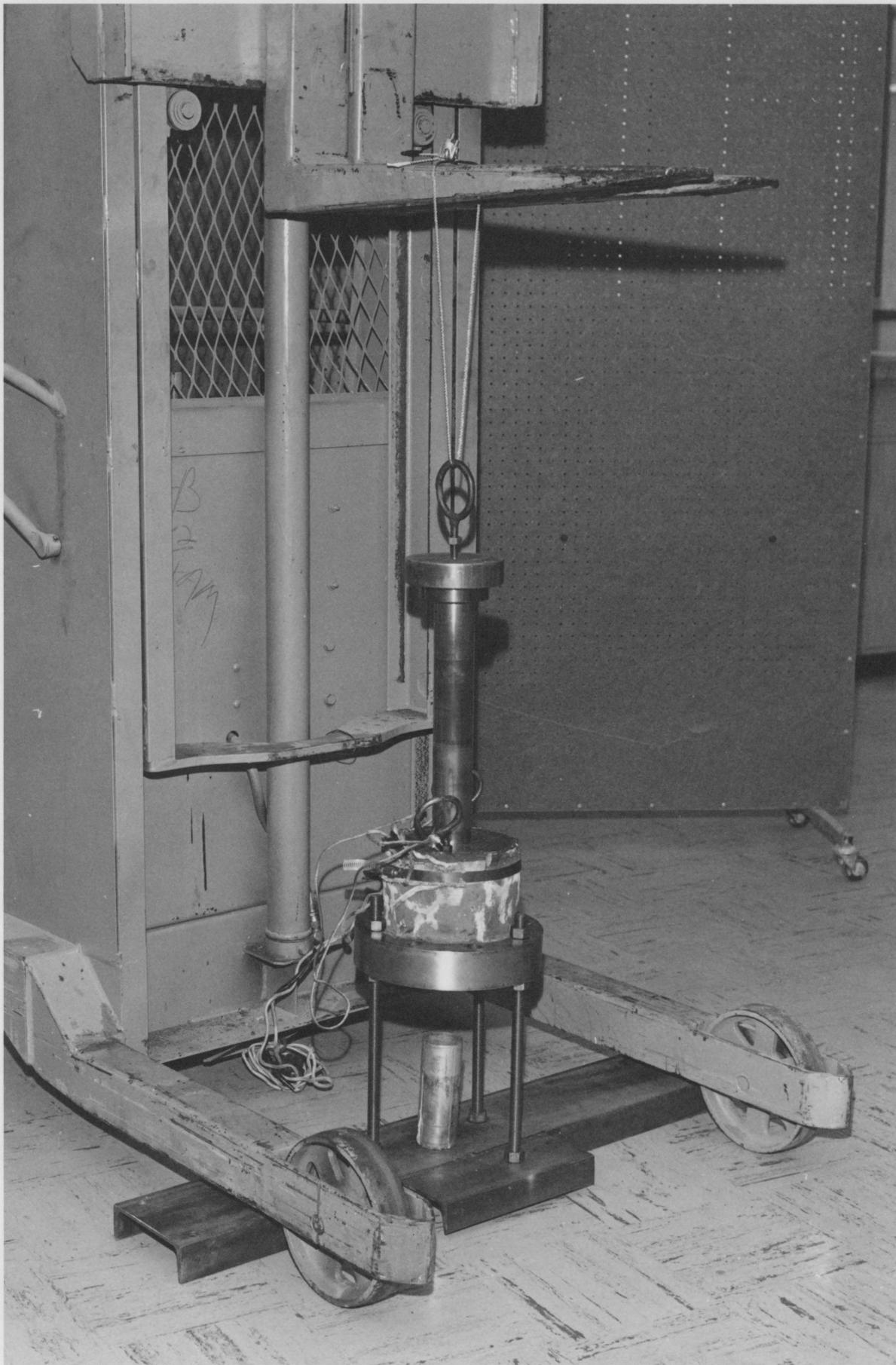
Figure 19- Removal of extruded cup from ram
