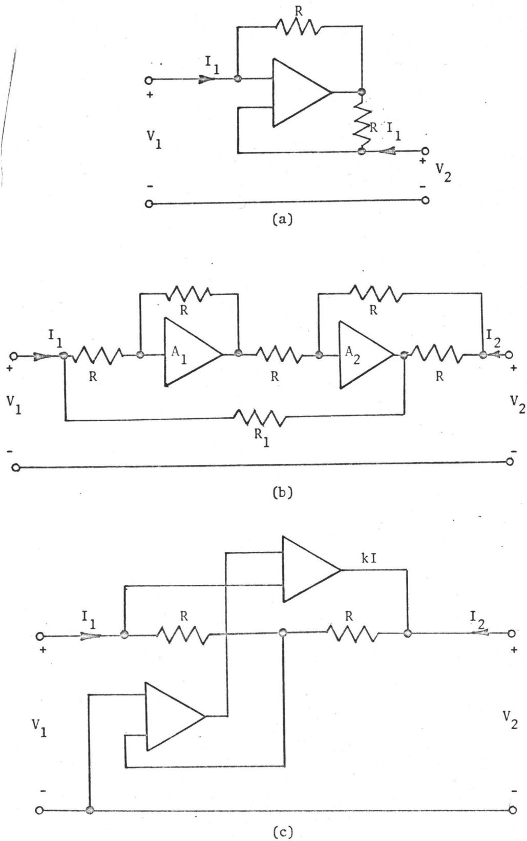
FIGURE 2-18: Practical Negative Impedance Converters Using Operational Amplifiers
