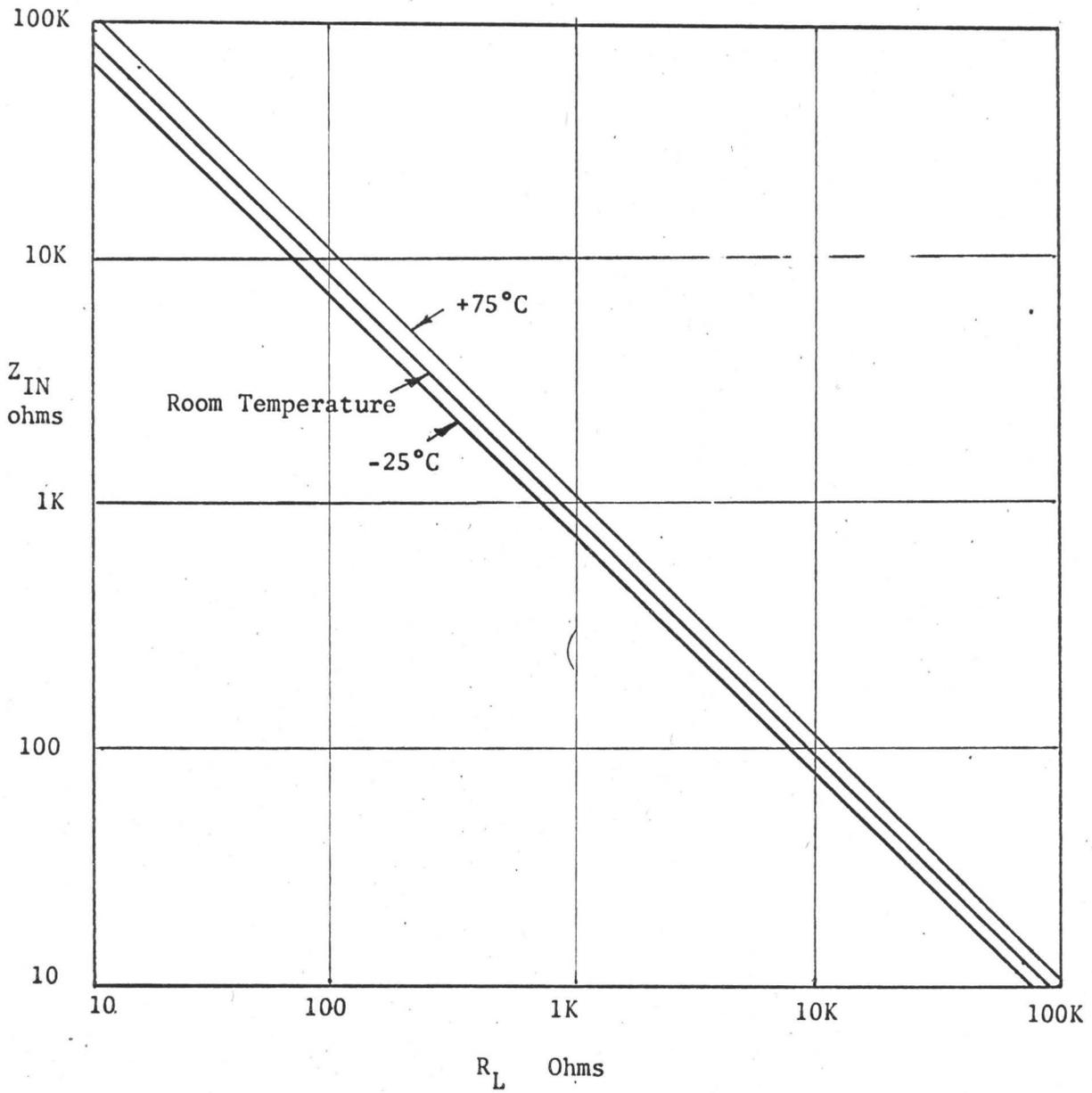
FIGURE 5-1: Input Impedance of Resistive Terminated Gyrator
