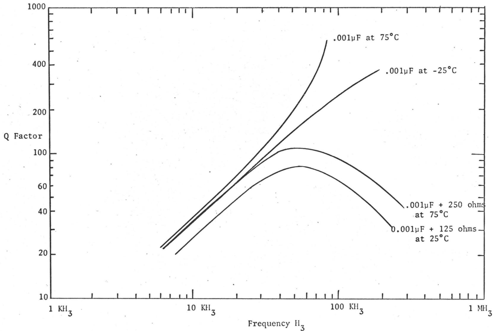
FIGURE 5-8: Q Factor Variation with Temperature and Compensation at High Frequencies
