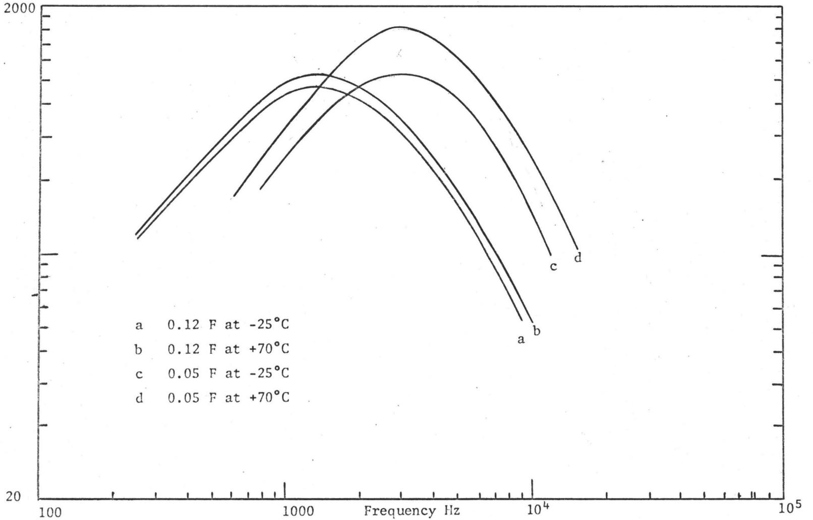
FIGURE 2(b): Q Factor Dependence on Temperature
