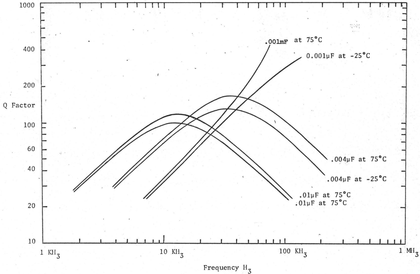
FIGURE 5-7: Q Factor Variation with Temperature at High Frequencies
