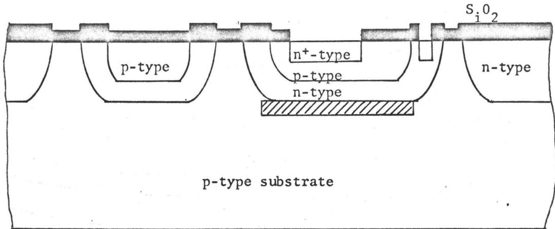
FIGURE 3-7: Cross Section of Emitter Diffusion
