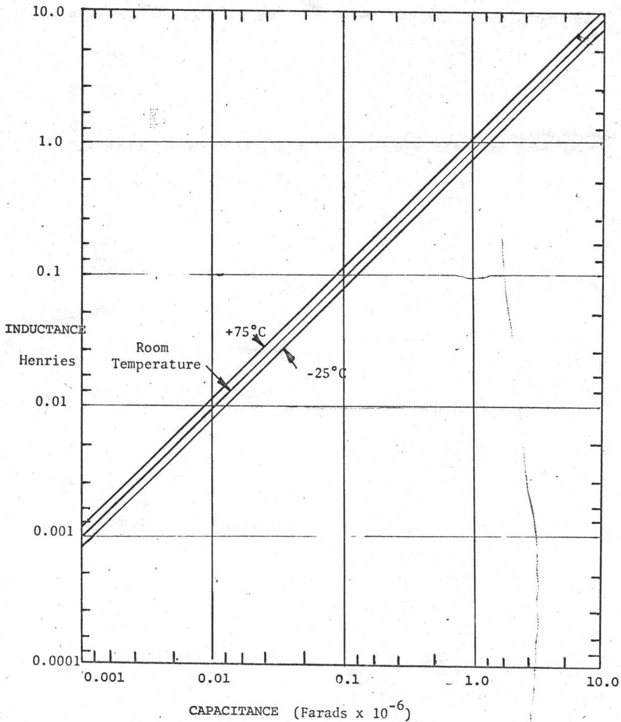
FIGURE 5-2: Input Impedance of Capacitive Terminated Gyrator
