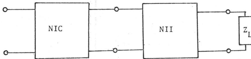
FIGURE 2-19: Gyrator Obtained Using a NII and a NIC
