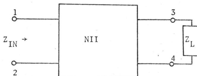
FIGURE 2-14: Negative Impedance Realized Using NII
