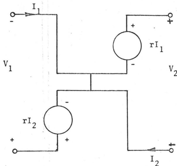
FIGURE 2-13: Series Connection of Two Transresistance Amplifiers
