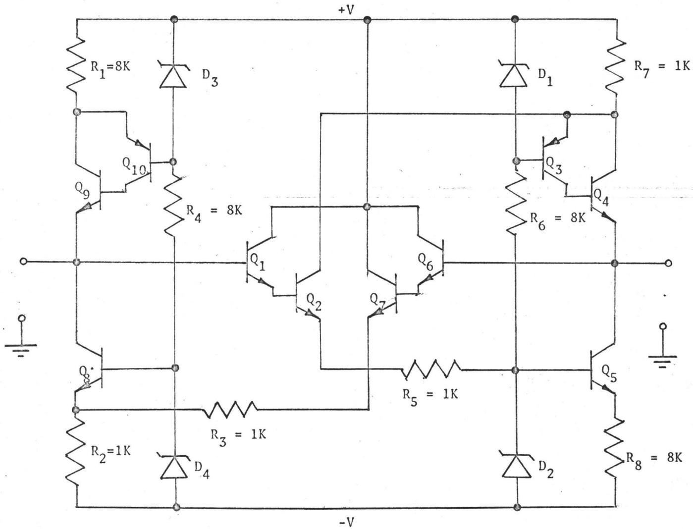
FIGURE 2-10: Improved Integrated Grounded Gyrator
