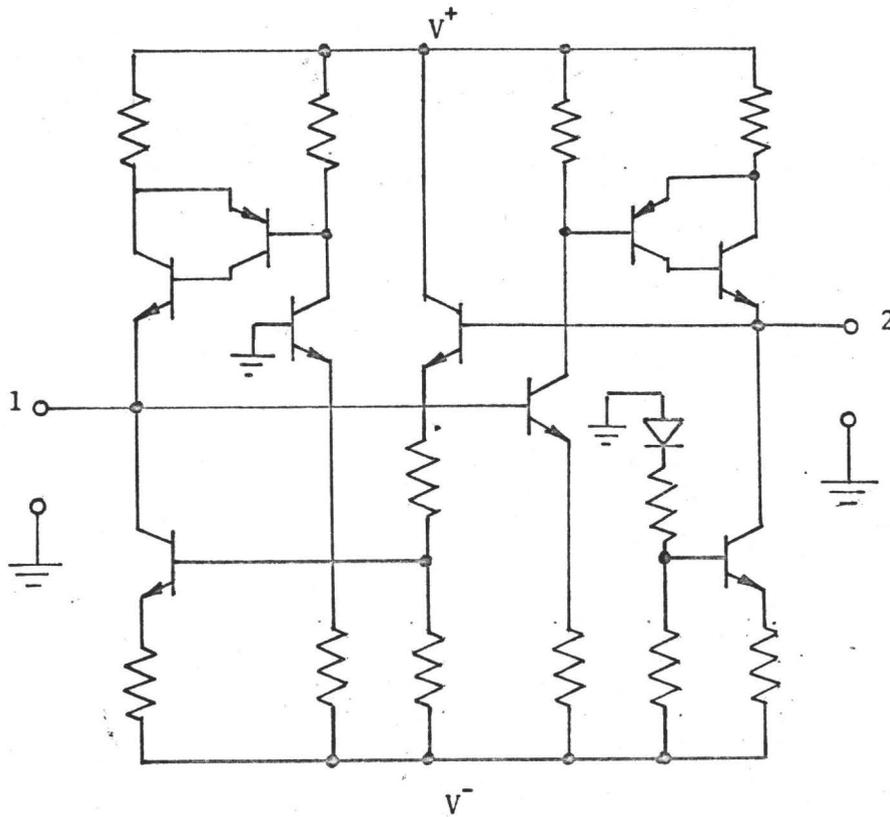
FIGURE 2-9: Direct Coupled Integrated Grounded Gyration
