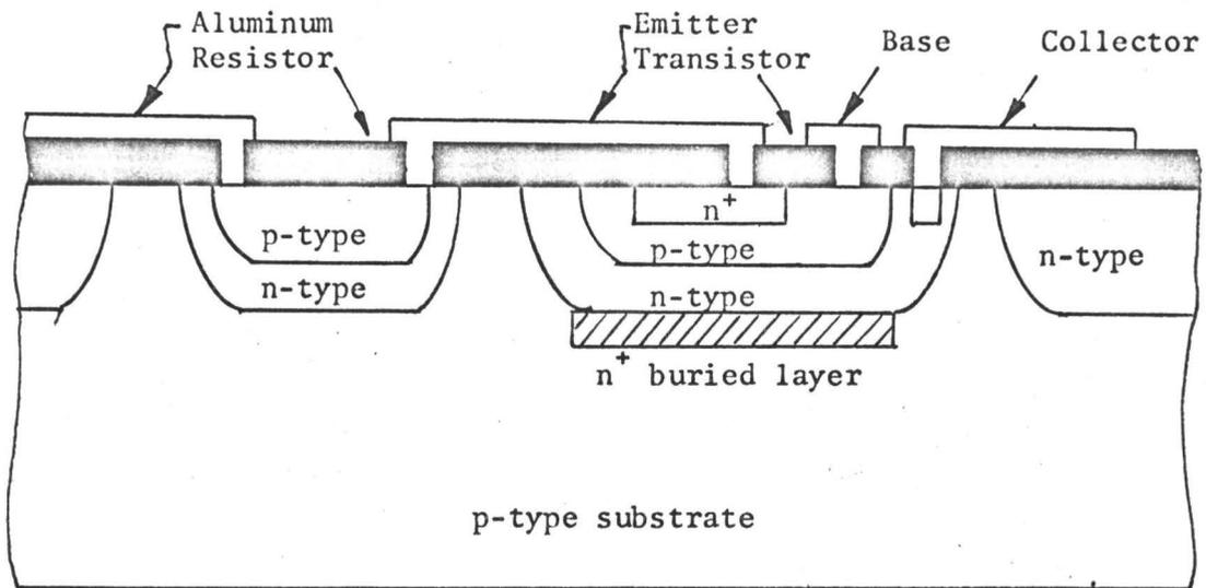
FIGURE 3-9(a): Cross Section of Aluminum Pattern
