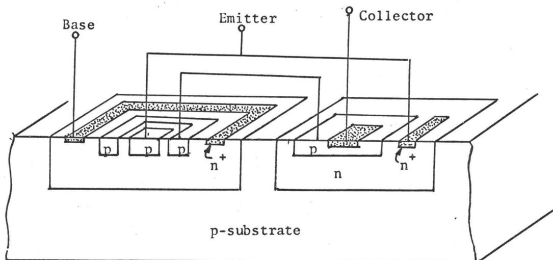
FIGURE 3-11(a): Cross Section of NPN-PNP Transistors
