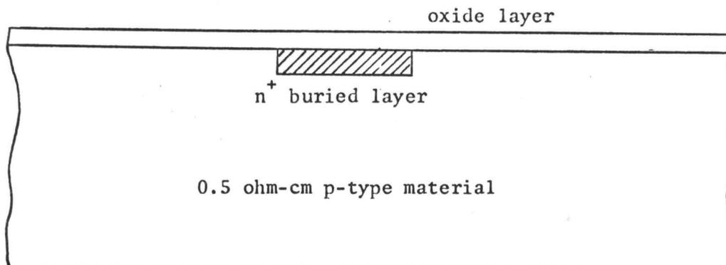
FIGURE 3-3: Cross Section of Buried Layer Diffusion
