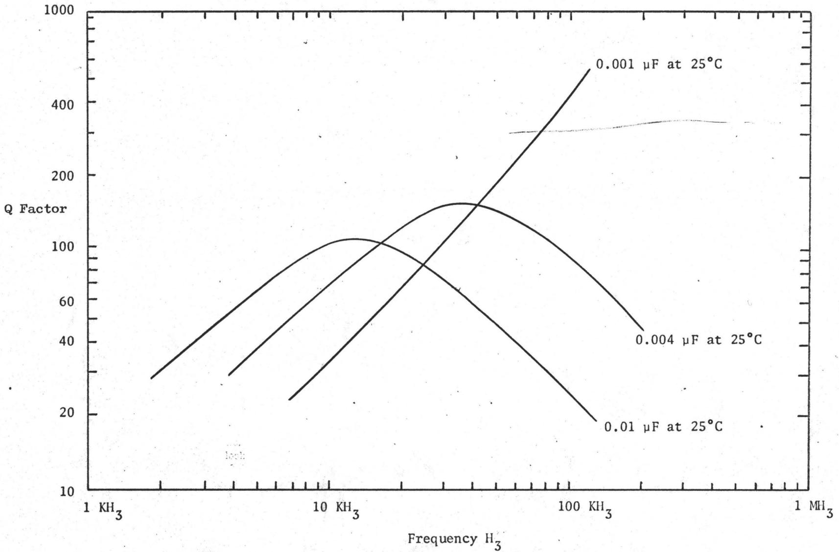
FIGURE 5-4: Q Factor at High Frequencies and Room Temperature
