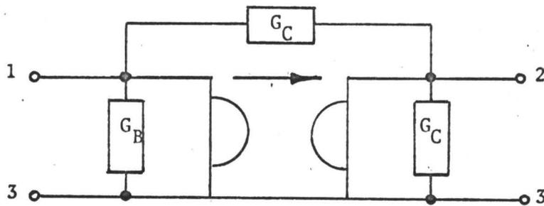
FIGURE 1-6: Equivalent  $\pi$  Network of Non-Ideal Gyrator
