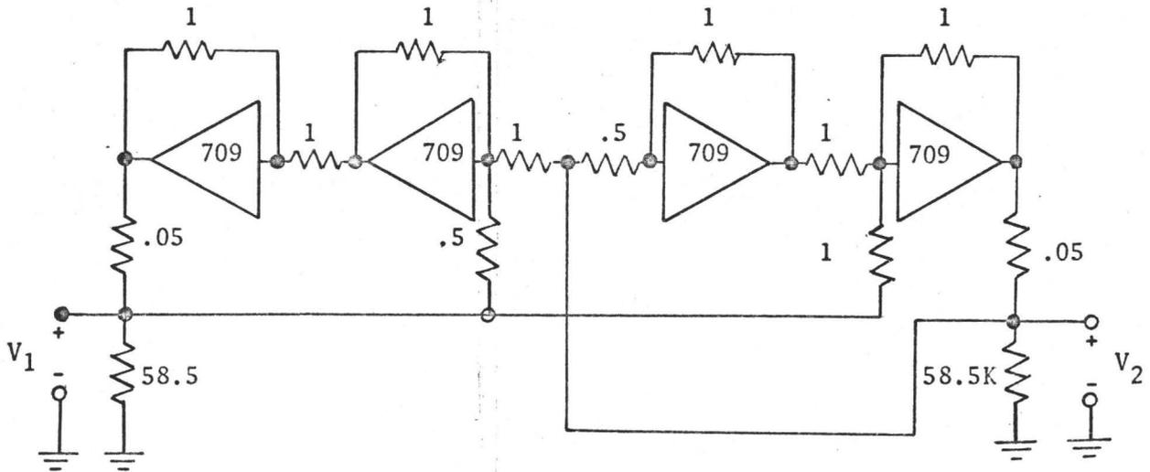
FIGURE 2-3: A Gyrator Realization Using Operational Amplifiers
