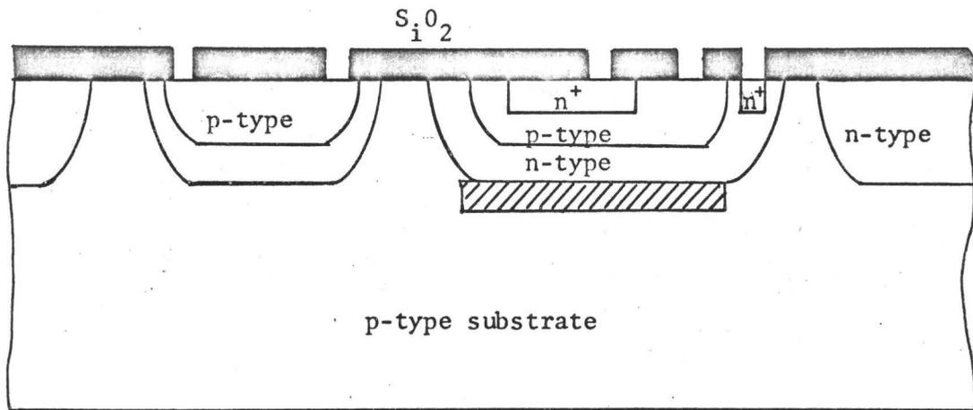
FIGURE 3-8: Cross Section of Openings for Metalization
