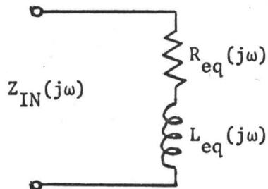
FIGURE 1-8: Equivalent Circuit of Simulated Inductor
