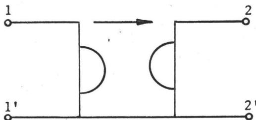
FIGURE 1-2: Equivalent Schematic of Gyrator
