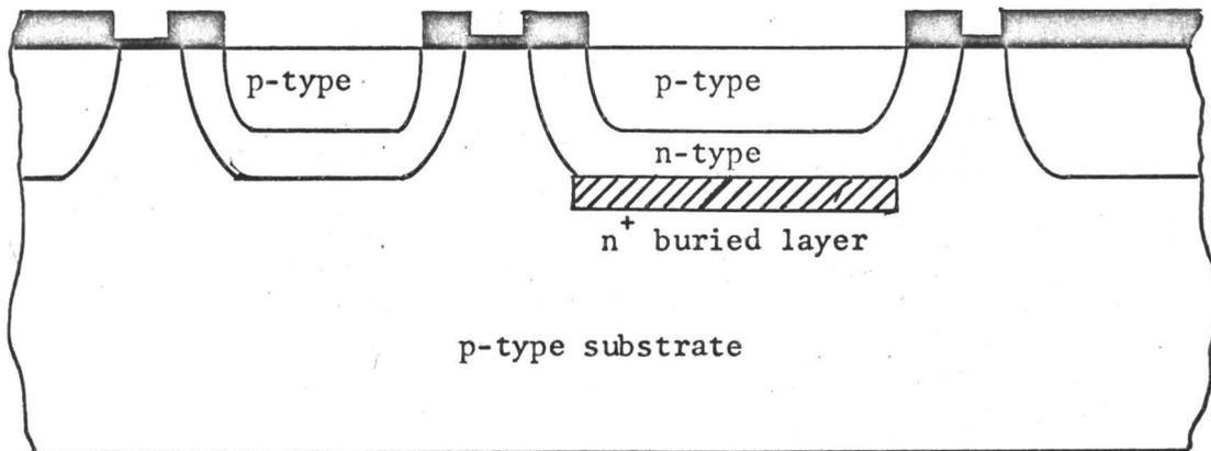
FIGURE 3-6: Cross Section of Base Diffusion
