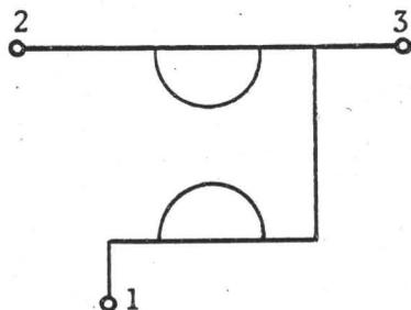
FIGURE 1-4: Grounded Gyrator Having Terminal 1
