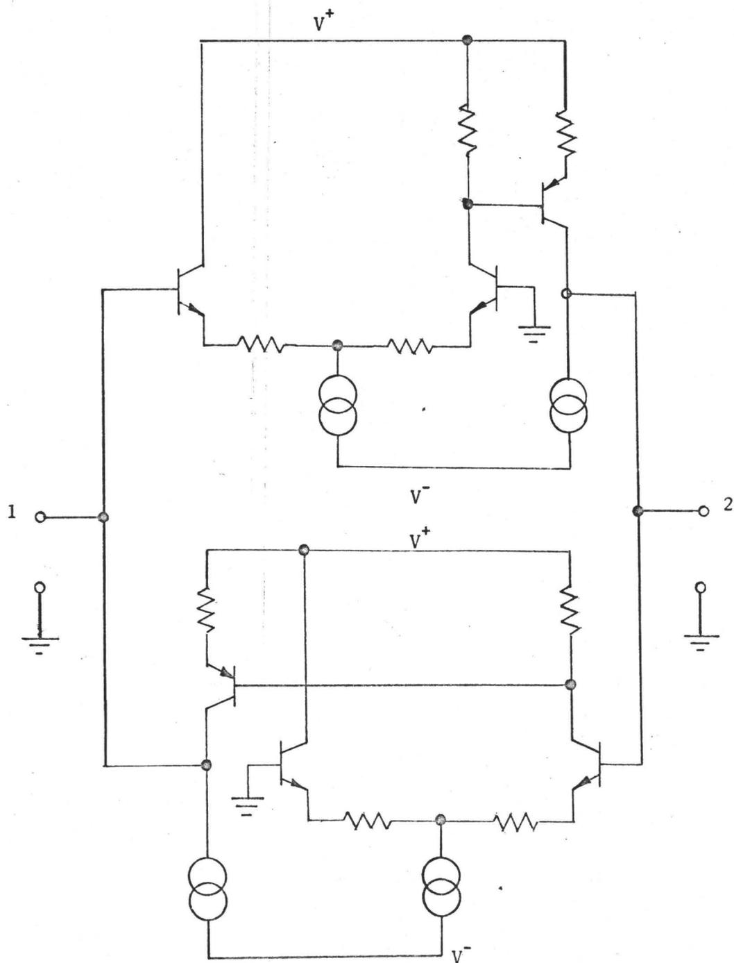
FIGURE 2-6: Grounded Gyrator Realization Using Differential Transistor Stages
