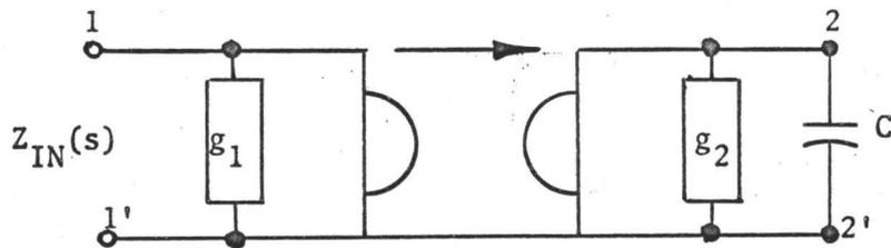
FIGURE 1-7: Simulated Inductor Using Non-Ideal Gyrator
