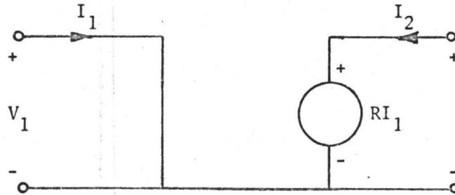
FIGURE 2-15: Current Controlled Voltage Source
