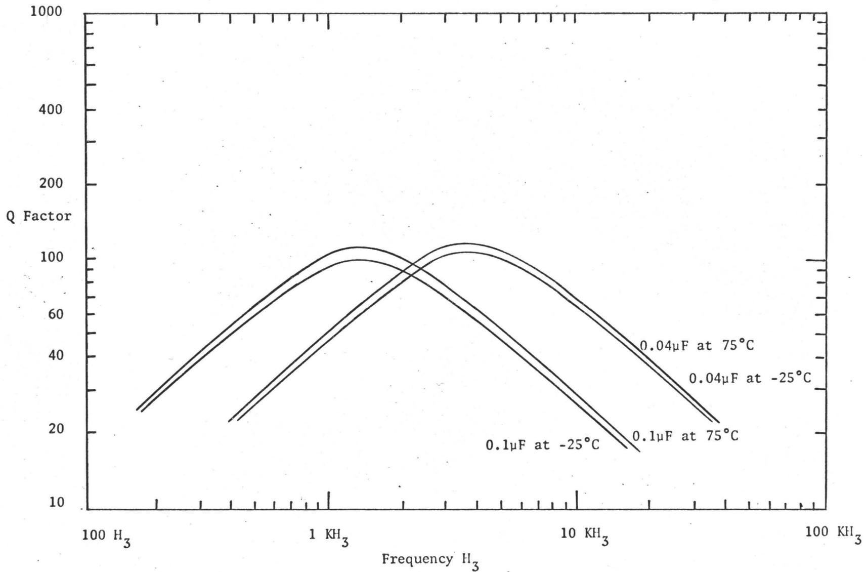
FIGURE 5-6: Q Factor Variation with Temperature at Low Frequencies
