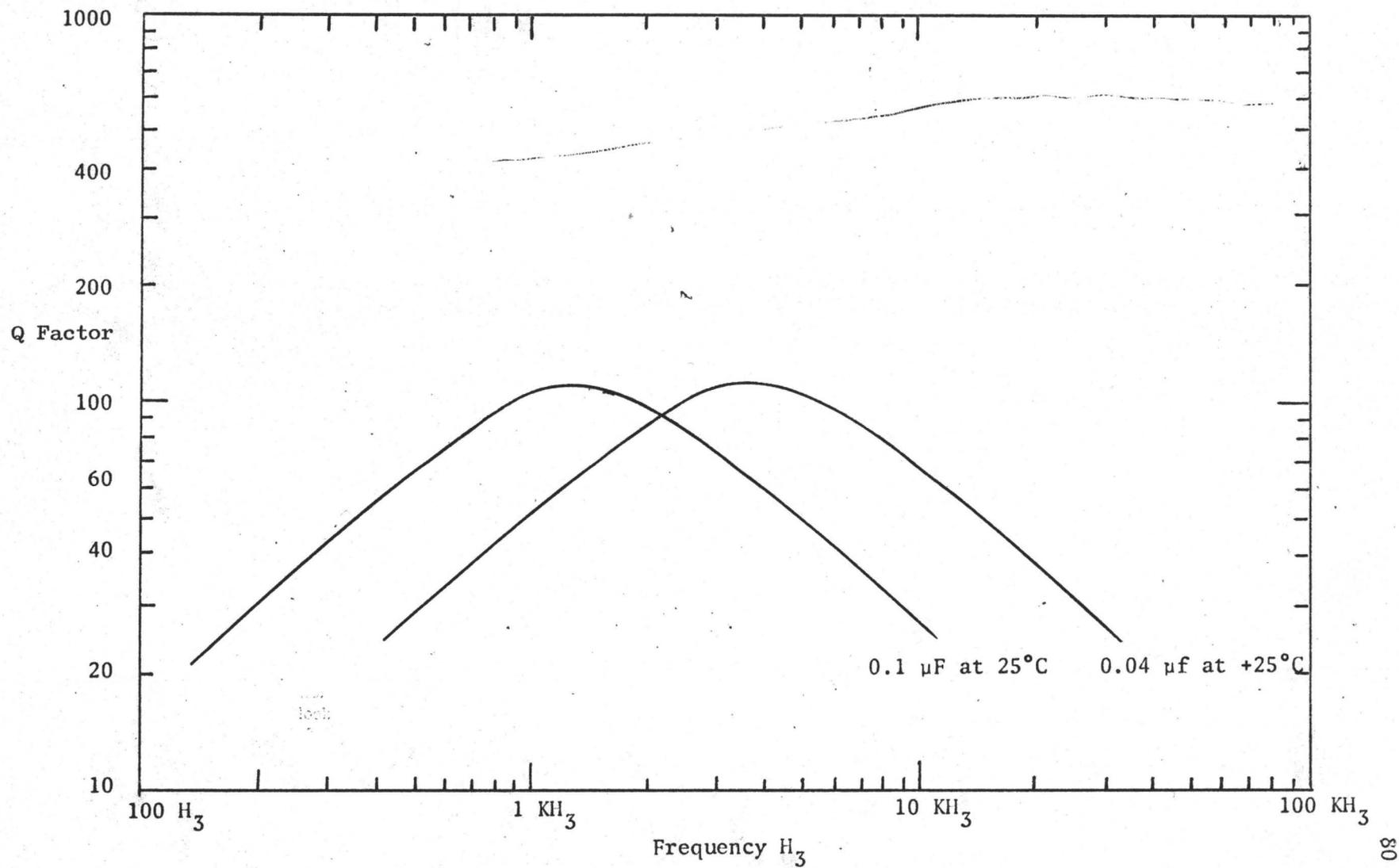
FIGURE 5-3: Q Factor at Room Temperature and Low Frequencies
