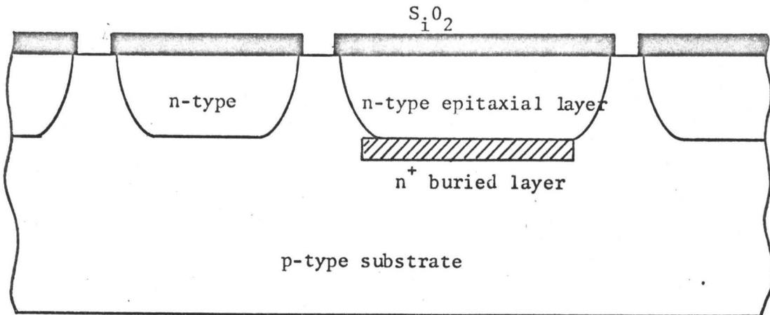
FIGURE 3-5: Cross Section of Isolation Diffusion
