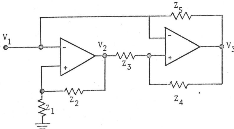
FIGURE 2-4: Grounded Gyrator Using Differential Amplifiers
