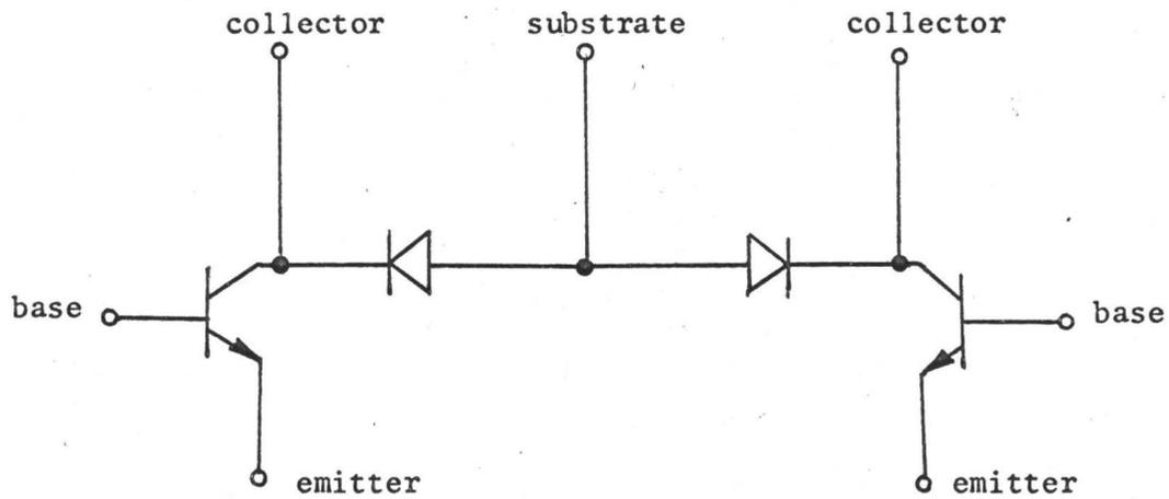
FIGURE 3-2: Equivalent Circuit of Two Isolated Transistors
