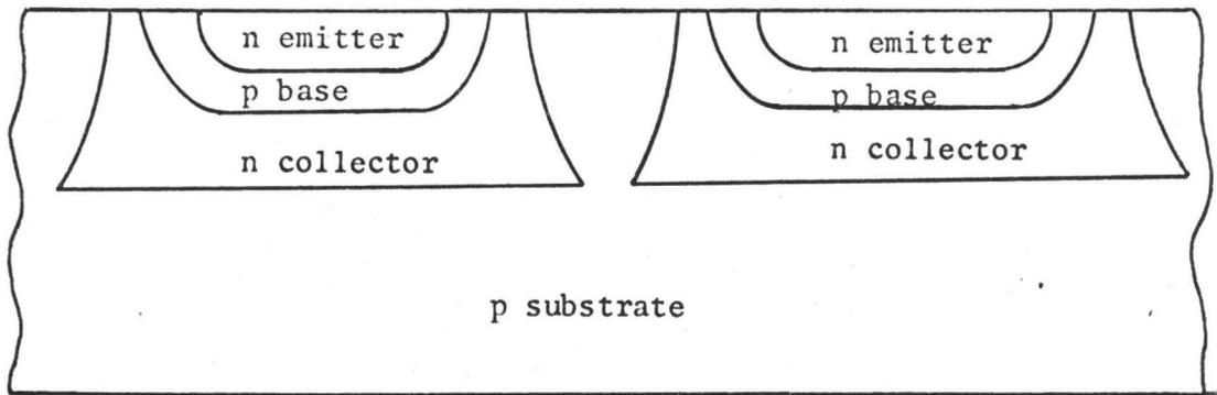
FIGURE 3-1: Cross Section of Monolithic npn Transistors
