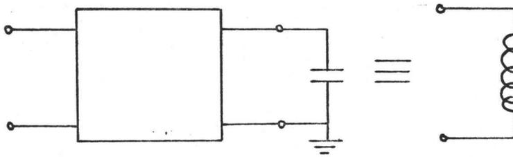
FIGURE 2-8: Simulated Floating Inductor
