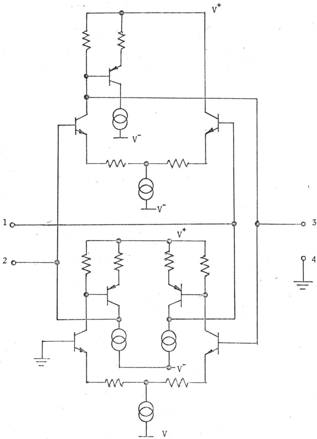
FIGURE 2-7: Semi-Floating Gyrator
