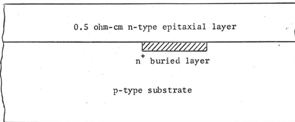
FIGURE 3-4: Cross Section of Epitaxial Layer
