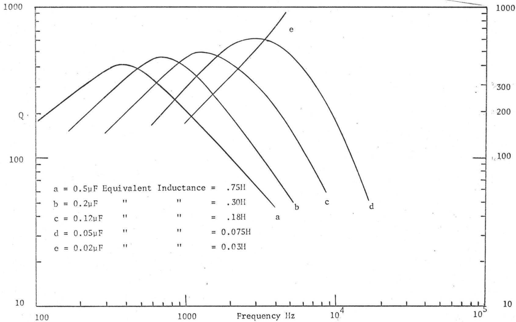
FIGURE 2(a): Measured Q Factor Against Frequency
