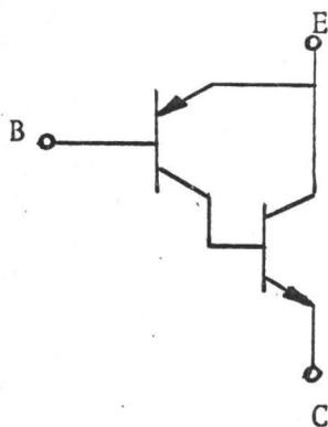
FIGURE 3-11(b): Equivalent Circuit of PNP Transistor
