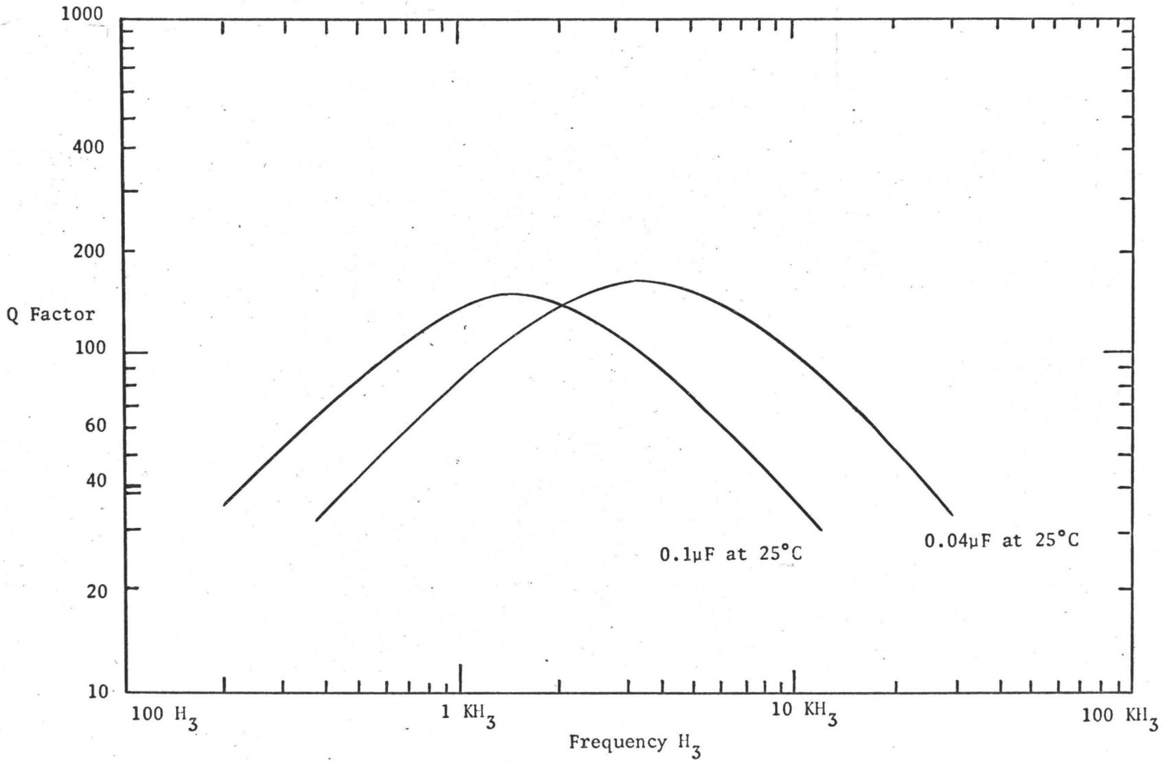
FIGURE 5-9: Q Factor of Gyrator Using Isolated Amplifiers
