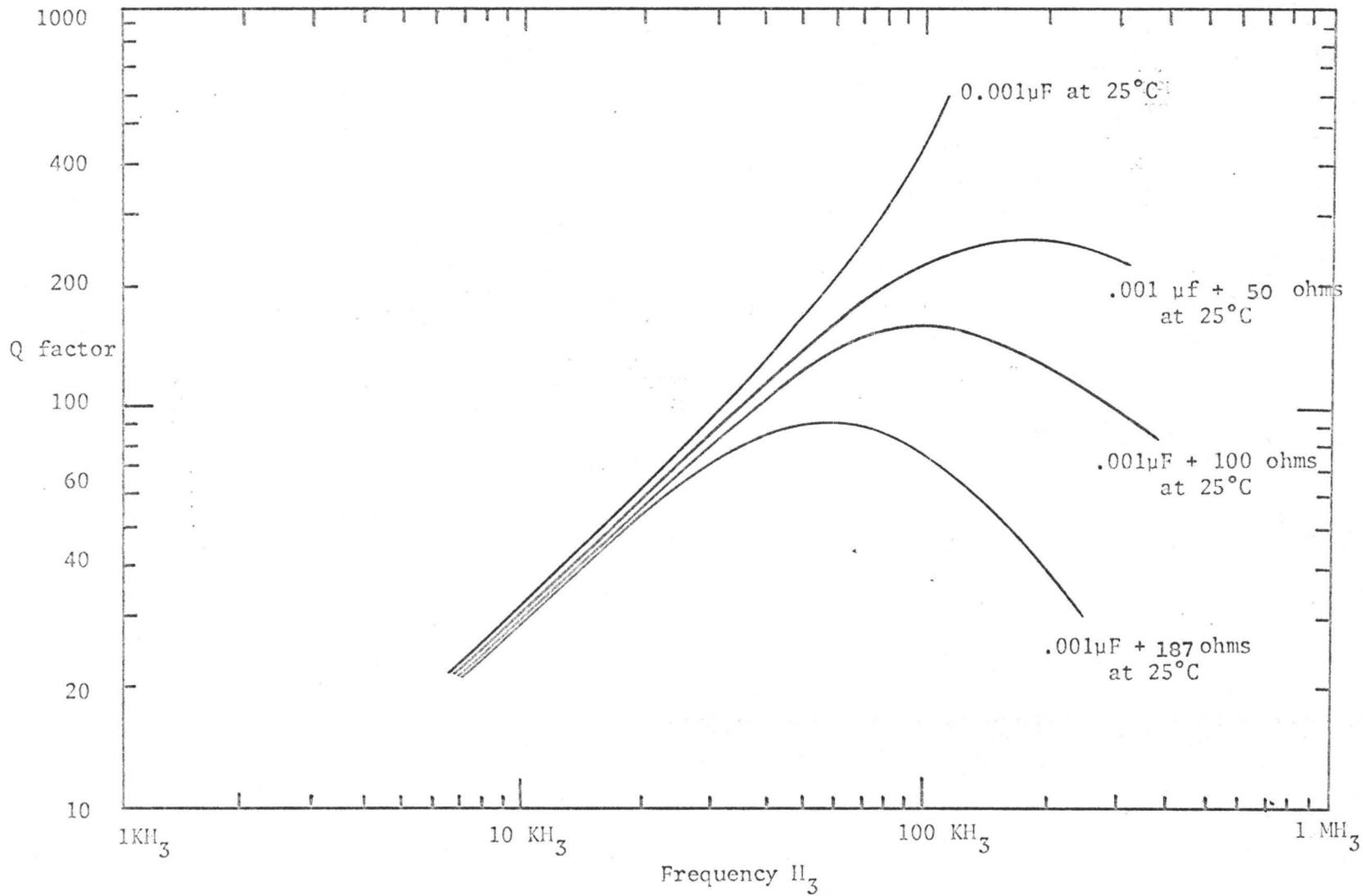
FIGURE 5-5: Q Factor of Compensated Gyrator at Room Temperature
