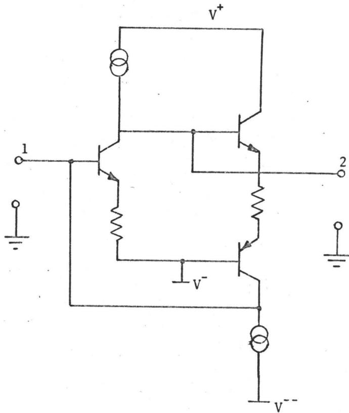
FIGURE 2-5: Grounded Gyrator Using Discrete Components
