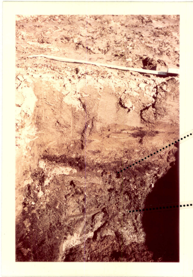
PLATE 5. Profile of the Silt Plain showing the buried peat layer and permafrost.
