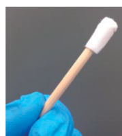
Fig. 4 Smell-Tell paper formatted as swab containing all of the components of the assay (pyridoxal, \text{Mg}^{2+} , and S -methyl-L-cysteine, PKase and Apo-TPase). The swab was contacted with a drop of ATP solution and was assessed by a human test panel after sitting on a dish for one hour, open to the atmosphere.
