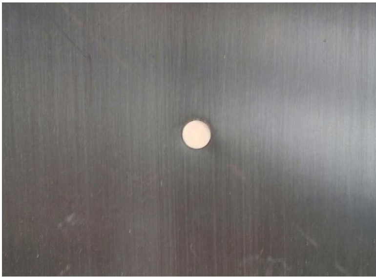
FIG. 6-2. Phantom layer with embedded dielectric cylinder.
