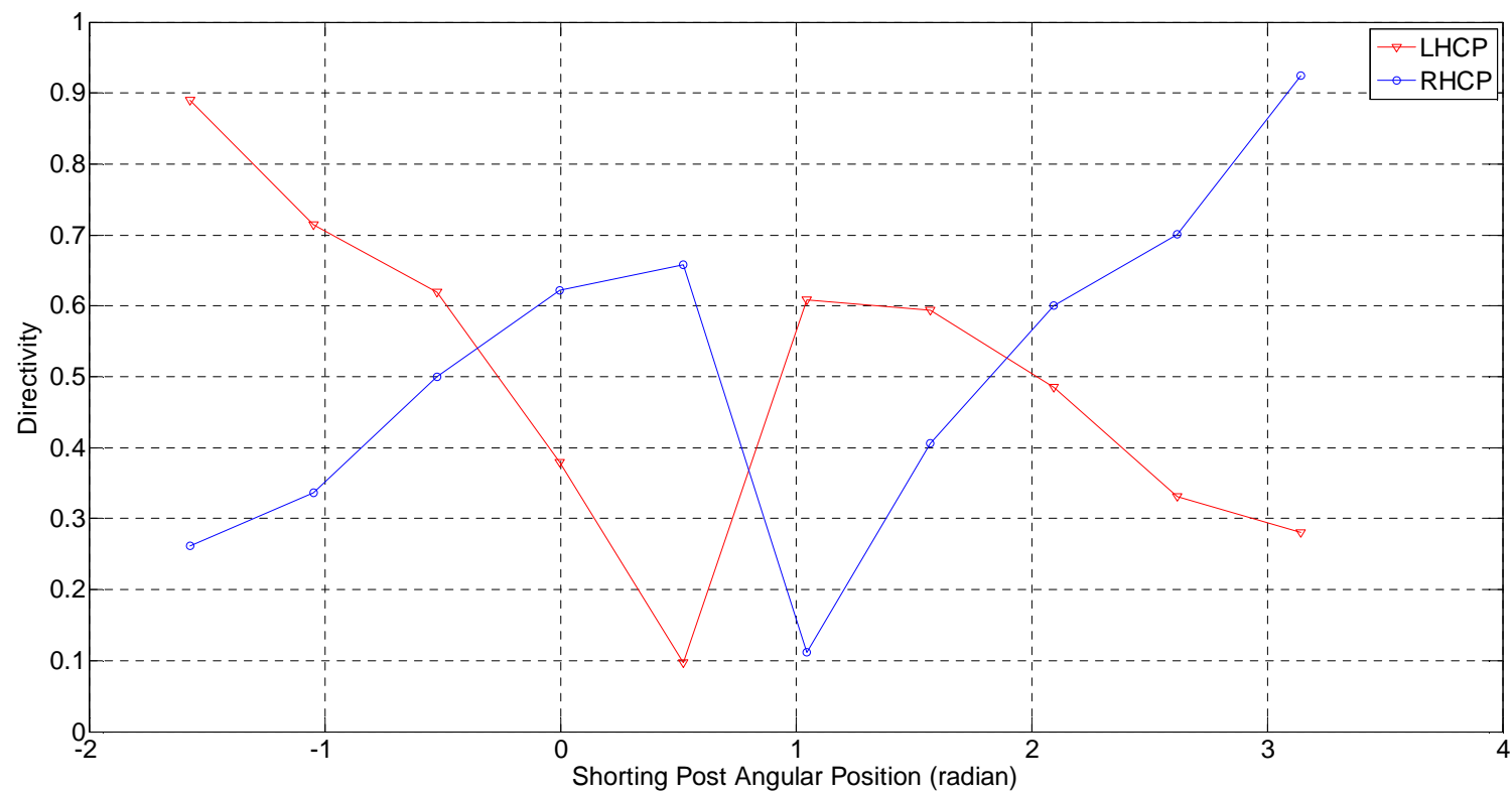
FIG. 4-12. Boresight directivity vs. shorting post angular position at 6.5 GHz.
