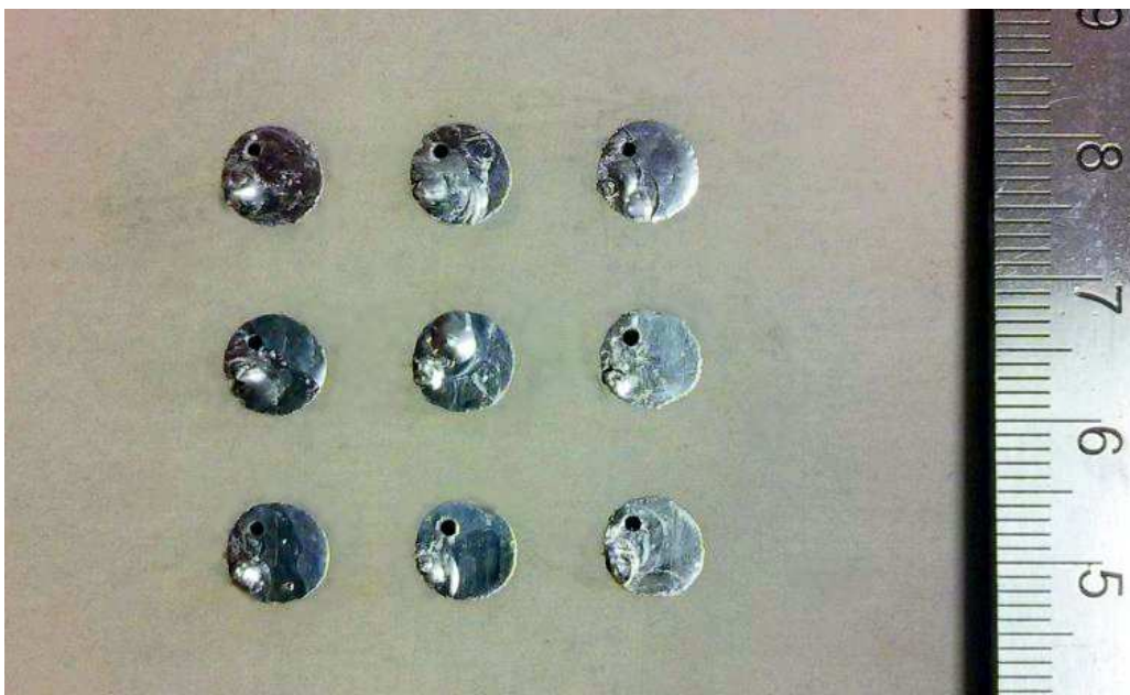
FIG. 4-23. Picture of fabricated 3x3 antenna array.
