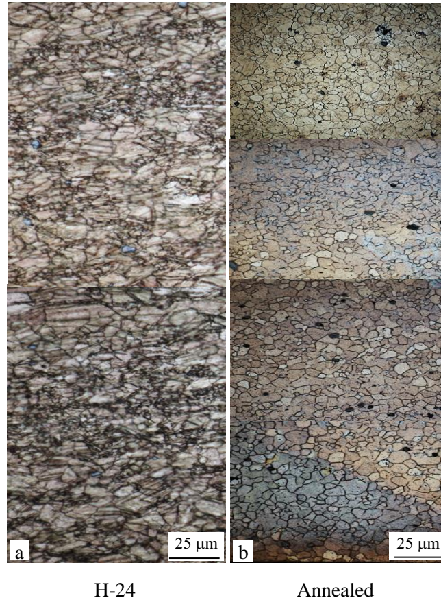
Fig. 6.2. Through thickness micrographs of AZ31 in (a) H-24 and (b) annealed conditions.
