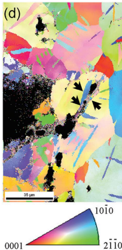
Figure 2.7: EBSD results near crack tip region after the fracture toughness test (Somekawa et al., 2009).
