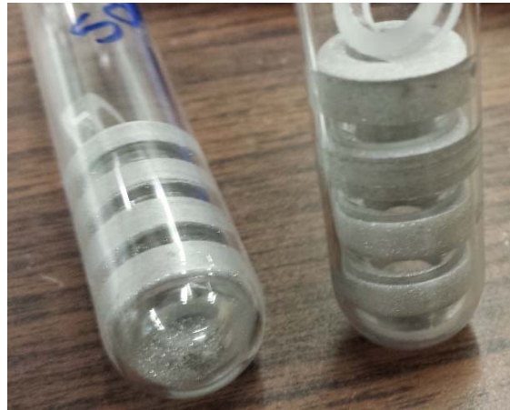
Figure 32- Samples sintered at 500°C – extensive growth
