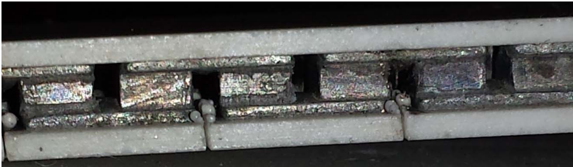
Figure 15 – Image of a commercial flat plate TEG module, irregular soldering and inconsistency are visible
