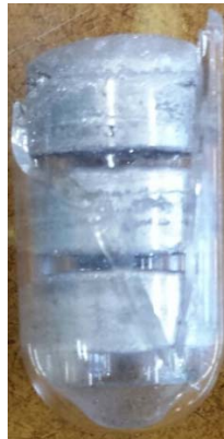
Figure 33 - Samples sintered at 550°C – extensive growth
