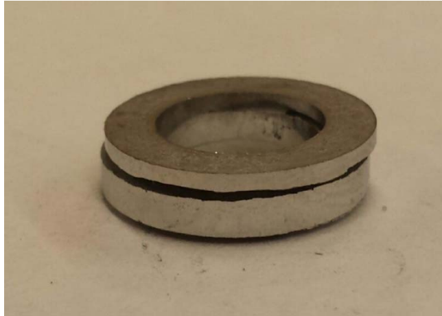
Figure 30 – Cracked sample during pressing process
