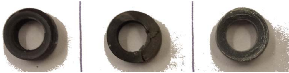
Figure 31 - Effect of location and orientation inside the furnace, left: deep inside the furnace, middle: in a horizontal orientation, right: outer half of the furnace – near door
