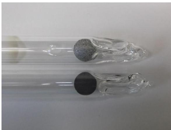
**Figure 2.1. A sample of PrSb before (top) and after (bottom) reaction at high temperature.**
