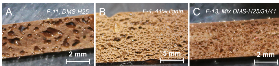
Figure 7.42 Cross-sectional images of lignin-silicone foams prepared from formulations with different molecular weight H-PDMS-H: (A) F-11, DMS-H25 (Mw = 6000 g/mol), (B) F-4, DMS-H31 (Mw = 28000 g/mol), and (C) F-13, Mixture of DMS-H25/31/41 (containing 26% H25, 48% H31, and 26% H41, H-41: Mw = 62700 g/mol).
