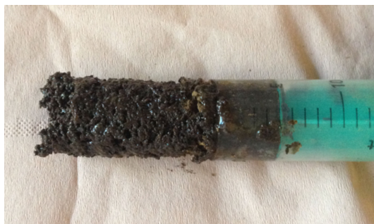
Figure 7.43 Attempts to make lignin-silicone foams using DMS-H41 (F-12) failed due to the high intrinsic viscosity of DMS-H41. The precursor is semi-cured, and could not be processed in extruder.
