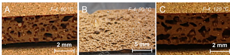
Figure 7.44 Cross-sectional images of lignin-silicone foams (formulation F-4) molded under different temperatures: (A) 60, (B) 90, and (C) 120°C.
