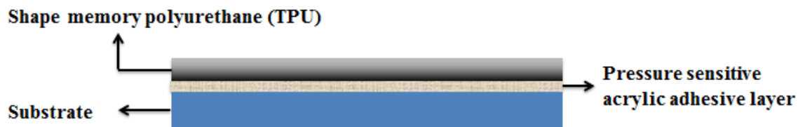
Figure 1-2 Multilayer structure of TPU based laminate
