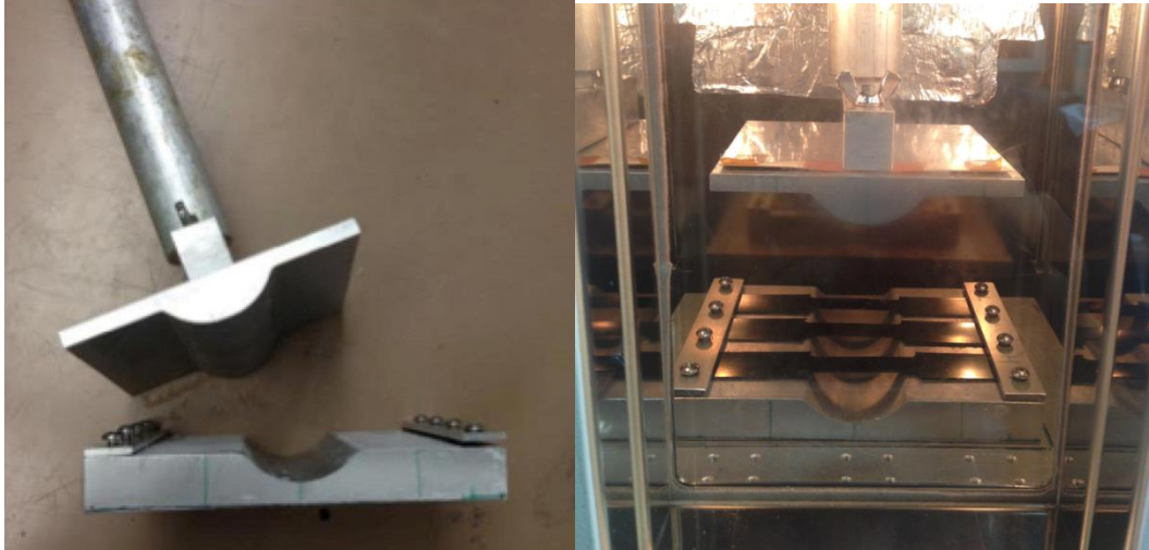
Figure 3-1 Matched molds used in the forming process (left) and thermoforming process inside the environmental chamber (right)
