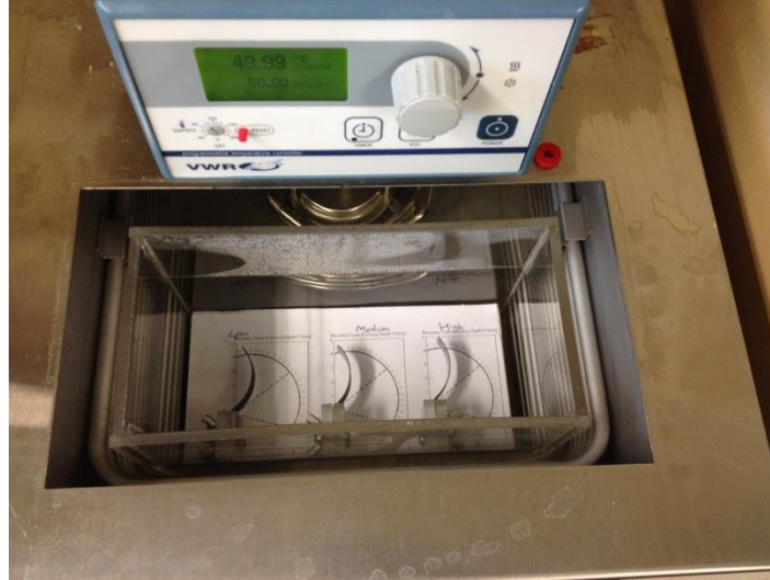
Figure 3-2 Temperature regulated recovery chamber using a digitally controlled circulating water bath
