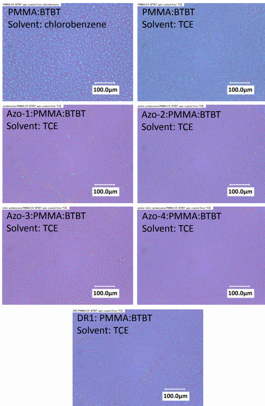
Figure S5.1: Optical Microscope images of films spin coated from 1,1,2,2-tetrachlorethane (TCE) onto an HMDS modified Si/SiO 2 wafer, as well as a control film spin coated from chlorobenzene. All films show similar morphology when spin coated from the same solvent.
