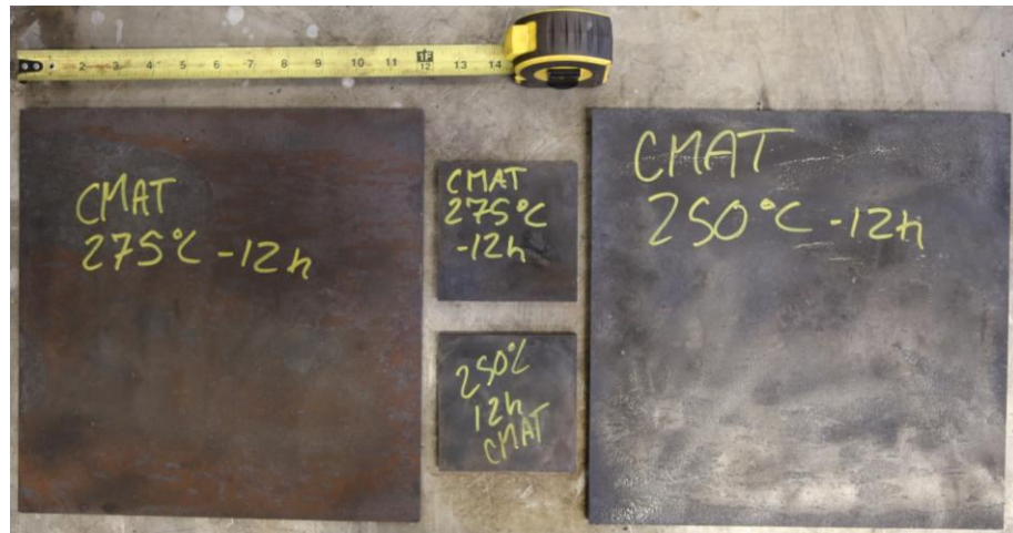
Figure 12-CMAT alloy plates produced with respective heat treatments written on them
