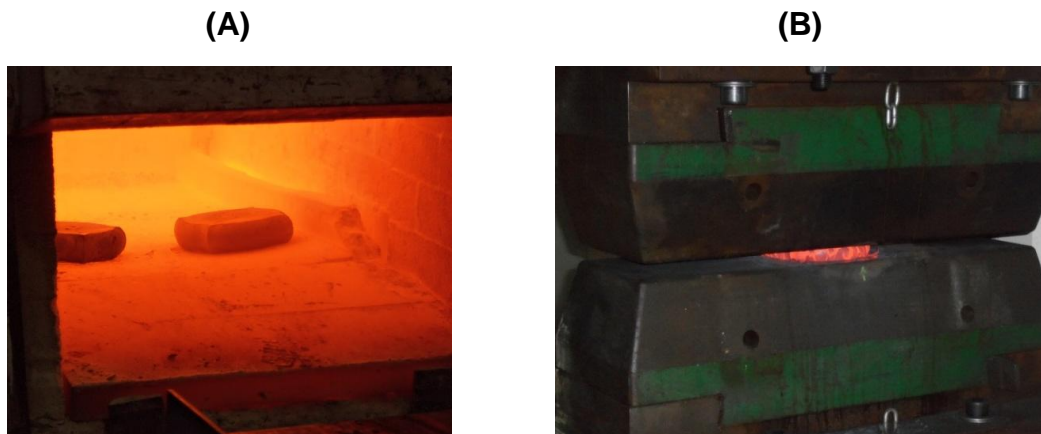
Figure 10-A: forged CMAT alloy disks being reheated to 1150°C between passes. B: hot disk being forged
