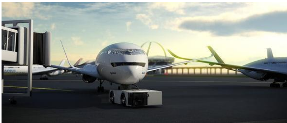
Figure 1-4 – Airbus Taxiing Vehicle [18]
