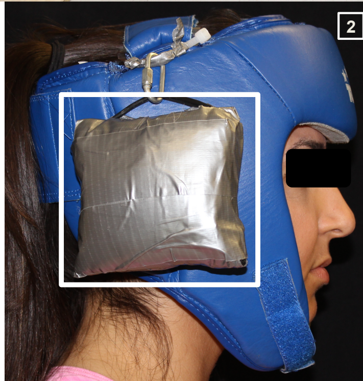
Figure 3.1: 1. Tilt board tilted at 52^\circ . Foot rest near the bottom of the board was adjusted to the participant's height. The height of the top of the board as well as the bottom of the board was adjusted to facilitate different angle requirements. 2. Load attached to the side of the helmet.
