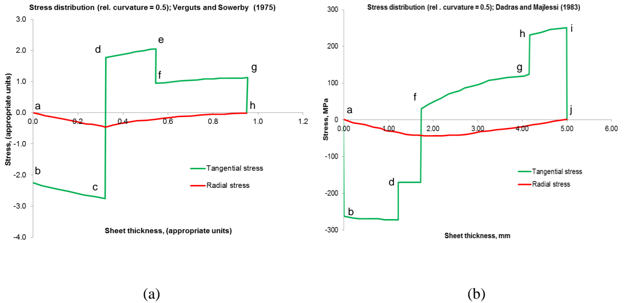
Figure 14. Stress distribution plots, (a) Bi-layer laminate by Verguts and Sowerby (1975), (b) Tri-layer laminate by Dadras and Majlessi (1983).
