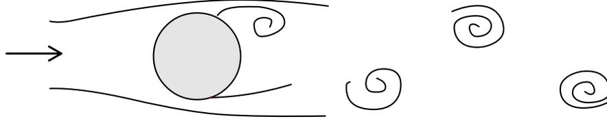
Figure 2.1: Kármán vortex street, showing flow past a cylinder generating an array of vortices.
