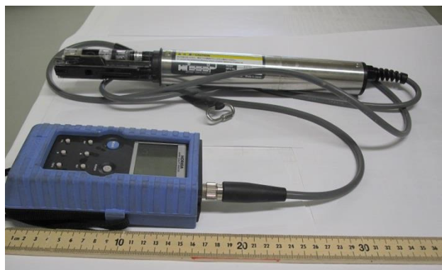
Figure 4.4 Photograph of the calibrator optical DO sensor (Horiba Sensor for Water Quality Monitor U-2000). The dimension of the detector exceeded 35 cm as shown in the picture.
