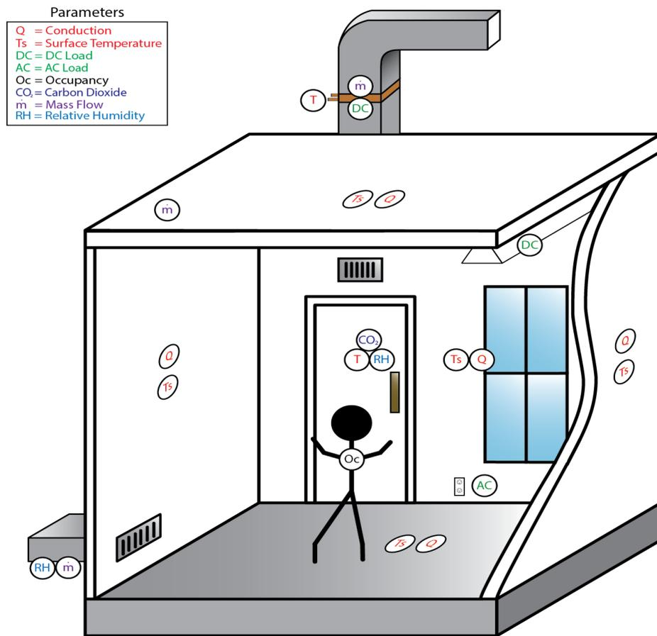
Figure 10: Locations of Sensors to Measure Energy Transfer in an Internal Zone with VAV and Reheat Coil
