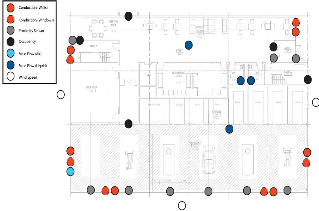
Figure 32: Proposed Location of Sensors for First Floor in Hatch Centre
