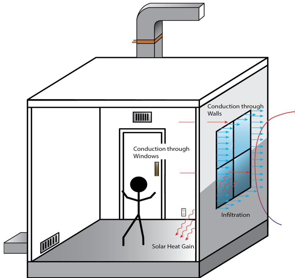
**Figure 9: Diagram of Energy Flows in an External Zone for a Commercial Building with VAV and Reheat Coil**
