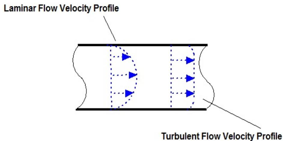
**Figure 2: 2-Dimensional Velocity Profile of Air in a Duct**
