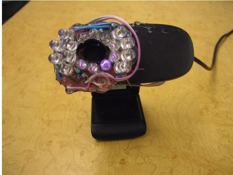
**Figure 33: Webcam with IR Filter and IR light Source**
