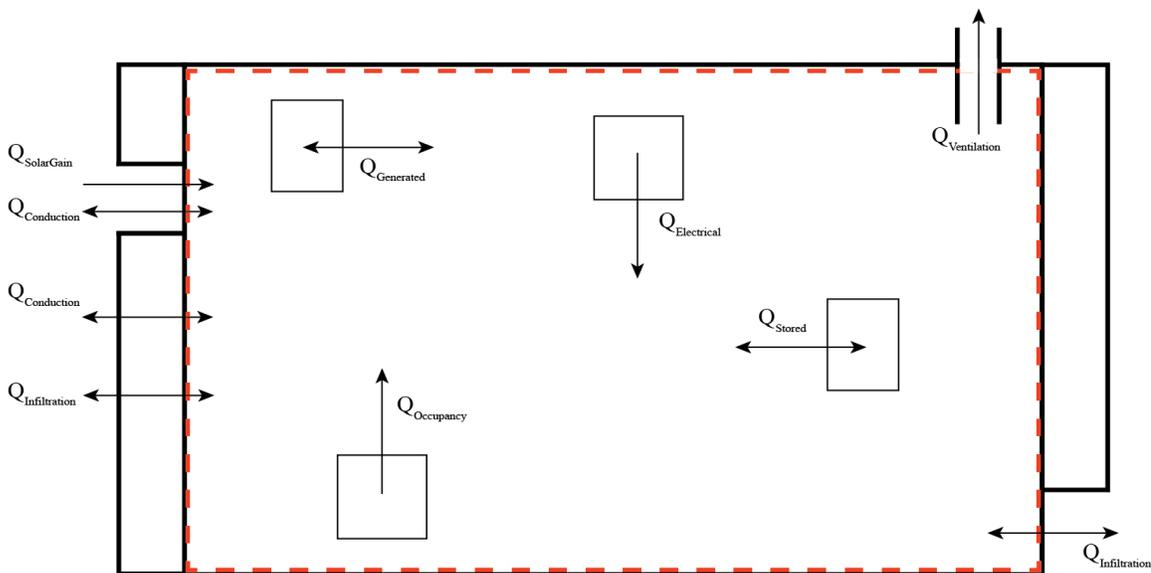
Figure 1: Schematic of the Control Volume for the Energy Transfer in a Commercial Building
