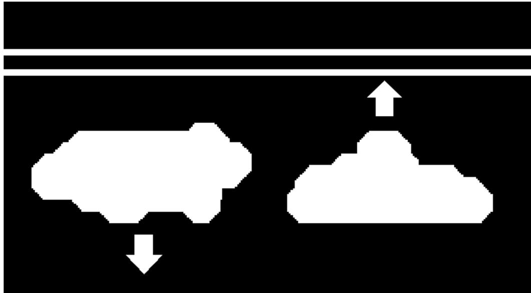
Figure 4: Representation of Signal Sent to Image Processing Software from Optical Turnstile Sensors with Arrows to Denote Movement
