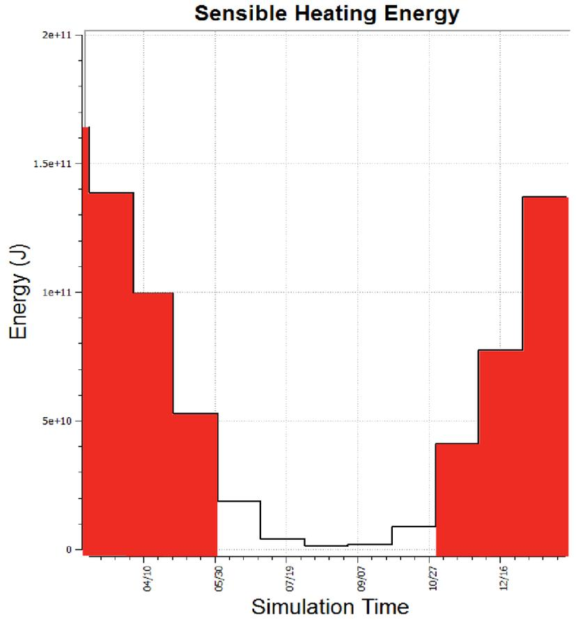
Figure 28: Monthly Sensible Heating Energy for the Building Energy Model
