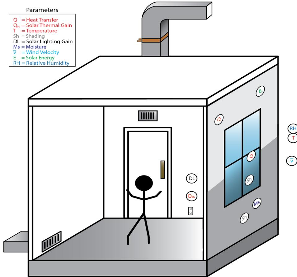
Figure 11: Locations of Sensors to Measure Energy Transfer in an External Zone with VAV and Reheat Coil
