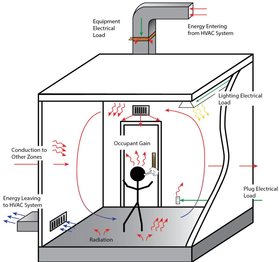
Figure 8: Diagram of Energy Flows in an Internal Zone for a Commercial Building with VAV and Reheat Coil
