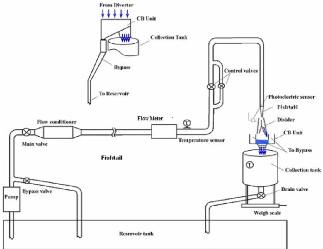
Figure 34: Schematic of the system used for the static gravimetric method
