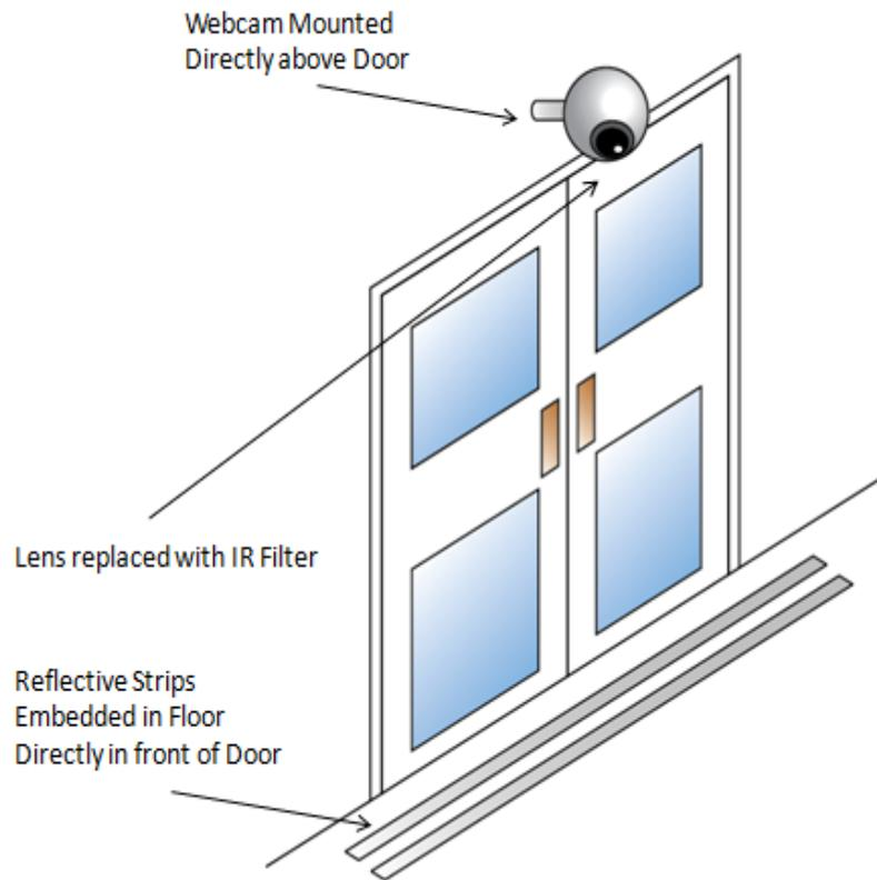
Figure 18: Diagram for Installation of the Occupancy Tracking System
