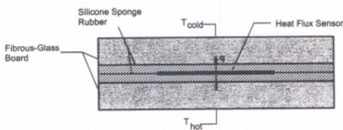
**Figure 36: Test assembly for heat flux sensor calibration**
