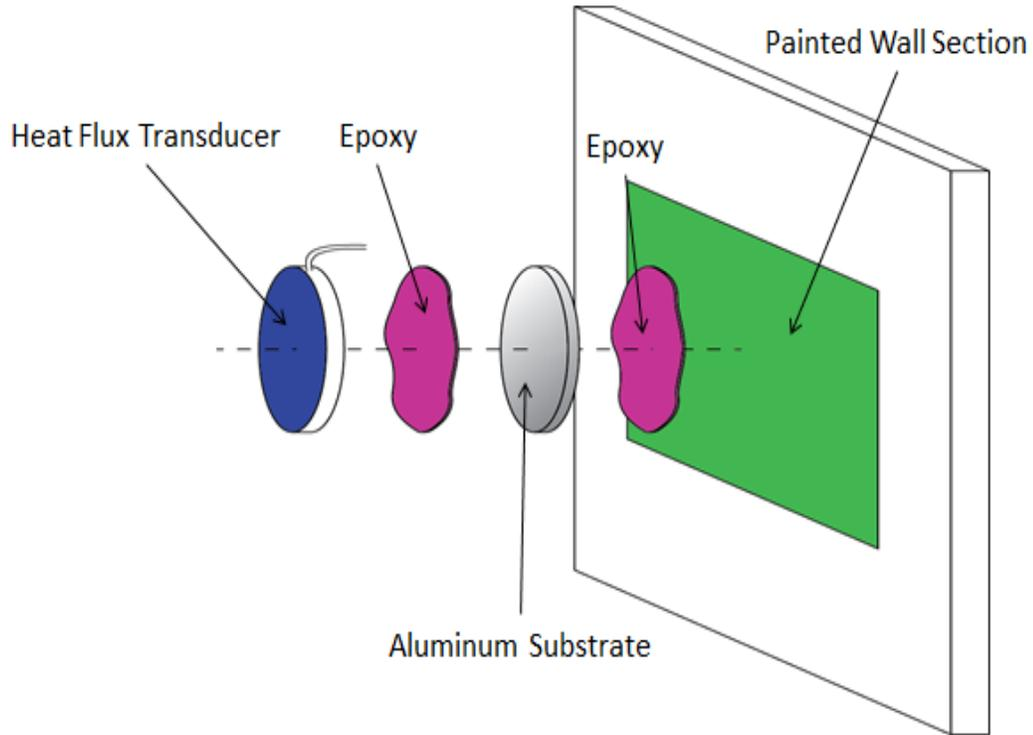
Figure 14: Recommended Heat Flux Transducer Installation on a Wall
