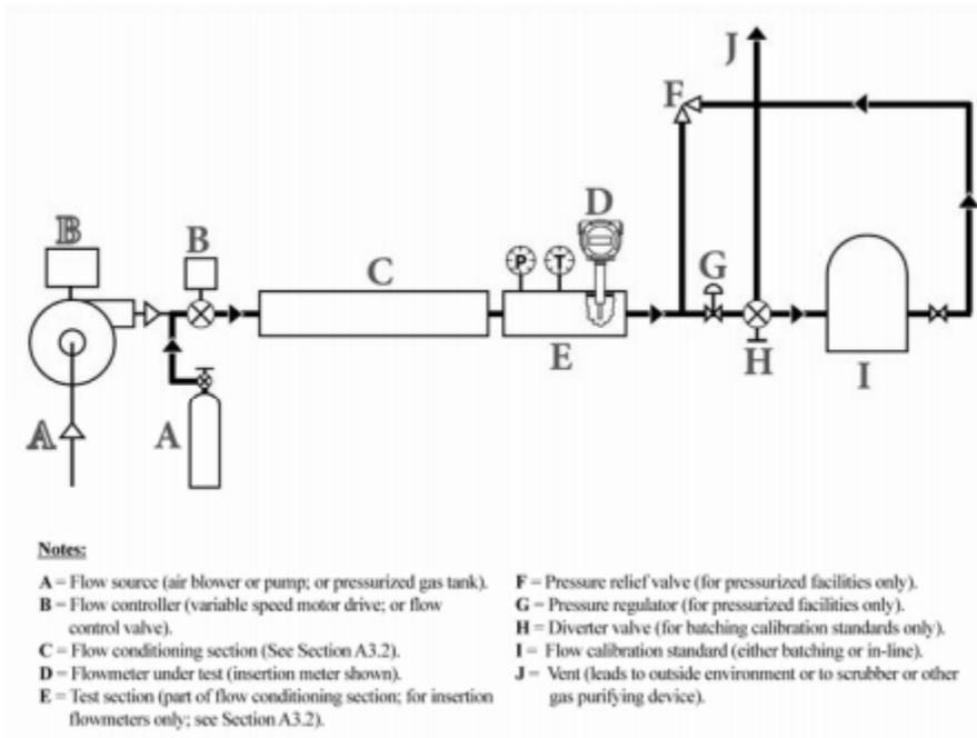
Figure 35: Schematic of System Required for an Open-Loop Tester for Airflow
