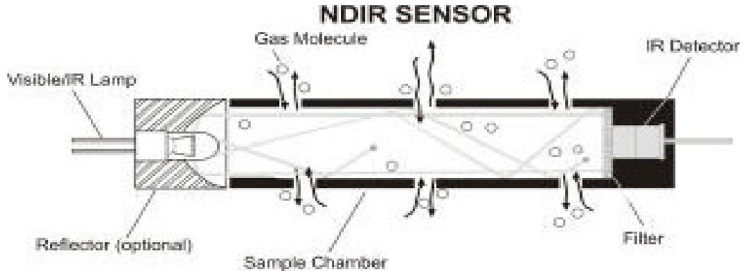
Figure 3: Schematic of an NDIR CO<sub>2</sub> Sensor
