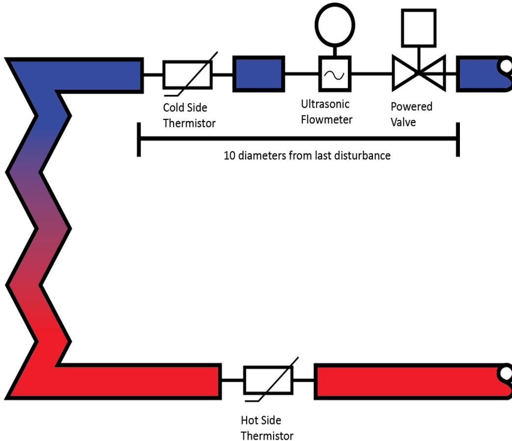
Figure 13: Schematic Diagram for Installation Liquid Flow Sensors around Heat Transfer Locations
