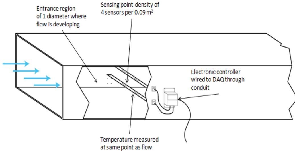
Figure 12: Installation for the Mass Air Flow in a Building
