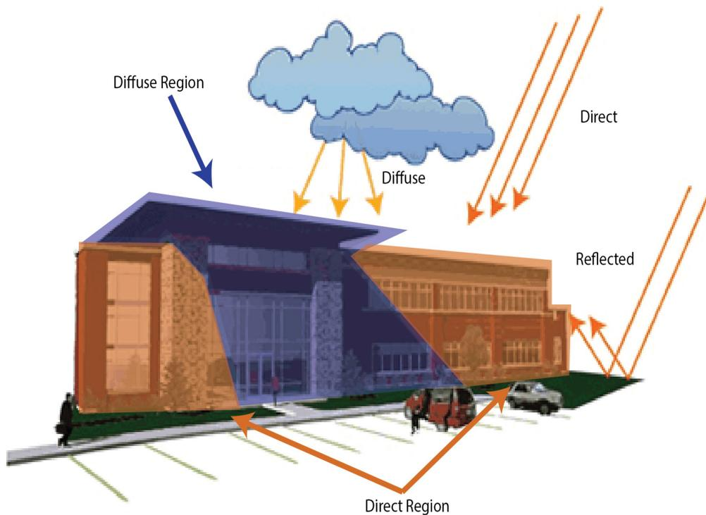
Figure 16: Areas of Direct and Indirect Sunlight on a Building
