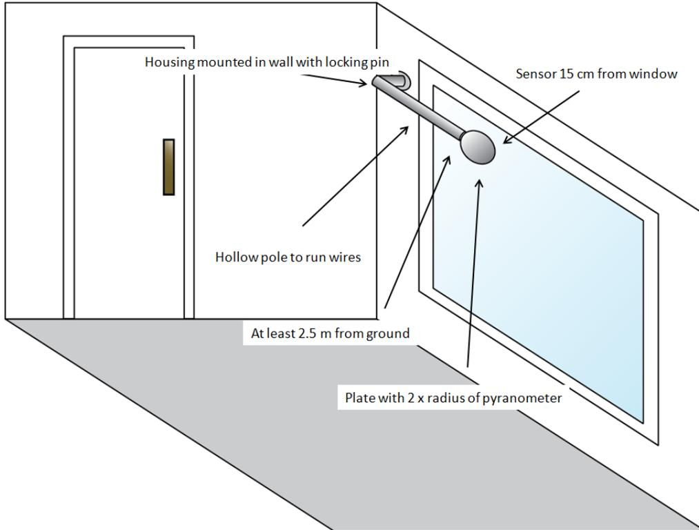
**Figure 15: Installation Summary of Pyranometer for Heat Gain Measurement System**
