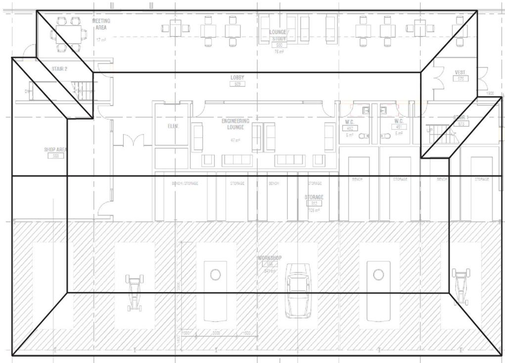
**Figure 6: Layout of the First Floor of the Hatch Centre with an Overlay of the Zone Layout**
