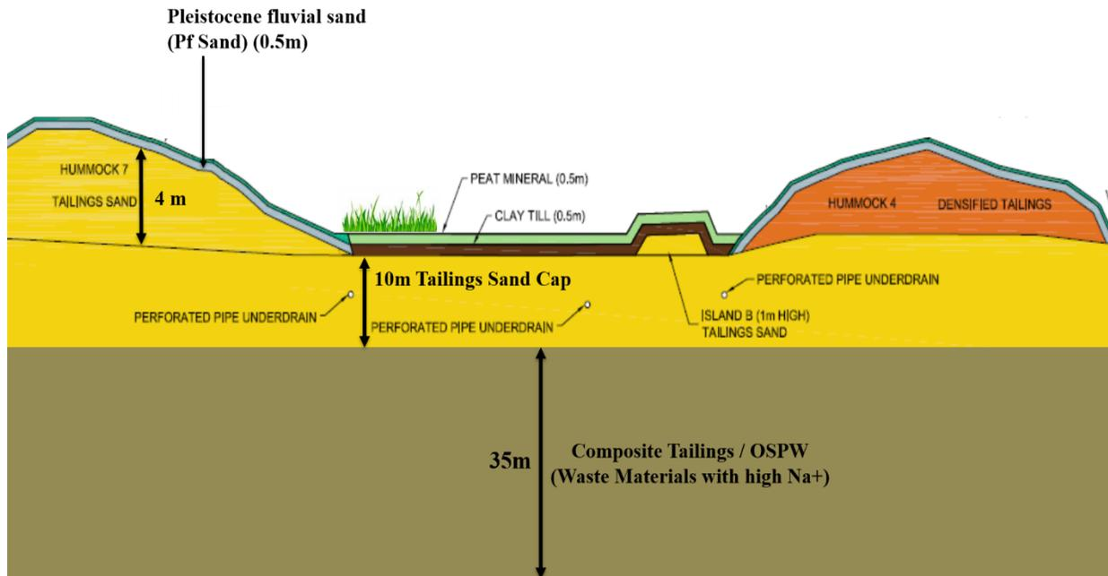
*Figure 3.1.* Cross section of the SFW looking east to illustrate construction materials. It should be noted that this diagram is not to scale.
