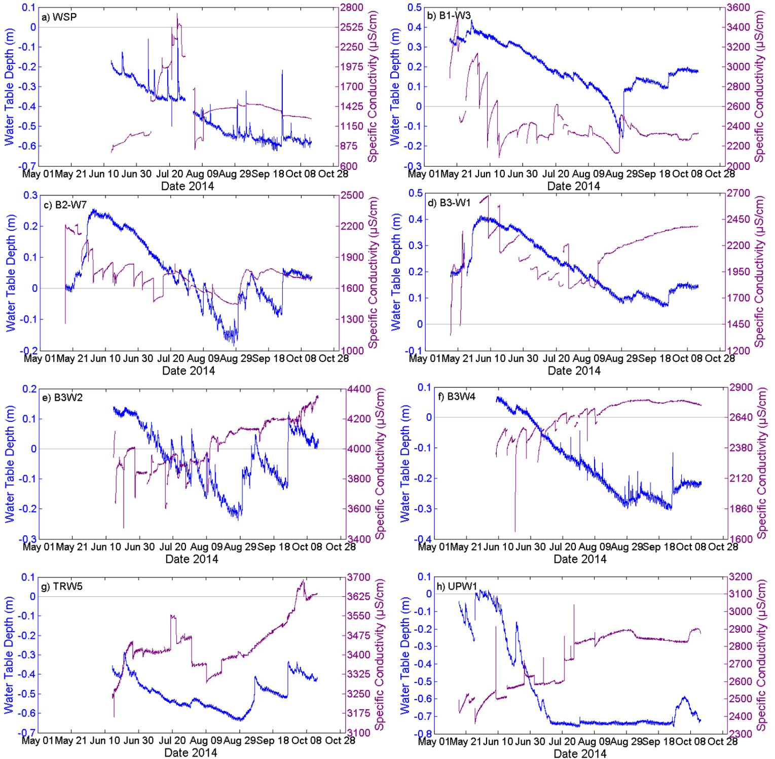
Figure 4.3. Water table depth and specific conductivity during May – October 2014. The grey horizontal line indicates the ground surface.
