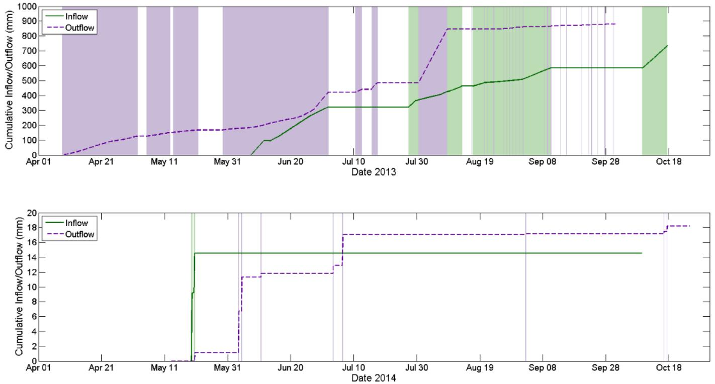
Figure 4.1. Cumulative inflow and outflow within the SFW for 2013 (top) and 2014 (bottom). Green and purple areas indicate the duration the inflow and outflow pumps were on, respectively as recorded by the Flow Transmitter.
