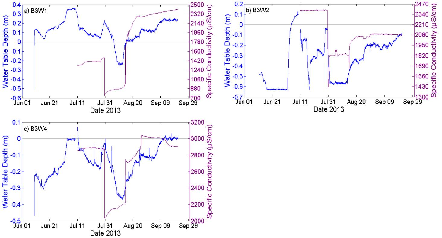
Figure 4.2. Water table depth and specific conductivity during May – September 2013. Grey horizontal line indicated the ground surface.
