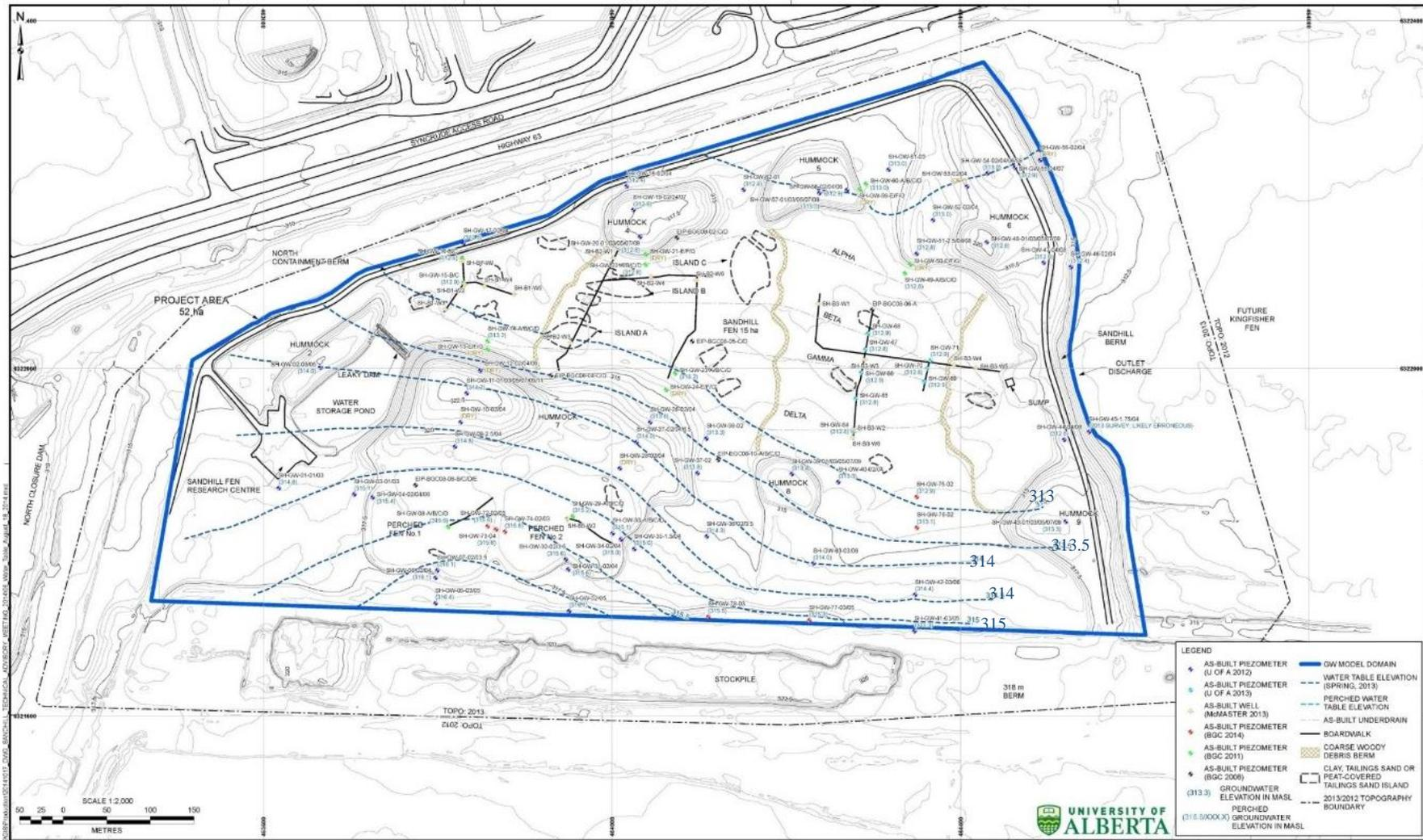
Figure 4.7. 2014 groundwater elevation in the SFW (BCG, 2015).
