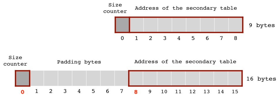
Figure 4.11: One entry of the main table. The top figure shows the two data members without considering padding bytes. In the bottom figure, 7 padding bytes are inserted after the size counter to make the address start at position 8.
