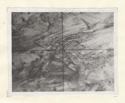
Staurolite Porphyroblast in Sillimanite - L49
