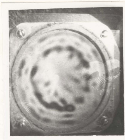
Fig. 19: The vibrational mode pattern of a piezoelectric speaker cone driven at a frequency of 6.6 kHz
