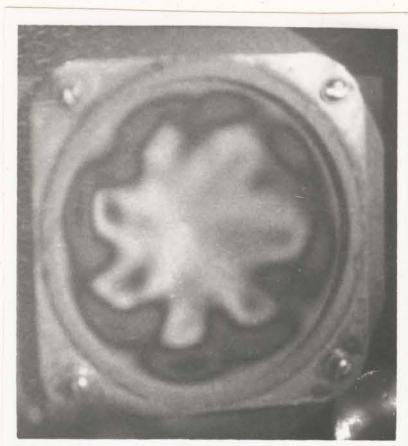
Fig. 15: The vibrational mode pattern of a piezoelectric speaker cone driven at a frequency of 3.0 kHz
