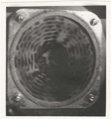
Fig. 23: The vibrational mode pattern of a piezoelectric speaker cone driven at a frequency of 15.5 kHz
