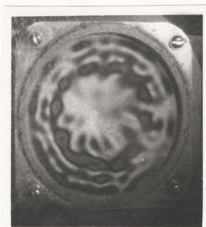
Fig. 18: The vibrational mode pattern of a piezoelectric speaker cone driven at a frequency of 5.5 kHz
