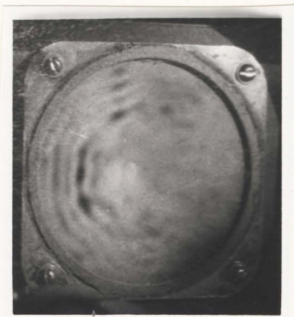
Fig. 20: The vibrational mode pattern of a piezoelectric speaker cone driven at a frequency of 8.2 kHz
