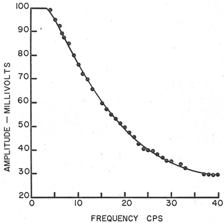
FIG. 8.1 FREQUENCY RESPONSE OF DIRECT WRITING DYNOGRAPH GALVANOMETER.
