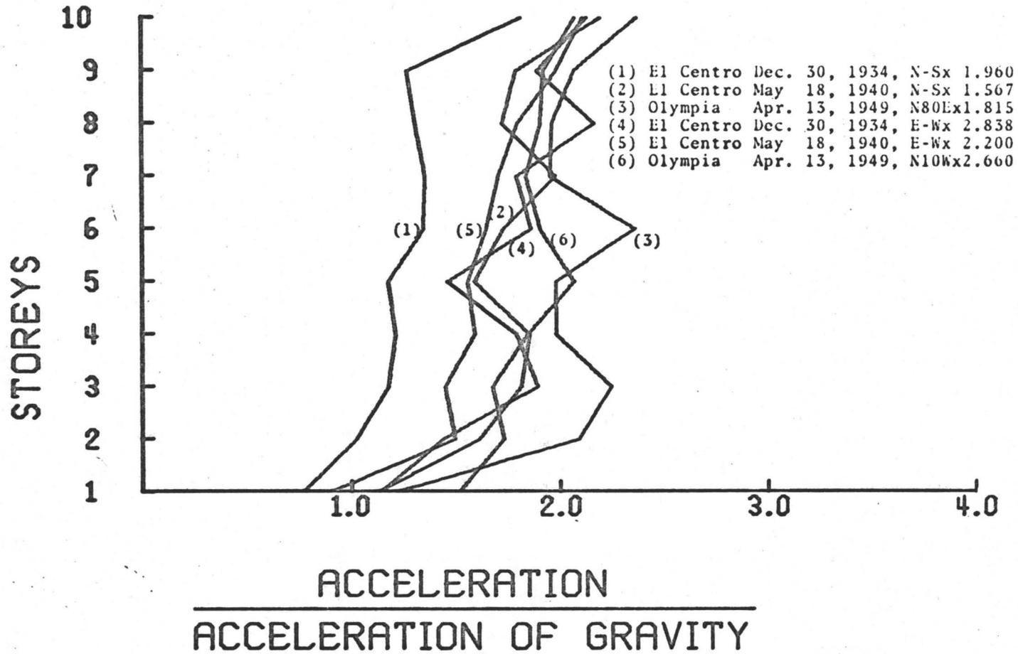
FIG. 4.54 EFFECT OF DIFFERENT EARTHQUAKE CHARACTERISTICS
