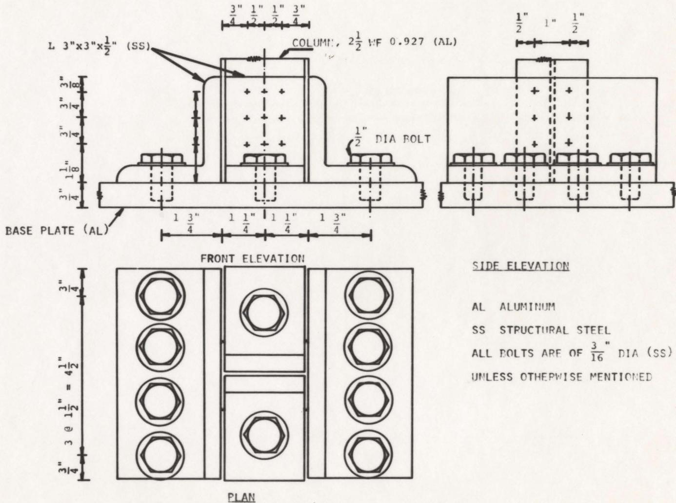
FIG. 6.5 DETAILS OF COLUMN BASE JOINT
