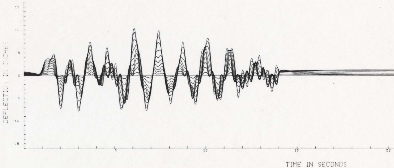
FIG. 4.11 INELASTIC RESPONSE HISTORY FOR  $\gamma = 1.0$ ,  $\alpha = 0.8$
