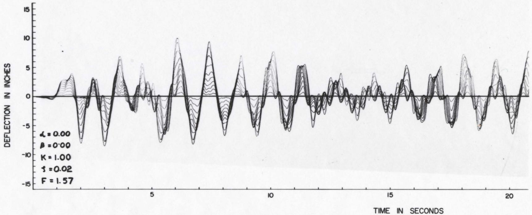
FIG. 4.1 INELASTIC RESPONSE HISTORY OF BASIC STRUCTURE,
