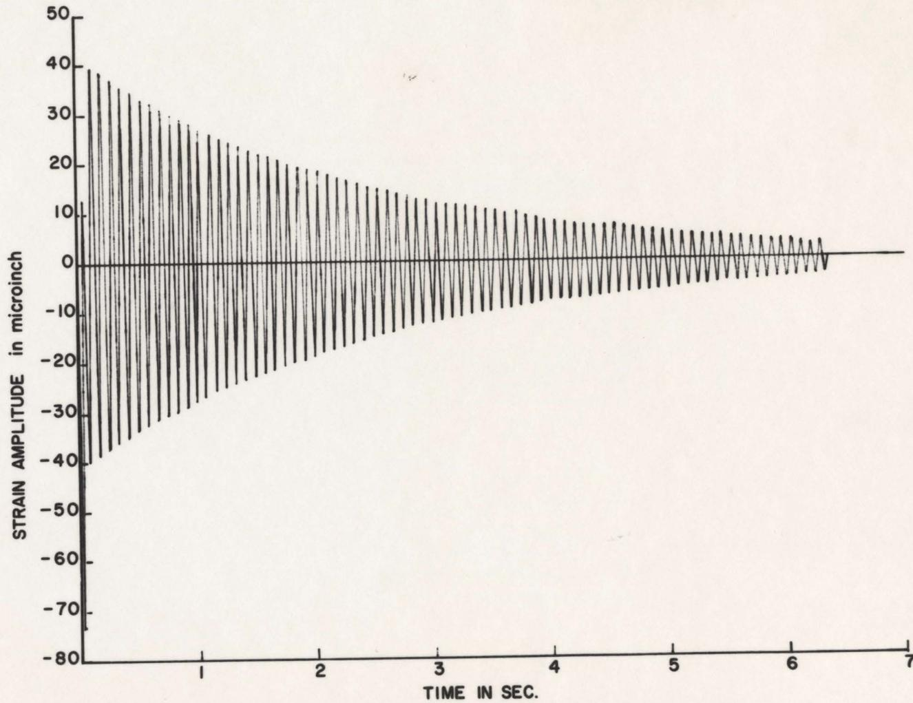
FIG. 8.2 TYPICAL STRAIN GAUGE RESPONSE TO IMPULSE
