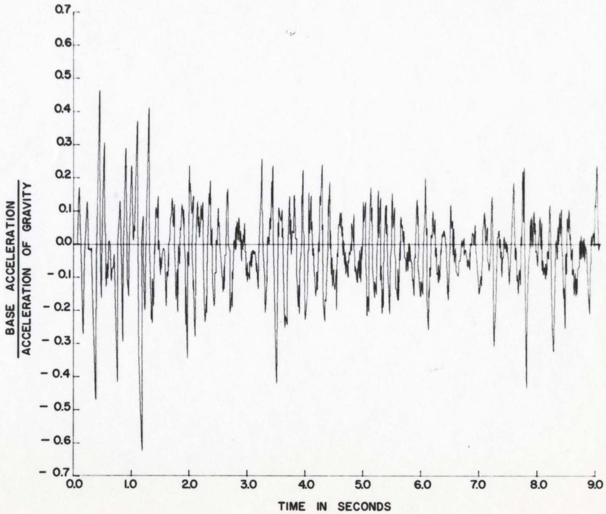
FIG. 8.4 RECORD OF BASE ACCELERATION
