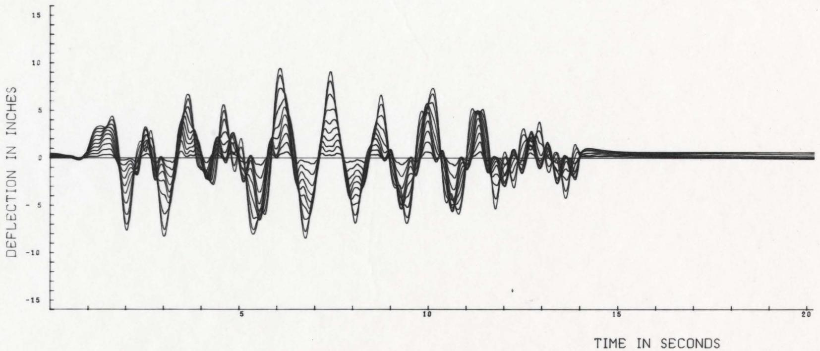
FIG. 4.10 INELASTIC RESPONSE HISTORY FOR  $\gamma = 0.5$ ,  $\alpha = 0.8$
