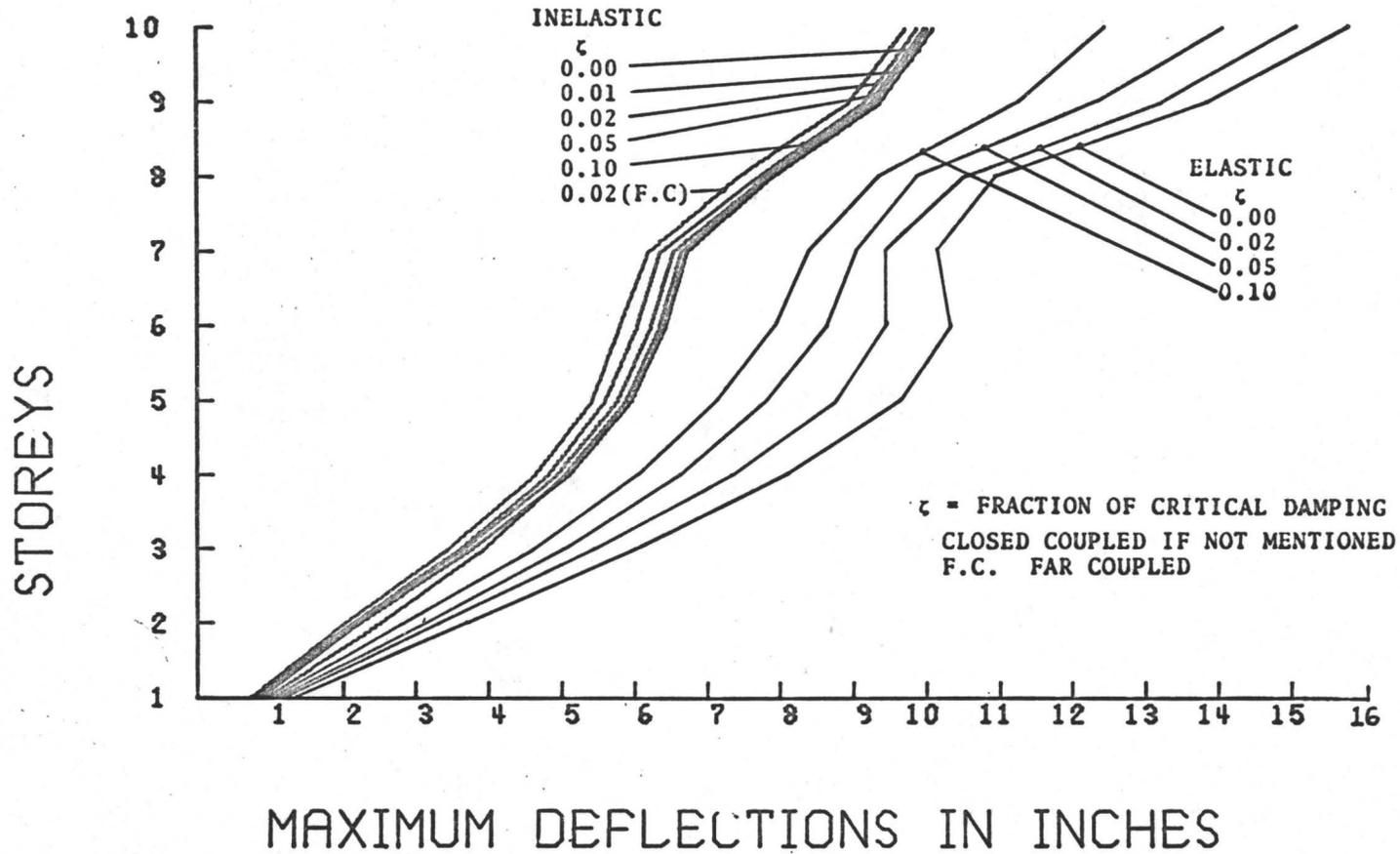
FIG. 4.38 EFFECT OF DAMPING
