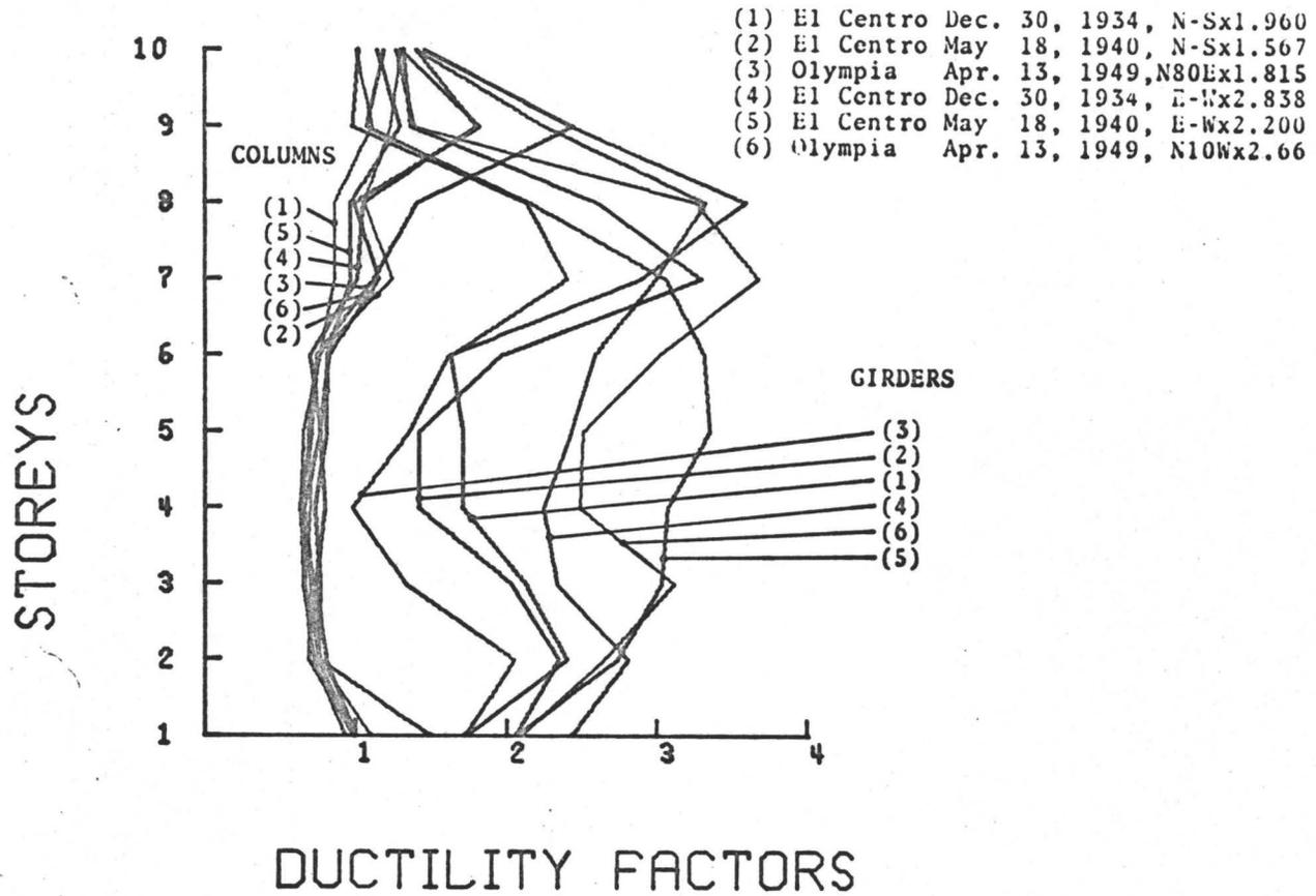
FIG. 4.53 EFFECT OF DIFFERENT EARTHQUAKE CHARACTERISTICS
