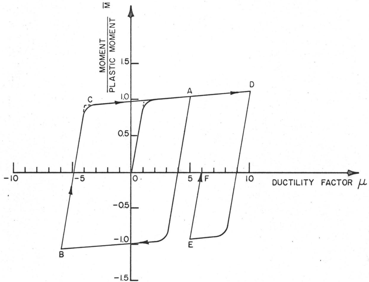
FIG. 6.8 MOMENT CURVATURE RELATIONSHIP OF COLUMNS FROM GIRDER COLUMN JOINT TEST
