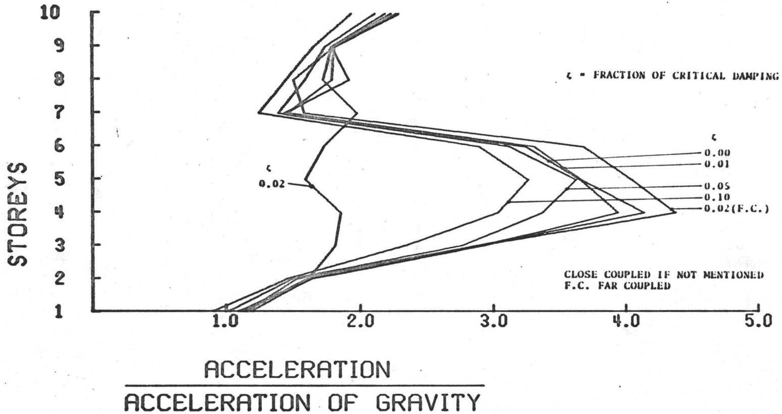
FIG. 4.37 EFFECT OF DAMPING
