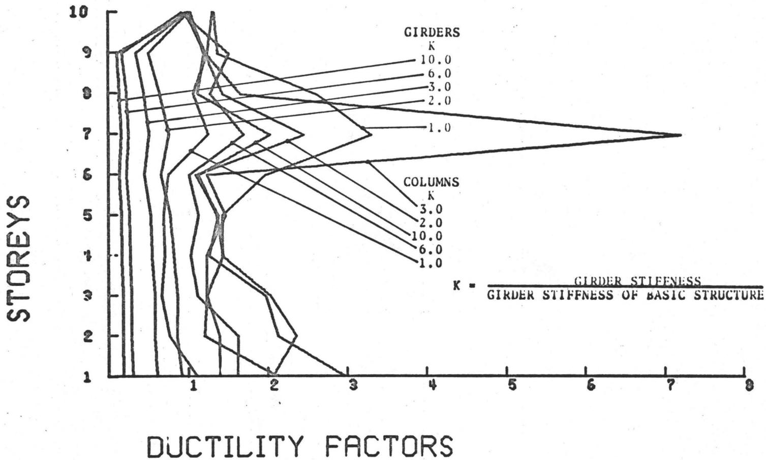
FIG. 4.28 EFFECT OF VARIATION OF RELATIVE STIFFNESS BETWEEN GIRDERS AND COLUMNS
