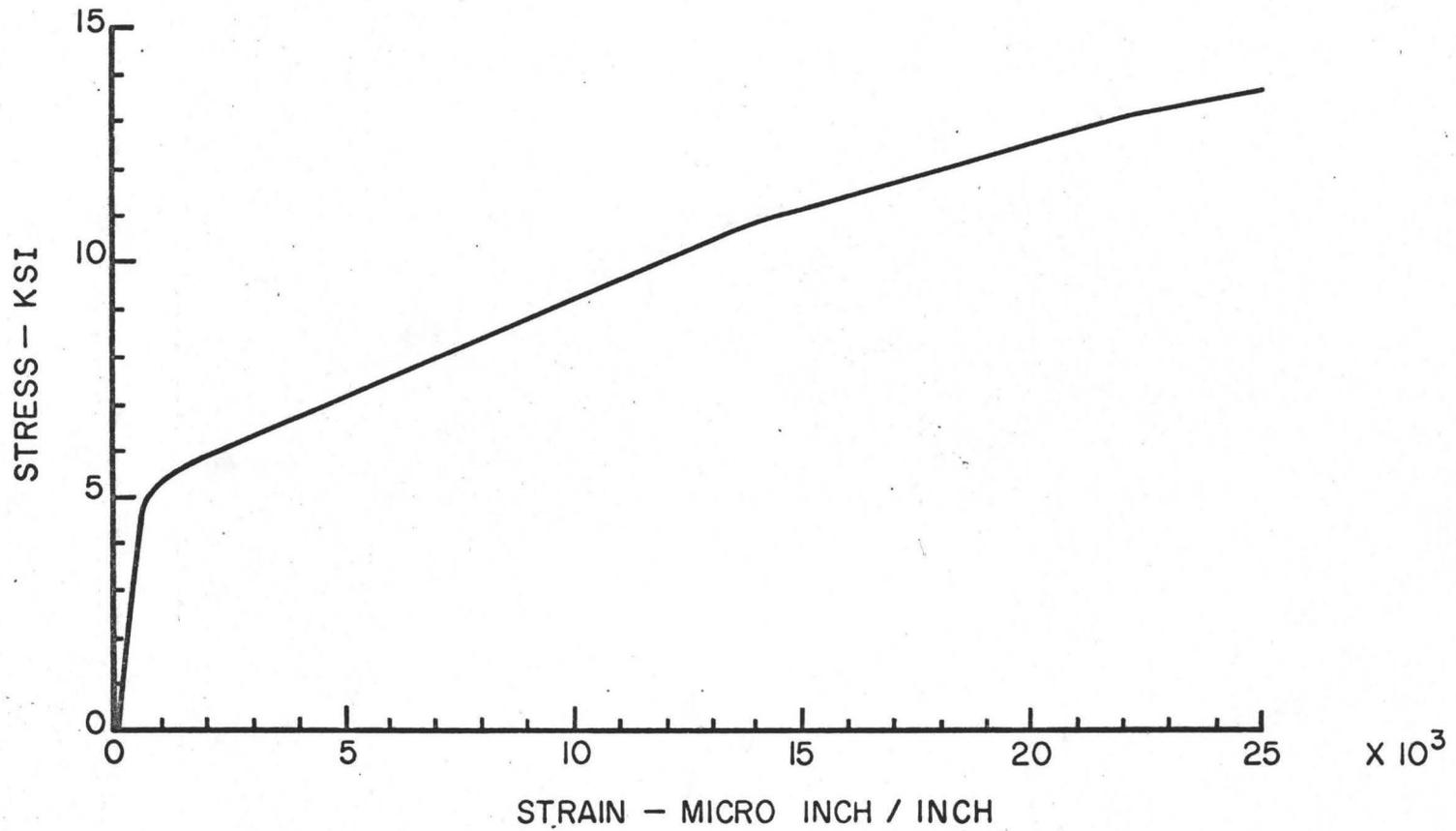
FIG. 6.6 ALUMINUM STRESS - STRAIN CURVE
