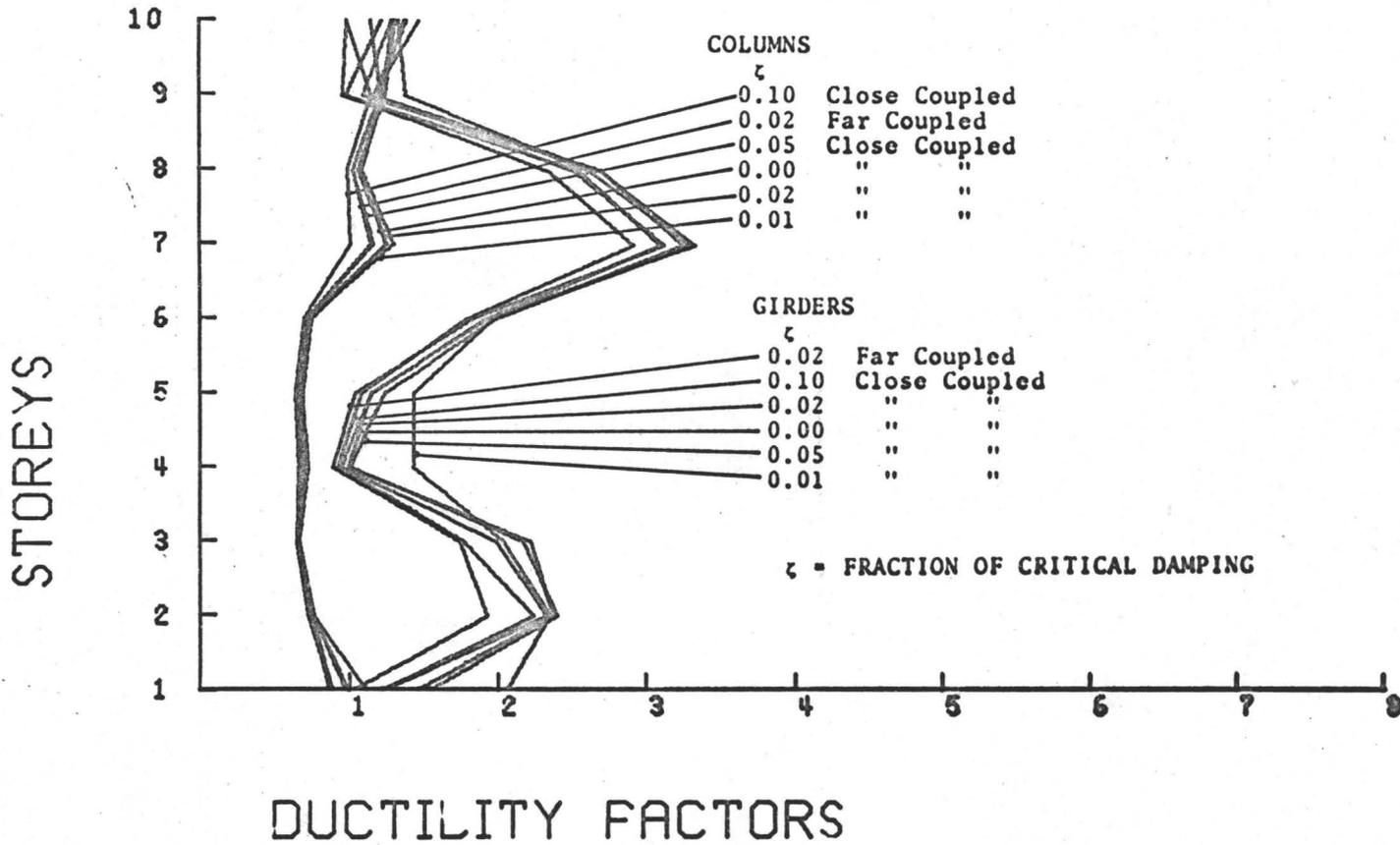
FIG. 4.36 EFFECT OF DAMPING
