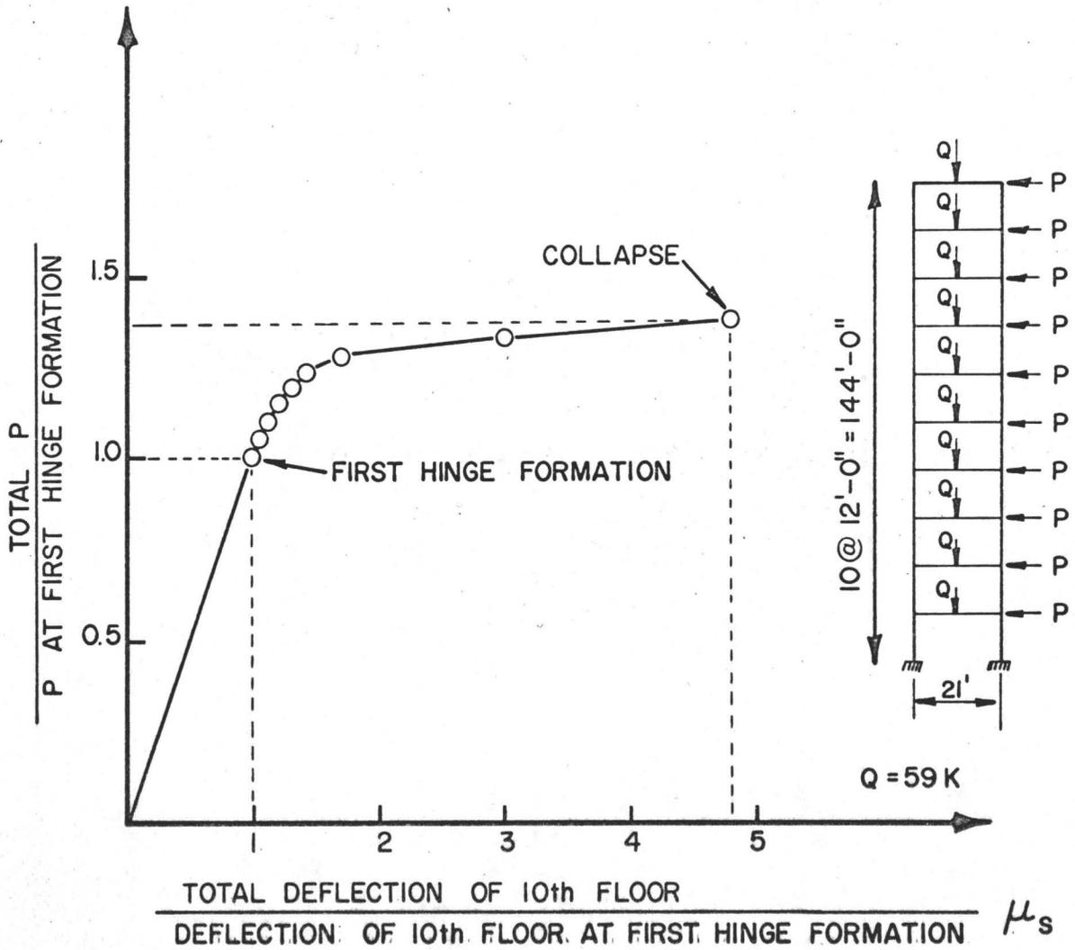
FIG. 3.2 LOAD DEFLECTION CURVE FOR BASIC STRUCTURE.
