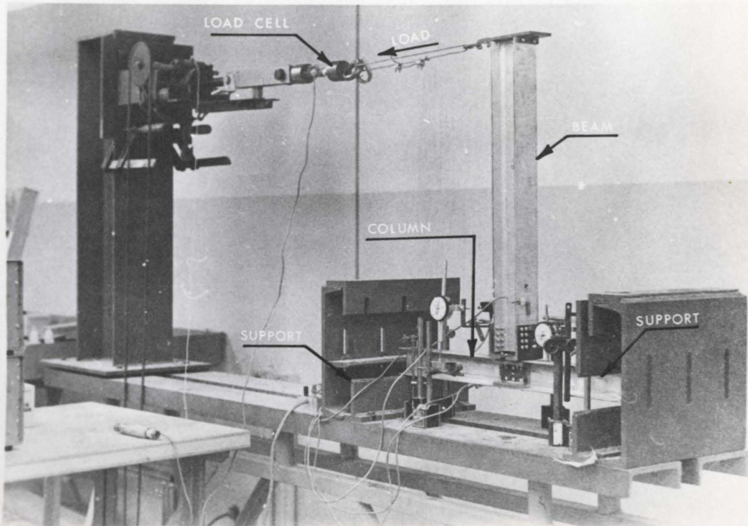
FIG. 6.7 EXPERIMENTAL SET-UP FOR GIRDER-COLUMN JOINT TEST
