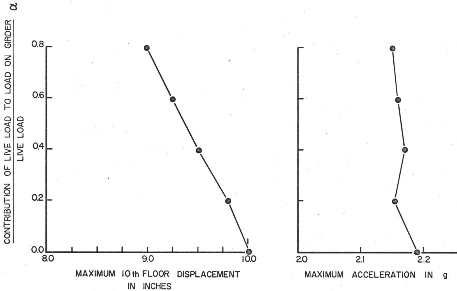
FIG. 4.9 EFFECT OF VARIATION OF LIVE LOAD AS A PURE LOAD ON THE GIRDER.
