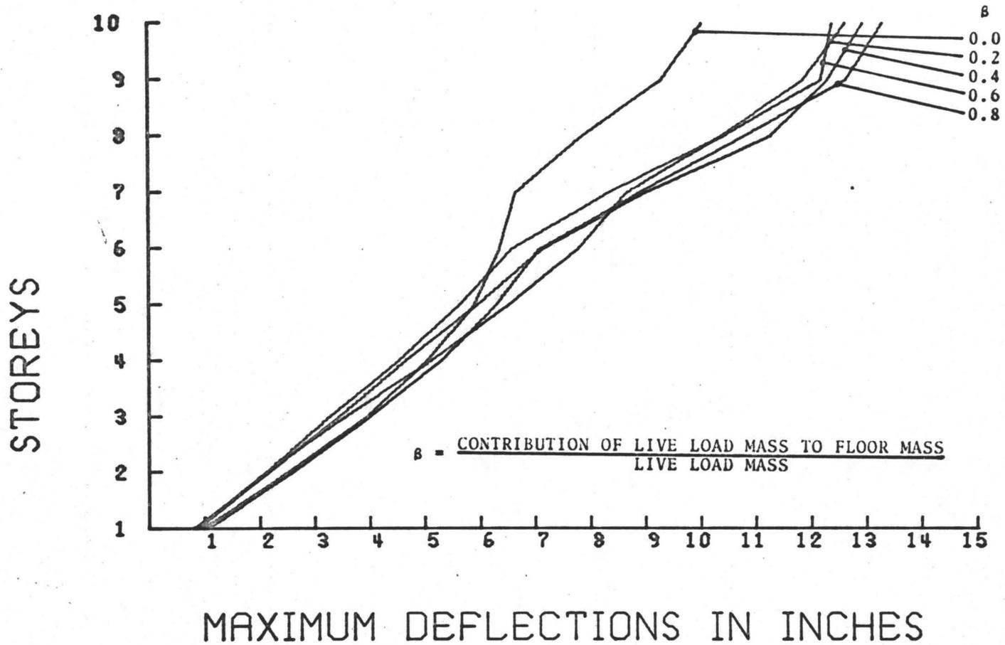
FIG. 4.22 EFFECT OF LIVE LOAD CONTRIBUTION TO FLOOR MASS
