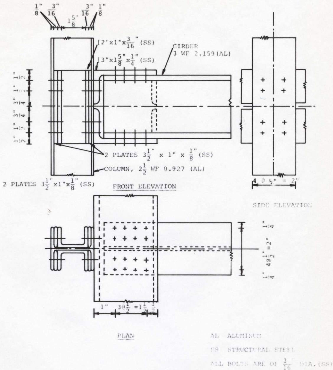
FIG. 6.3 DETAILS OF GIRDER COLUMN JOINT
