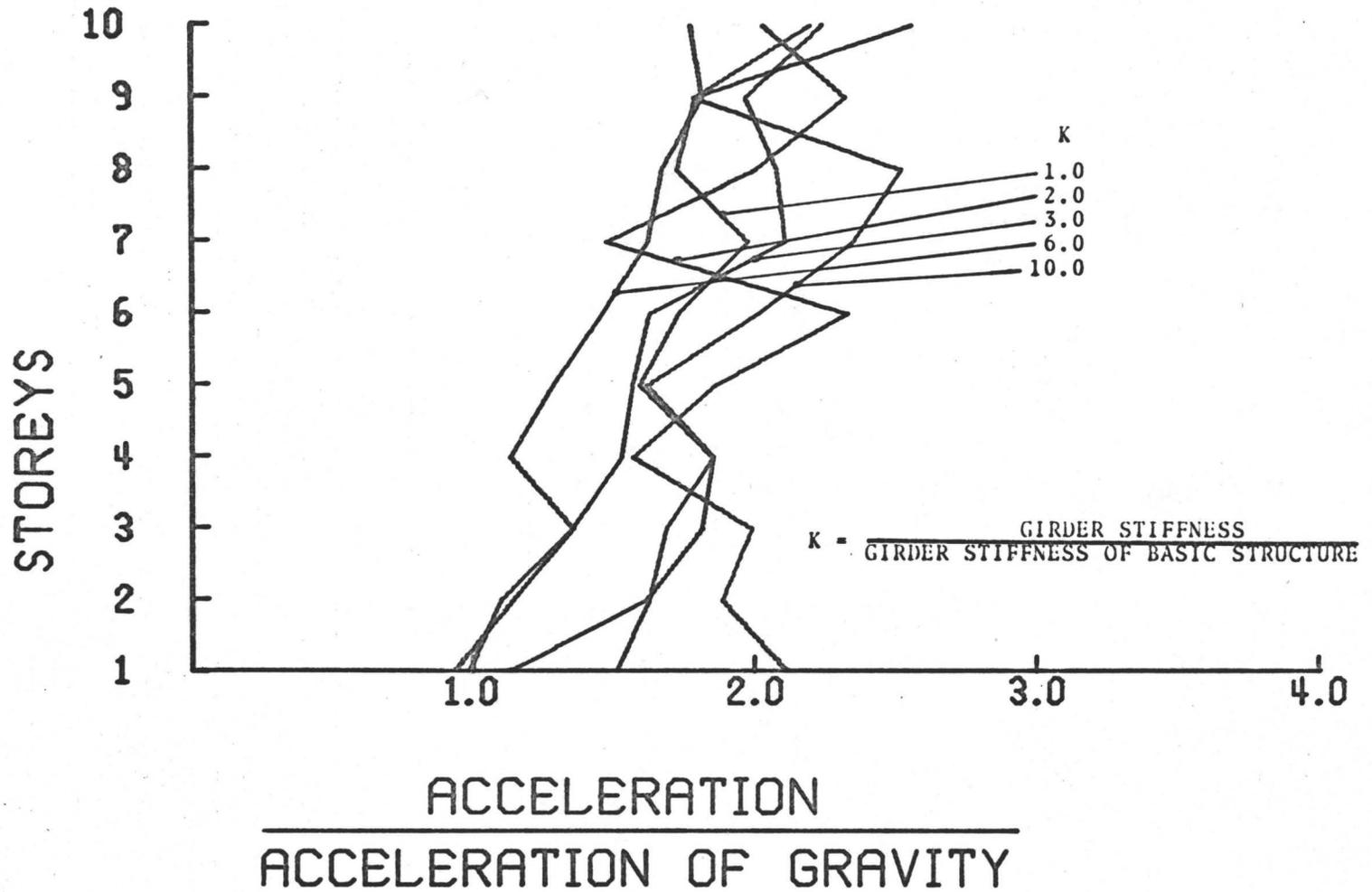
FIG. 4.29 EFFECT OF VARIATION OF RELATIVE STIFFNESS BETWEEN GIRDERS AND COLUMNS
