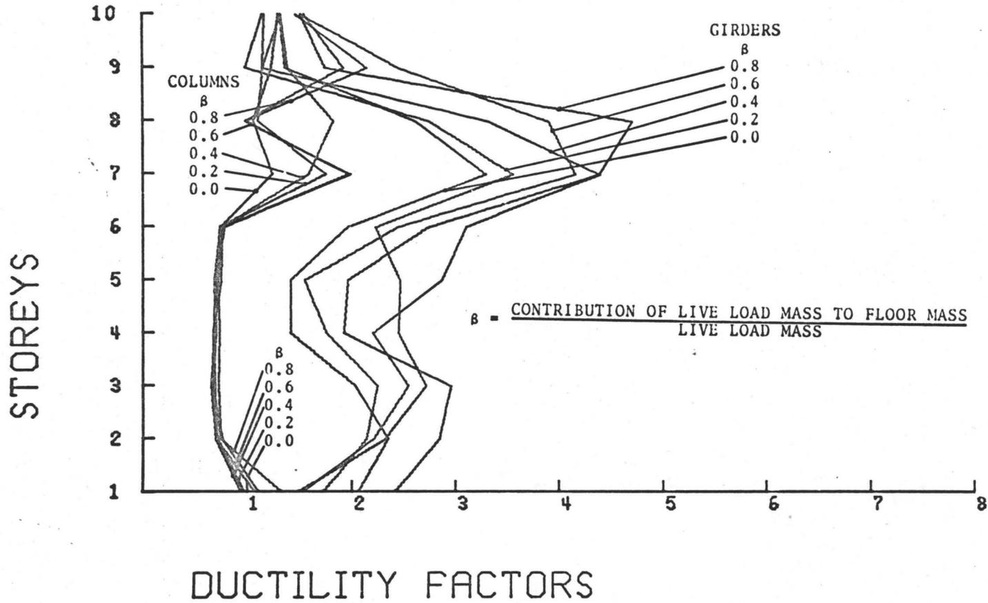
FIG. 4.20 EFFECT OF LIVE LOAD CONTRIBUTION TO FLOOR MASS
