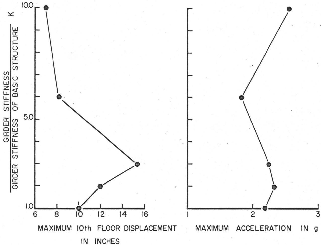
FIG. 4.31 EFFECT OF RELATIVE STIFFNESS BETWEEN GIRDERS AND COLUMNS.
