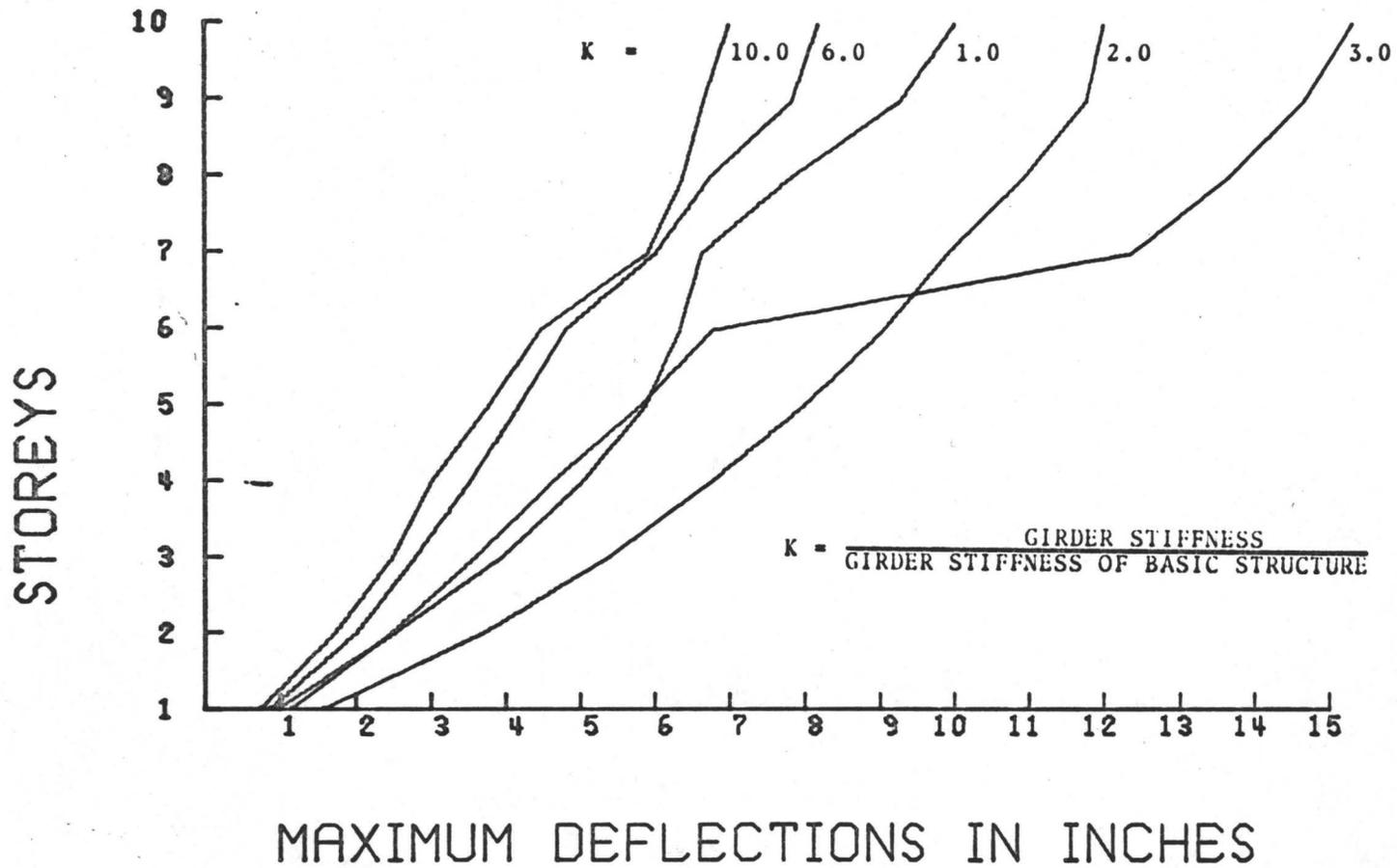
FIG. 4.30 EFFECT OF VARIATION OF RELATIVE STIFFNESS BETWEEN GIRDERS AND COLUMNS
