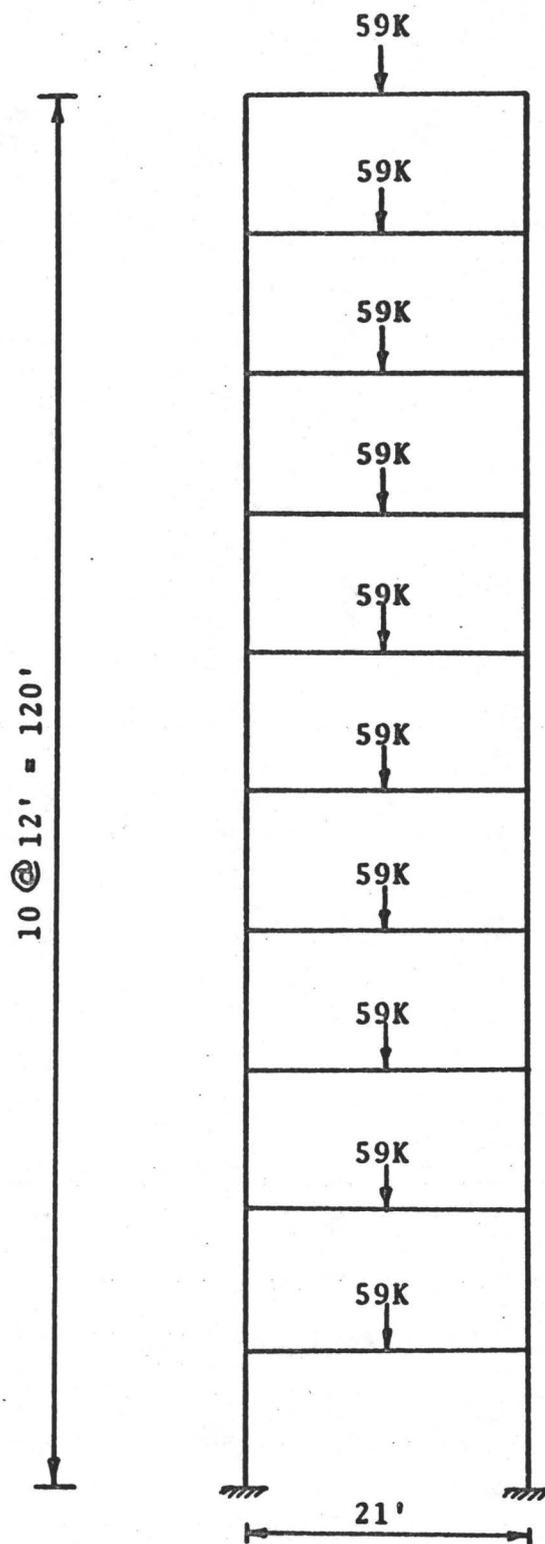
FIG. 3.1 THE BASIC STRUCTURE
