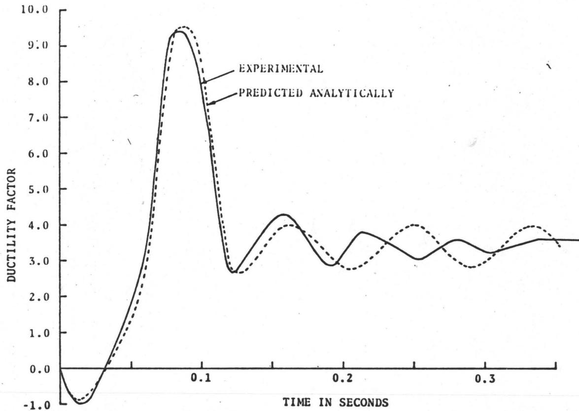
FIG. 8.7 INELASTIC STRAIN RESPONSE OF BOTTOM END OF FIRST STOREY COLUMN
