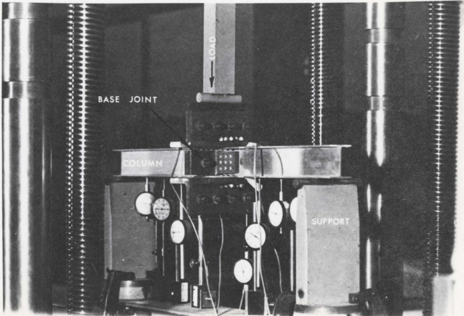
FIG. 6.9 EXPERIMENTAL SET-UP FOR COLUMN BASE JOINT TEST
