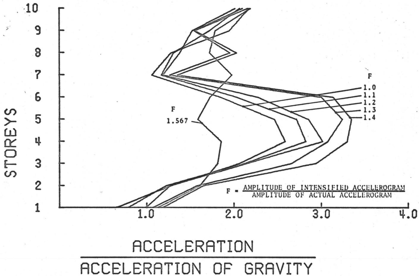
FIG. 4.45 EFFECT OF VARIATION OF EARTHQUAKE INTENSITY
