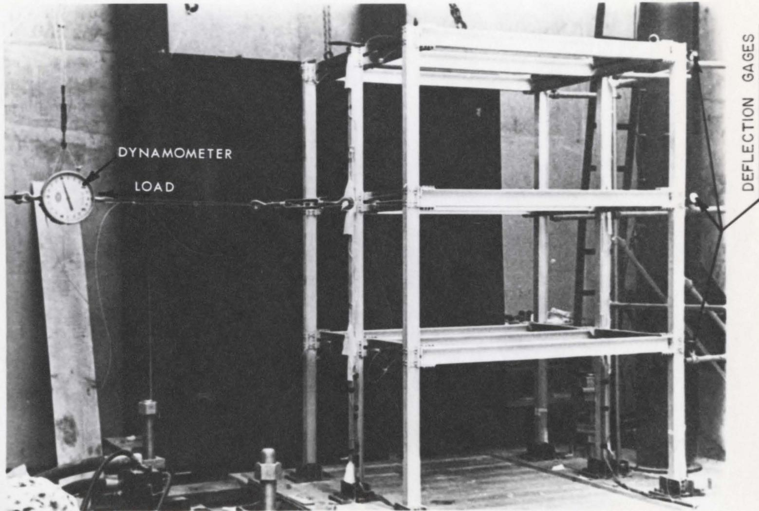
FIG. 6.11 EXPERIMENTAL SET-UP FOR THE DETERMINATION OF FLEXIBILITY
