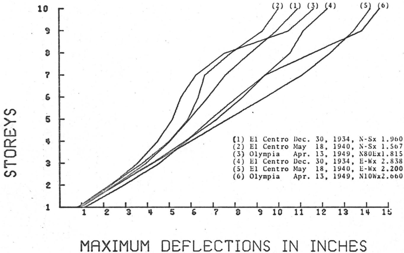
FIG. 4.55 EFFECT OF DIFFERENT EARTHQUAKE CHARACTERISTICS
