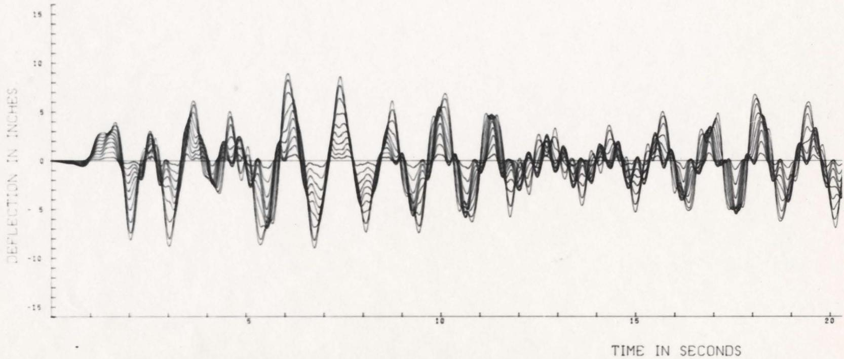
**FIG. 45 INELASTIC RESPONSE HISTORY FOR  $\alpha = 0.8$ ,  $\gamma = 0.0$**
