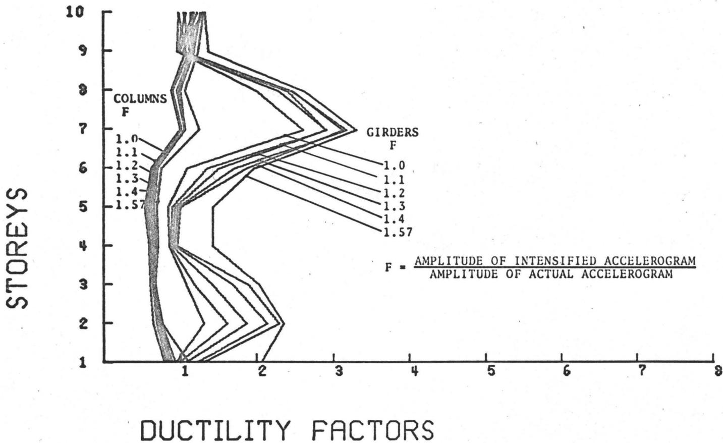
FIG. 4.44 EFFECT OF VARIATION OF EARTHQUAKE INTENSITY
