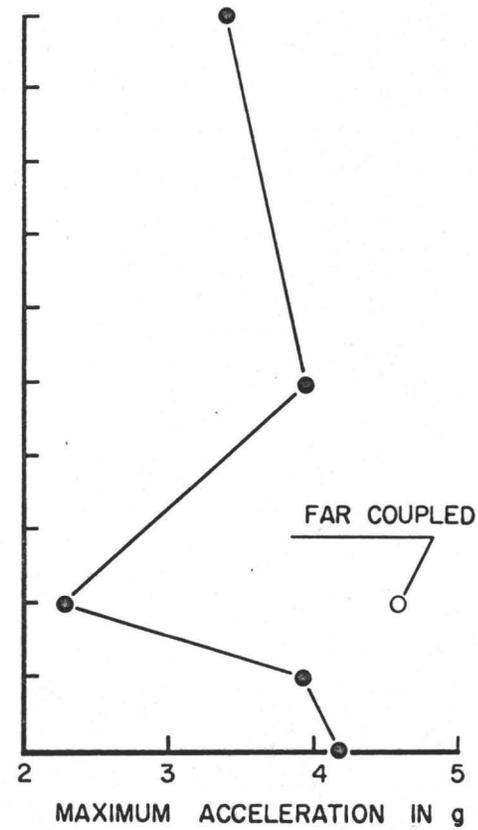
FIG. 4.39 EFFECT OF DAMPING.
