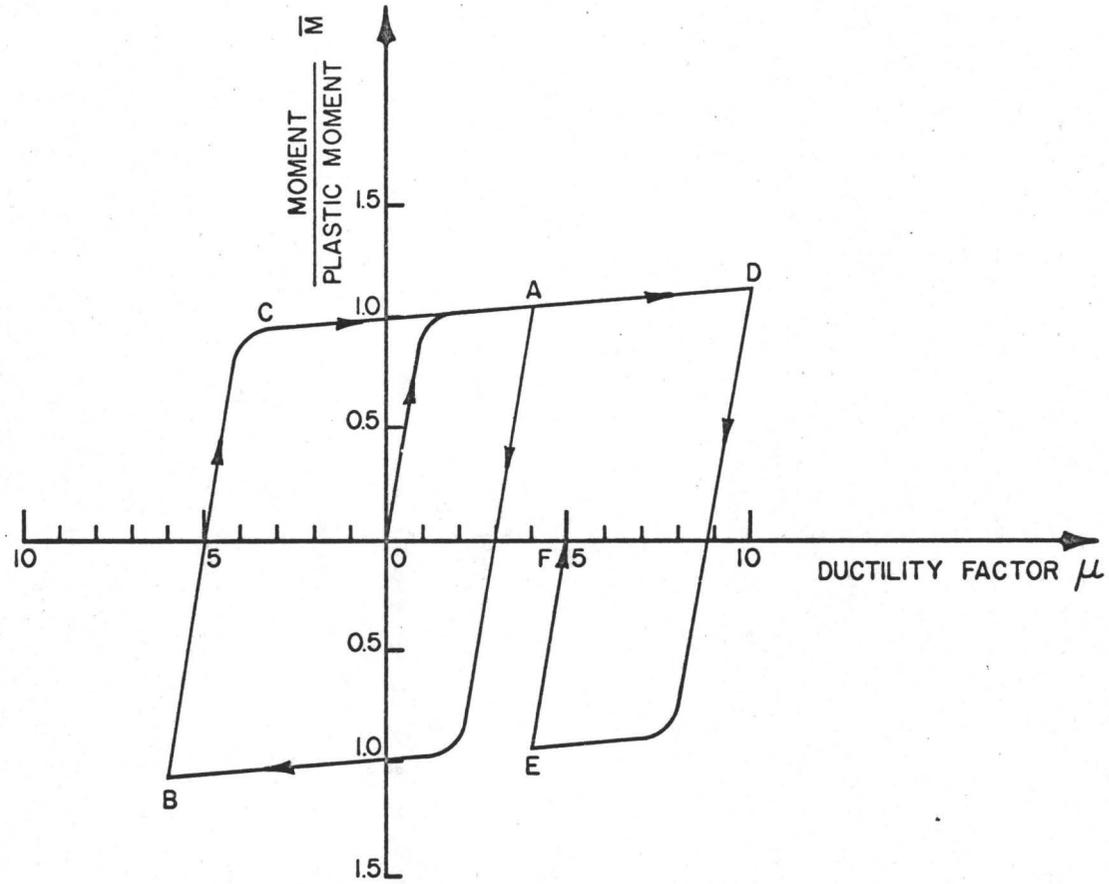
FIG. 6.10 MOMENT CURVATURE RELATIONSHIP OF COLUMNS FROM COLUMN-BASE JOINT TESTS
